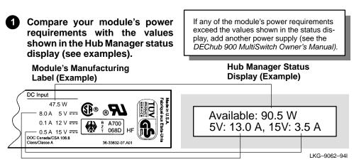
**NOTE:** The 12-volt power in the DEChub 900 is derived from the 15-volt power source. Although it is listed separately in the product specifications, the 12-volt requirements are included in the 15-volt power total.
