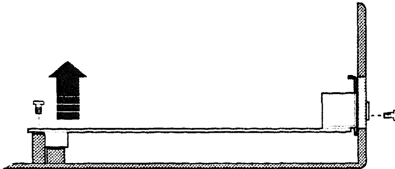
Figure 20 Lifting the Board Away from Support Posts
