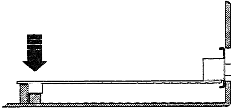
Figure 5 Pushing Module onto Support Posts
