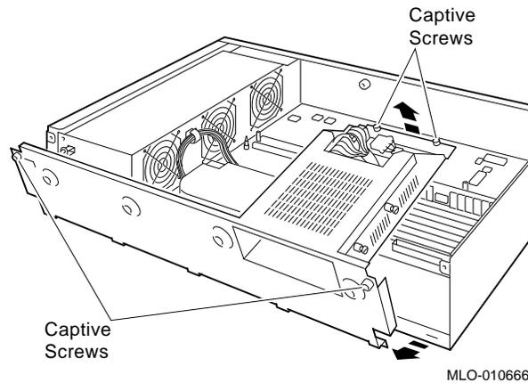
4. Pull up carefully from the back of the drive bracket. As you raise the end of the bracket, you can pull the disconnected ends of the cables through the cutout in the bracket.
