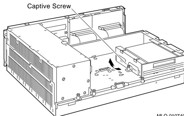
2. Lift the left side of the drive until the tabs on the right side clear the cutouts in the drive shelf.
