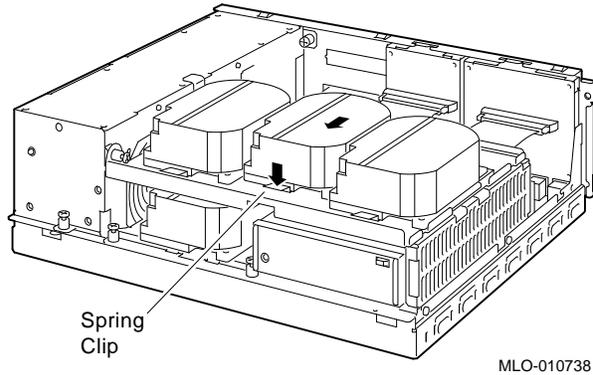
3. Lift the disk drive up from the drive mounting shelf and release the spring clip.
