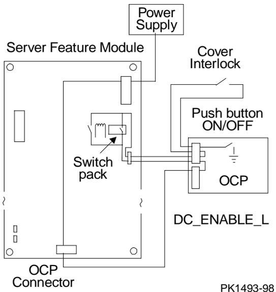
Figure 1-15 shows the distribution of the power enable circuit through the system. Opens in the circuit, or the RCM signal RCM\_DC\_EN\_L, or a power supply detected power fault causes interruption to the DC power applied to the system.
