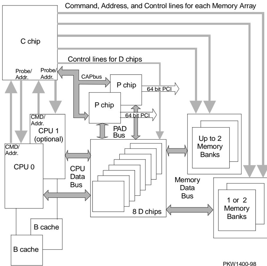
The AlphaServer DS20 is a switch-based interconnect system; it uses a cross-bar switch chipset that allows data to move directly from place to place in the system. The CPU, memory, and I/O devices physically connect to the system board and each has one or two logical connections to the switch. The arrows on the block diagram shown in Figure 1-4 indicate the flow of data, command/address, and control signals.
