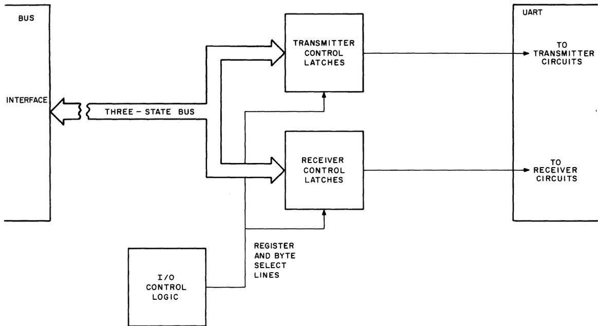
Figure 4-7 Control/Status Register During DATO or DATOB
