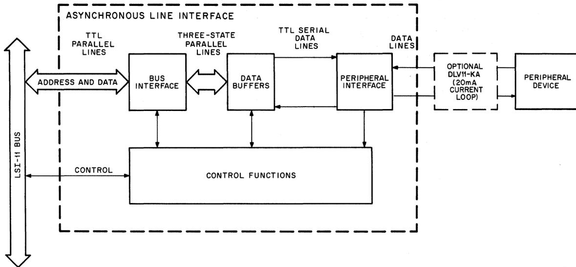
Figure 4-2 DLV11-J Data Flow, Simplified Block Diagram
