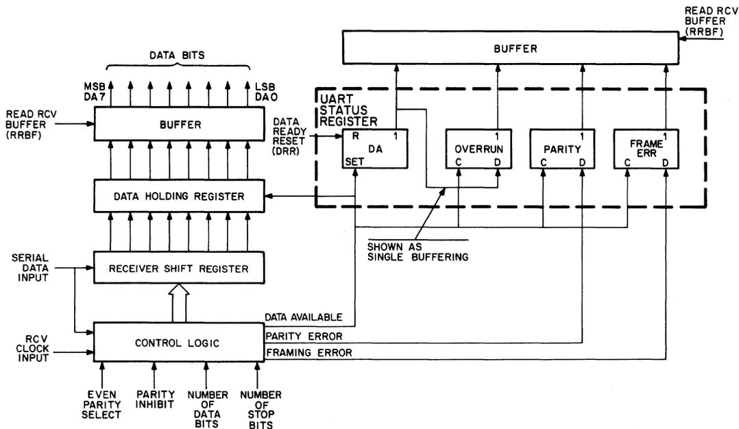
Figure 4-11 UART Receiver Block Diagram
