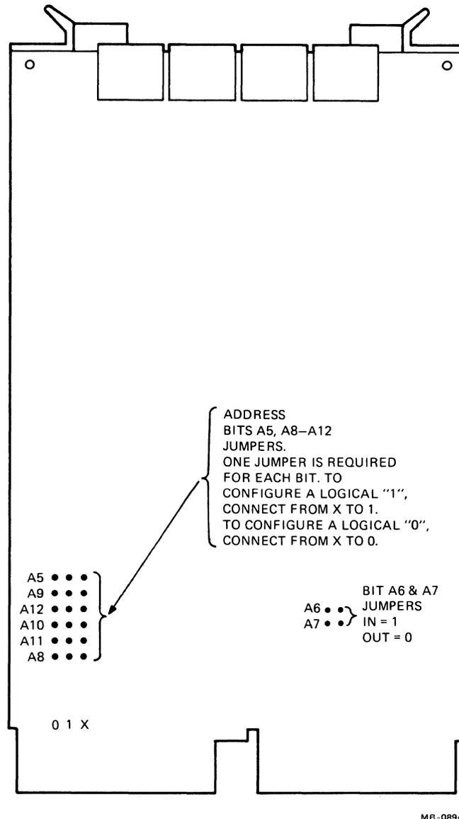
Figure 2-3 Device Register Address Jumper Locations
