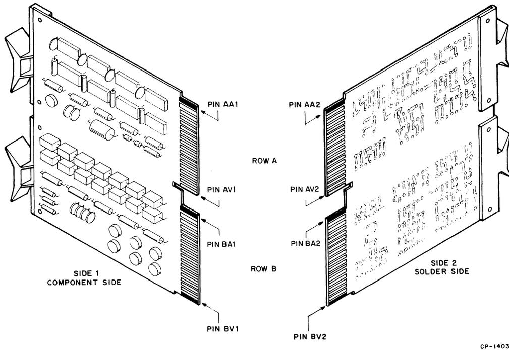
Figure 2-9 Module Contact Finger Identification
