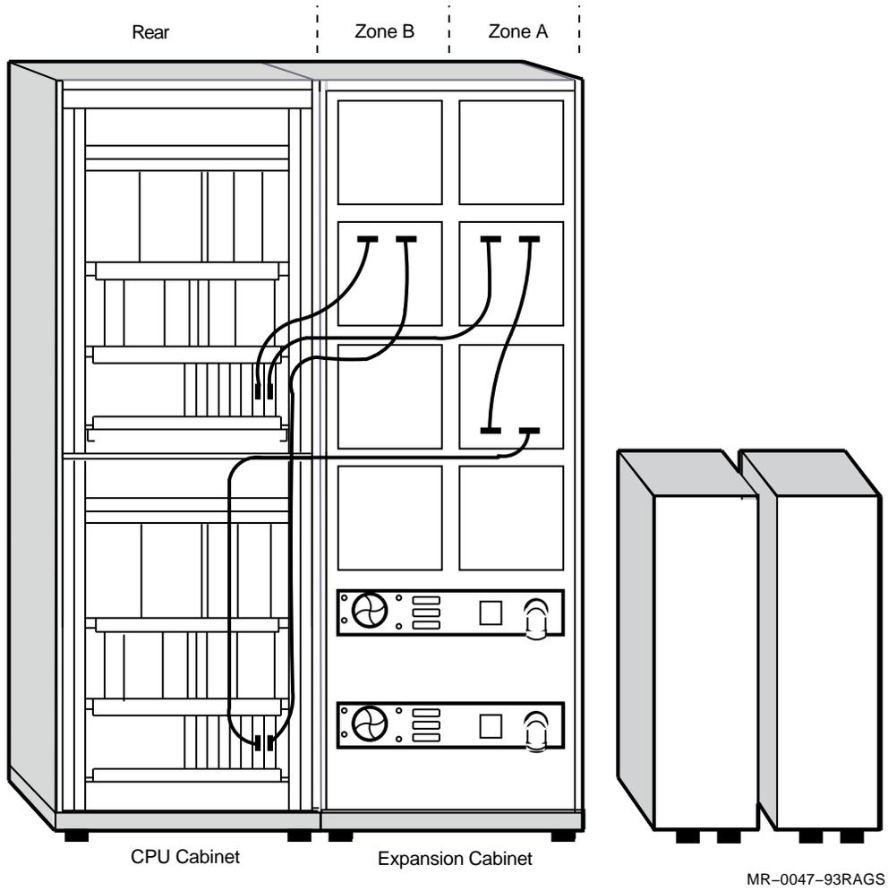
Figure 2-8 Console Module Connectors
