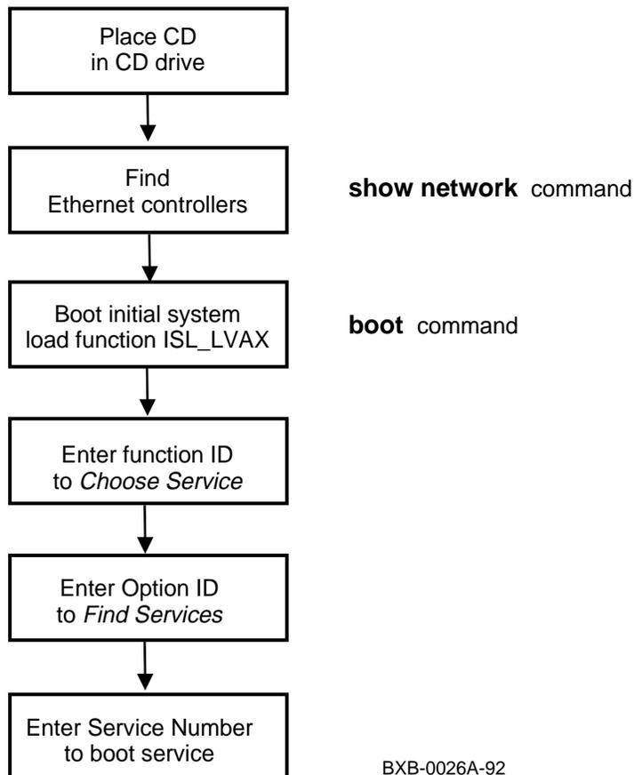
Some systems use Ethernet-based CD servers to load the operating system. The InfoServer consists of one or two CD drives and connects to standard Ethernet or ThinWire groups or networks.
