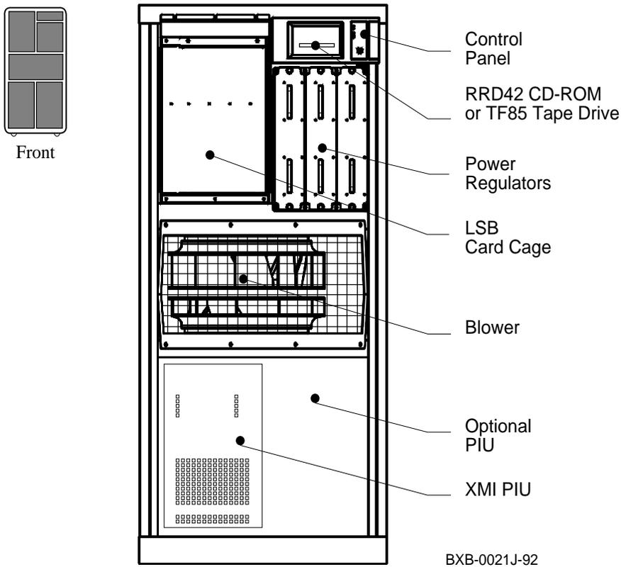
These components are visible from the inside front of the cabinet (see Figure 1-4 for their location):
