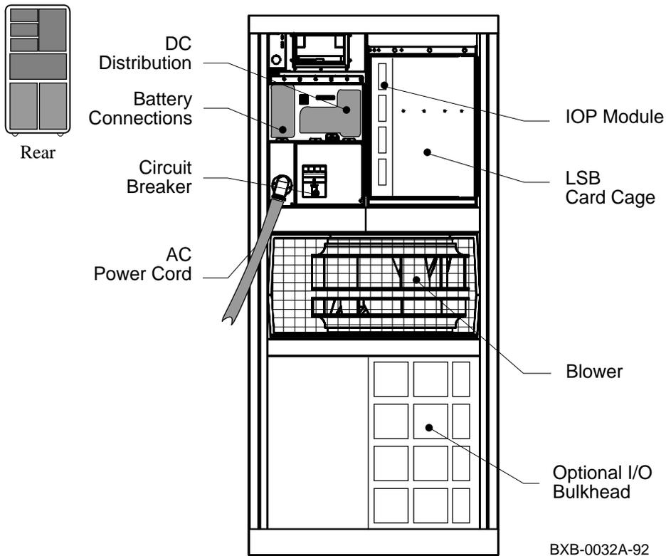
The following components are visible from the rear of the cabinet (see Figure 1-5):
