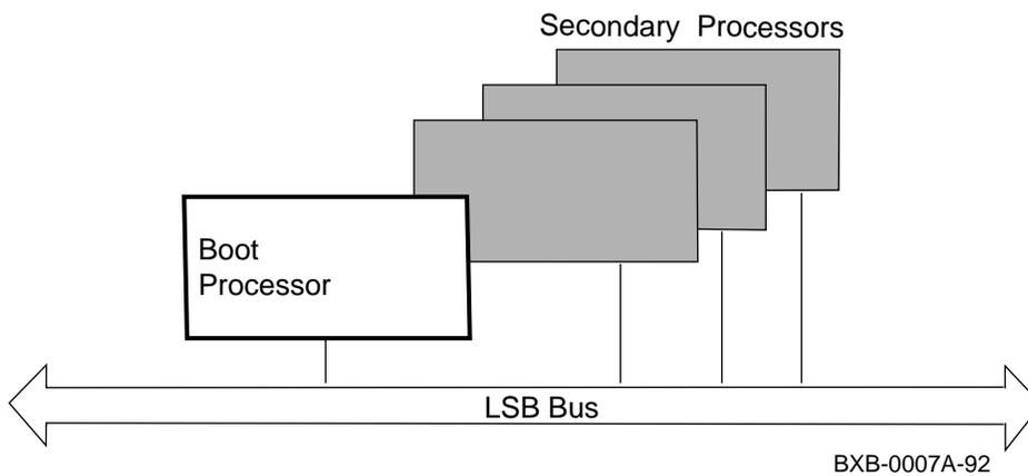
One processor is designated as the boot processor (or primary processor) and becomes the primary communicator to the console terminal.
