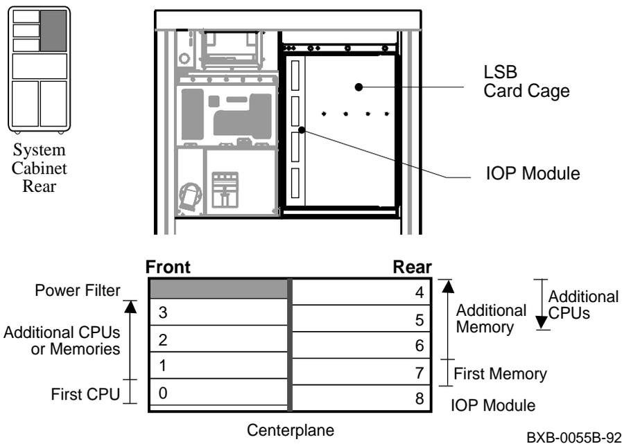
The 9-slot LSB card cage is located in the upper left (front and rear) of the system cabinet, as viewed from the front. The LSB card cage must contain one IOP module, which is always installed in slot 8. The other eight slots contain a combination of memory and CPU modules. Unused slots contain filler modules, which manage the airflow through the cabinet.
