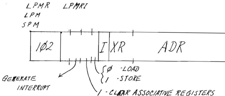
An instruction (OP code 120,000,,) has been added to the PDP-10. This instruction transfers eight words in a block pointed to by the effective address (absolute) to or from the paging device. Load Page Memory (LPM 102,000,,) transfers from memory to the paging device, and Store Page Memory (SPM 102,040,,) writes back in memory the same eight words of state information.
