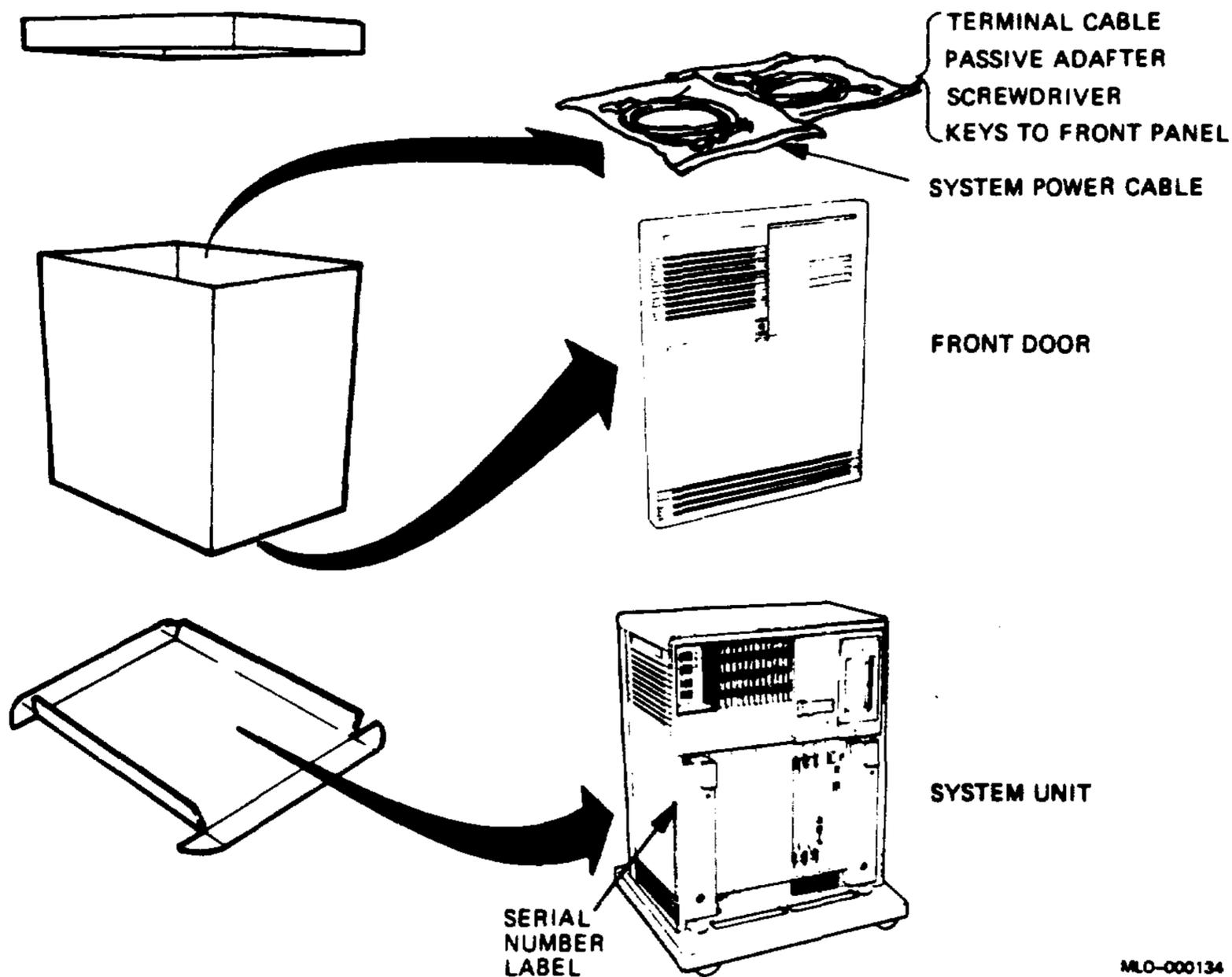
Verify that the system power requirements match the power source. The correct voltage for the system is listed on the serial number label next to the left power supply (Figure 2-2). If the voltage does not match the power source, do not continue. Contact the customer's sales representative.
