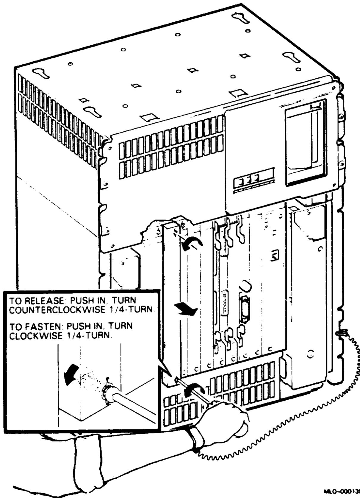
**Figure 3-4: Removing a Module**
