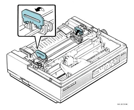
7. Move the paper release lever toward the front of the printer to set the printer in tractor mode.
