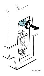
2. Replace the old fuse with a new one of equal value.
