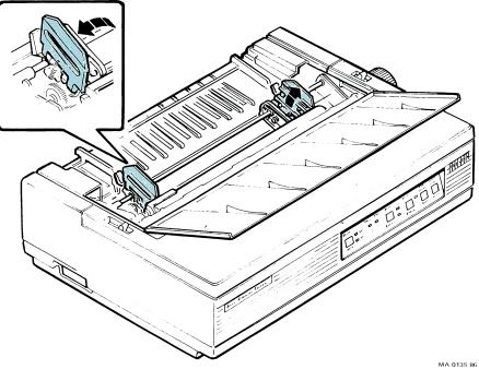
5. Align the pinfeed holes on both edges of the paper with the tractor pins of both tractors. Close the tractor doors to secure the paper.
