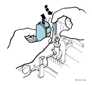
5. Push the head clamp to the right and insert the replacement printhead into the connector on the carriage.
