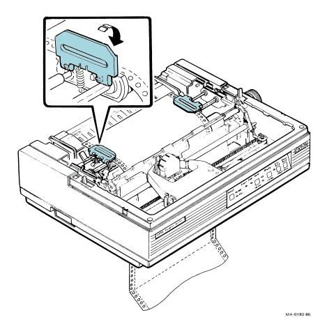
12. Adjust the right tractor by moving it to the right or left so that the paper is stretched taut between the two tractors. Lock both tractors in place by pushing the clamps toward the back of the printer.
