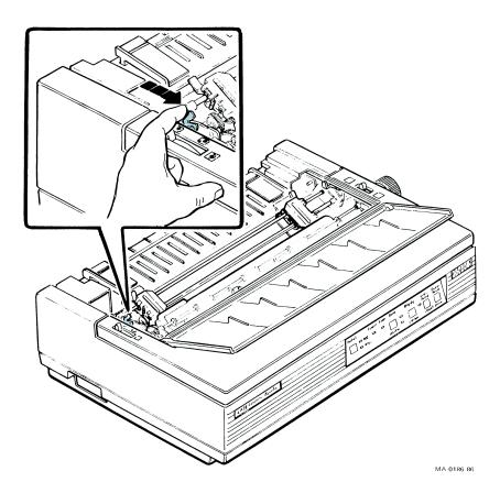
4. Move the right tractor release lever toward the front of the printer while pushing the tractor unit down. The tractors are now in the push position.
