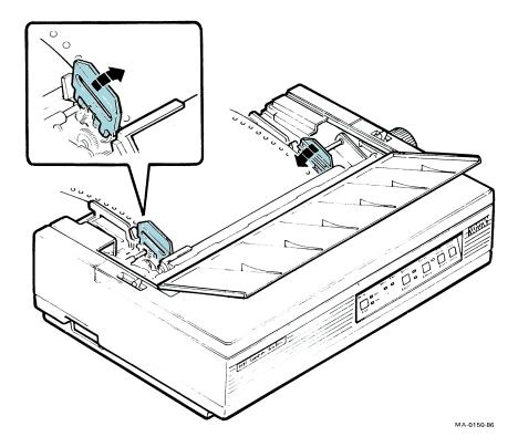
8. Adjust the right tractor by moving it to the right or left so that the paper is stretched taut between the two tractors. Lock the right tractor clamp by pushing the clamp toward the back of the printer.
