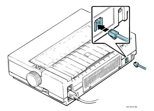
3. Plug the other end of the interface cable directly into your host computer. If you use an adapter, first plug the interface cable into the appropriate adapter and then to your host computer or video terminal (with printer port).
