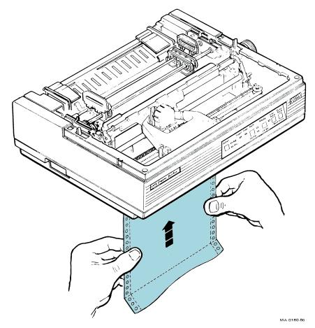
10. Pull the paper up between the platen and the smudge guard and bring it back to the tractors.
