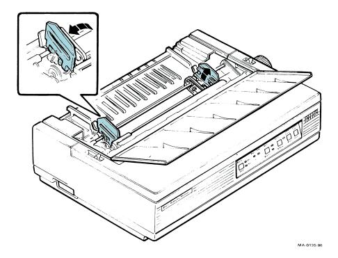
7. Align the pinfeed holes on both edges of the paper with the tractor pins of both tractors. Close the tractor door to secure the paper.
