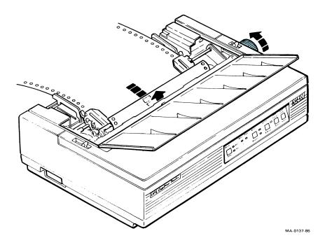
10. Push the bail bar lever toward the back of the printer to set the bail bar against the paper and the platen.
