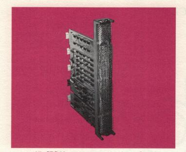
All PDP-11 processors, memories and peripherals are electrically and mechanically modular subsystems supported in System Units which are simply plugged together to form a computer tailored to user needs.
