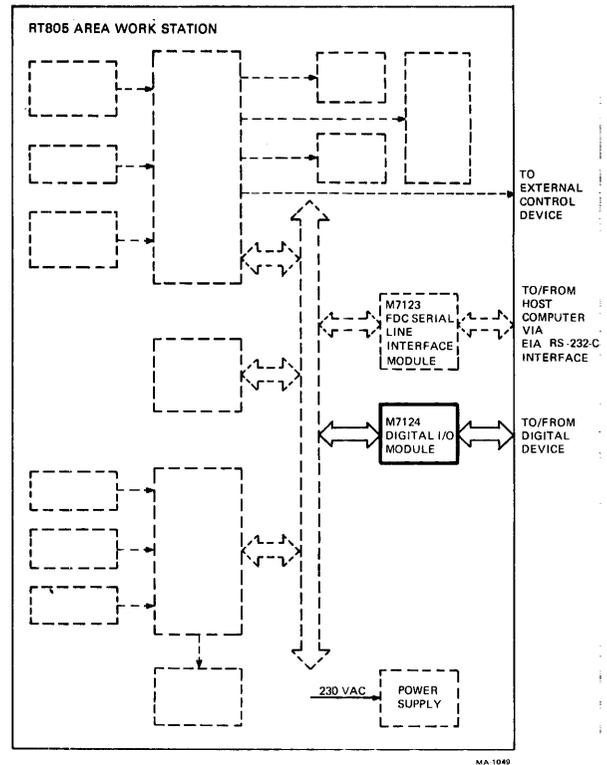
Figure 1-27 RT805-BA/BB (EIA RS-232-C) with XD (I/O) Option – Block Diagram
