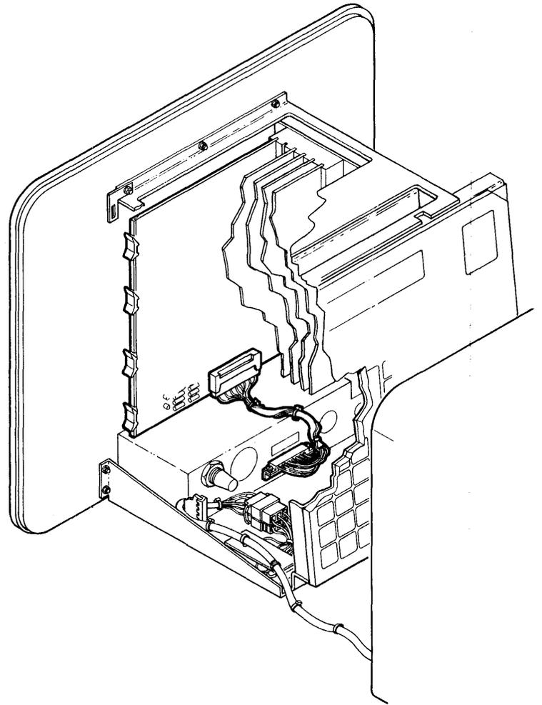
Figure 2-9 RT805-XC (20 mA Current Loop) Option Location
