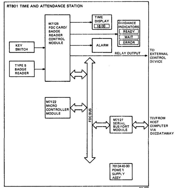
Figure 1-14 RT801-AA/AB with DECdataway Interface – Block Diagram
