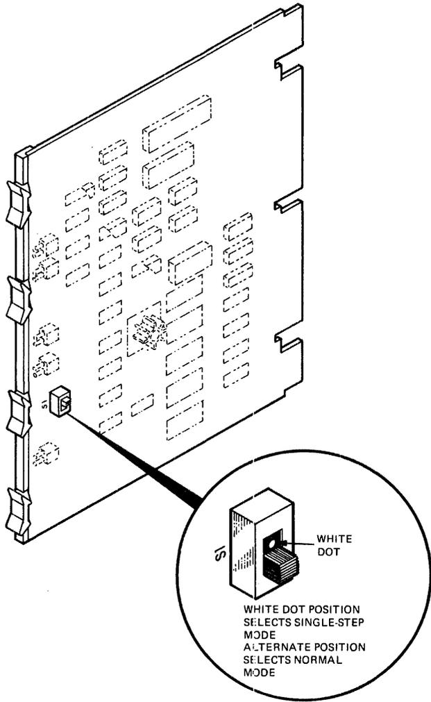
Figure 4-1 M7122 Normal/Single-Step Switch
