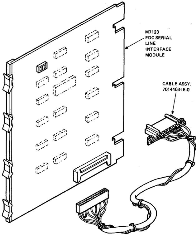
Figure 2-8 RT805-XC (20 mA Current Loop) Option Kit
