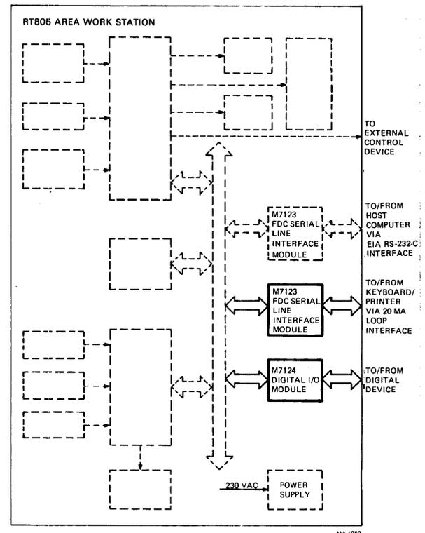
Figure 1-28 RT805-BA/BB (EIA RS-232-C) with XC (20 mA), XD (I/O) Options – Block Diagram
