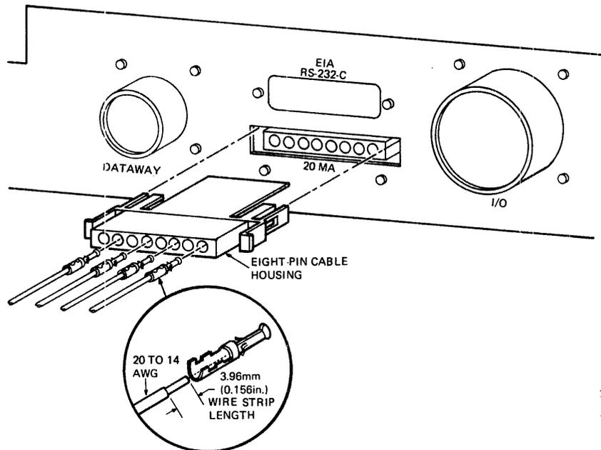
Figure 2-15 20 mA Cable Assembly Details
