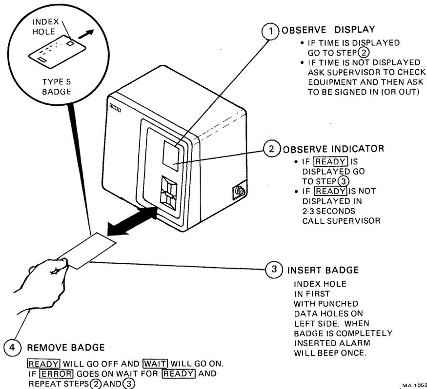
Figure 3-5 Typical RT801 Operating Procedure
