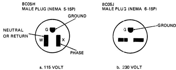
Figure 1-12 Power Plug Configurations
