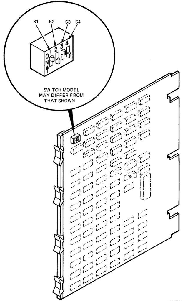
Figure 4-2 M7125 Terminal Identification Switch Pack
