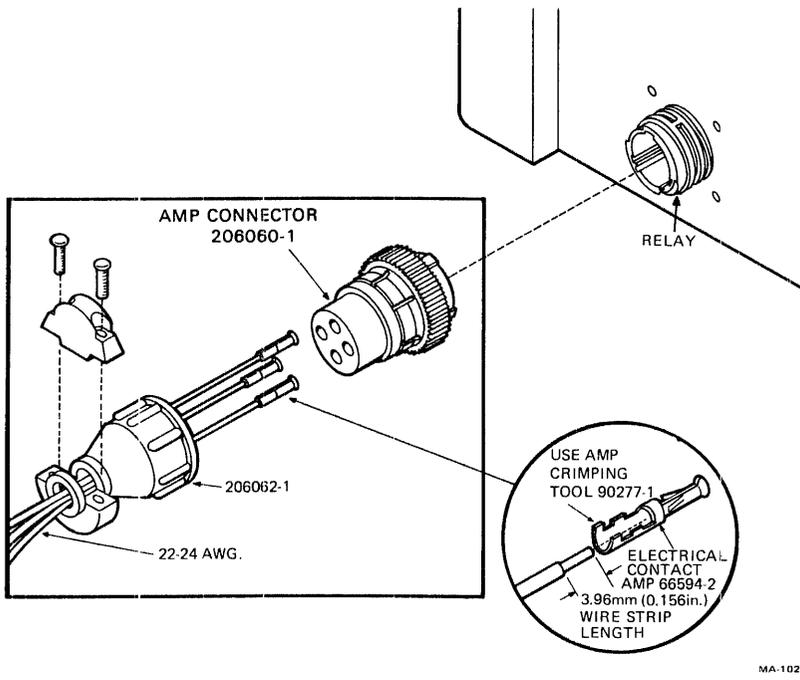
Figure 2-4 External Control Circuit Connector Details
