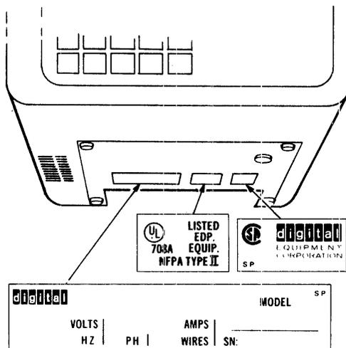
Figure 1-13 Electrical Data Plates
