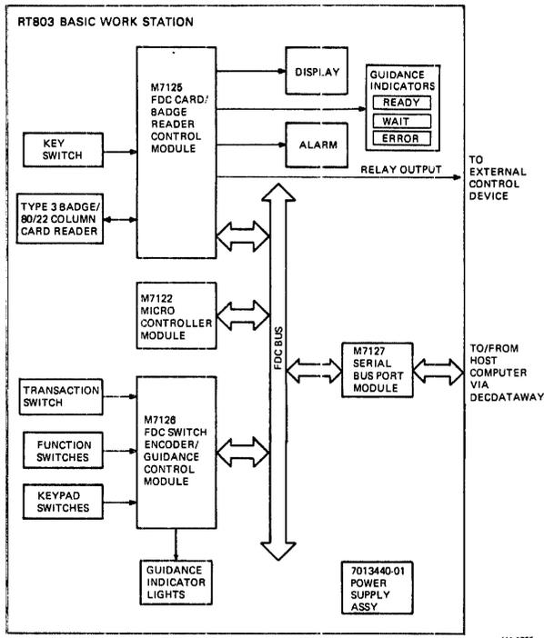
Figure 1-17 RT803-AA/AB (DECdataway) – Block Diagram
