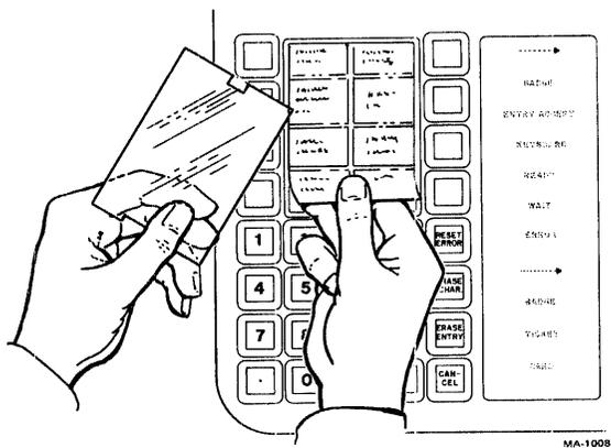
Figure 1-11 RT805 Transaction Switches Instruction Insert
