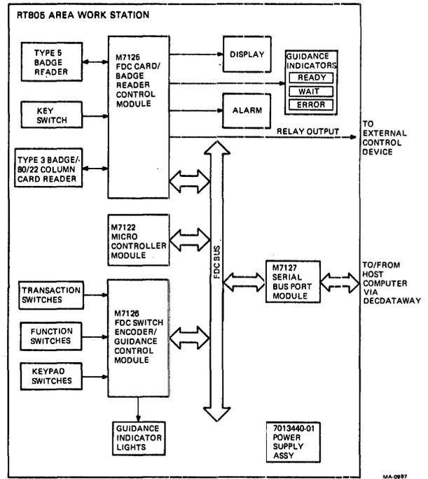
Figure 1-20 RT805-AA/AB (DECdataway) – Block Diagram
