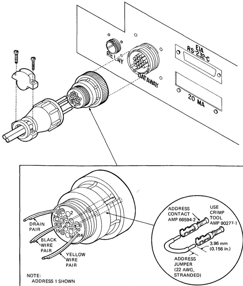
Figure 2-5 DECdataway Connector Addressing Details
