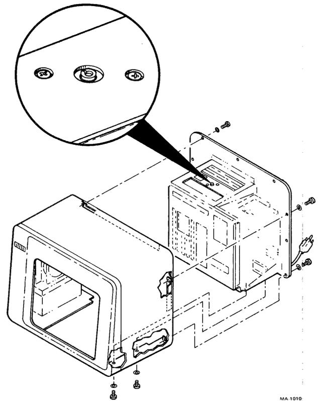
Figure 4-4 Terminal Over Temperature Switch
