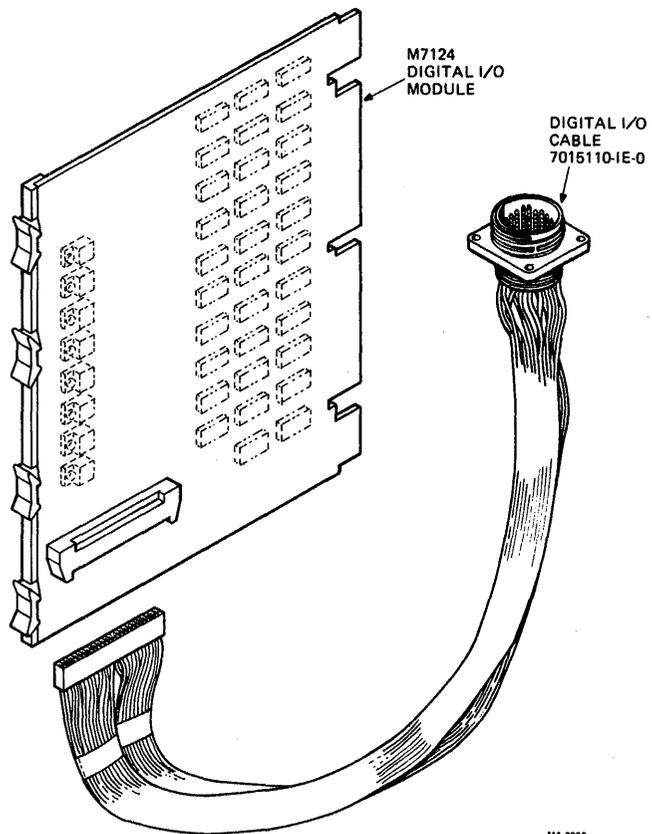
Figure 2-16 RT805-XD (Digital I/O) Option Kit
