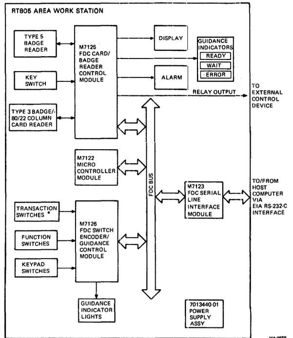
Figure 1-21 RT805-BA/BB (EIA RS-232-C) – Block Diagram
