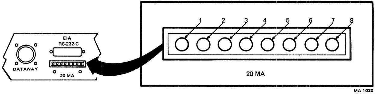
Figure 2-14 20 mA Connector Pin Designations
