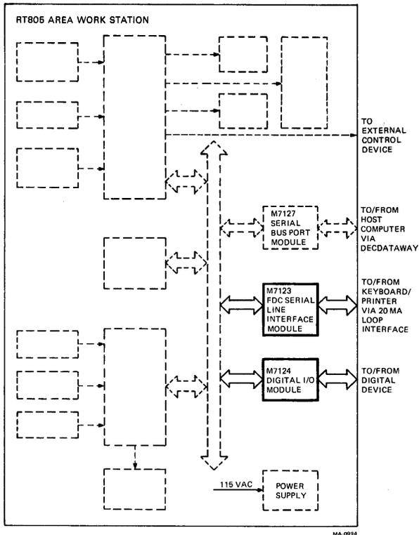
Figure 1-25 RT805-AA/AB (DECdataway) with XC (20 mA), XD (I/O) Options – Block Diagram
