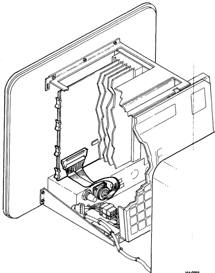
Figure 2-17 RT805-XD (Digital I/O) Option Location
