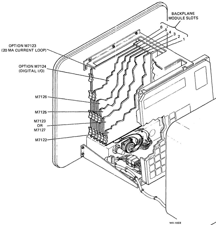
Figure 2-10 RT805 Option Modules Backplane Slot Assignments
