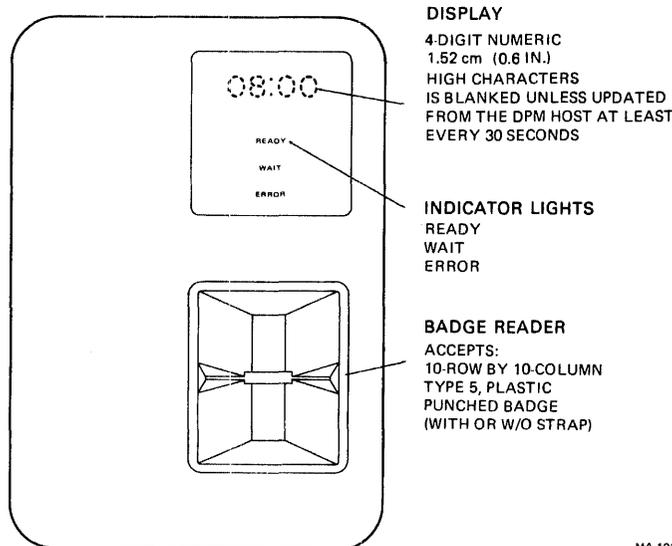
Figure 1-7 RT801 Operator's Panel
