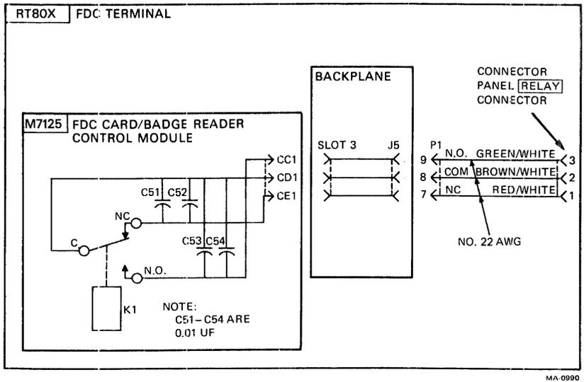
Figure 2-3 External Control Circuit - Schematic Diagram
