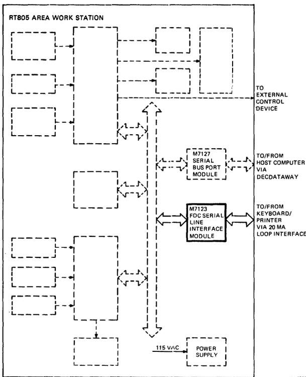
Figure 1-23 RT805-AA/AB (DECdataway) with XC (20 mA) Option — Block Diagram
