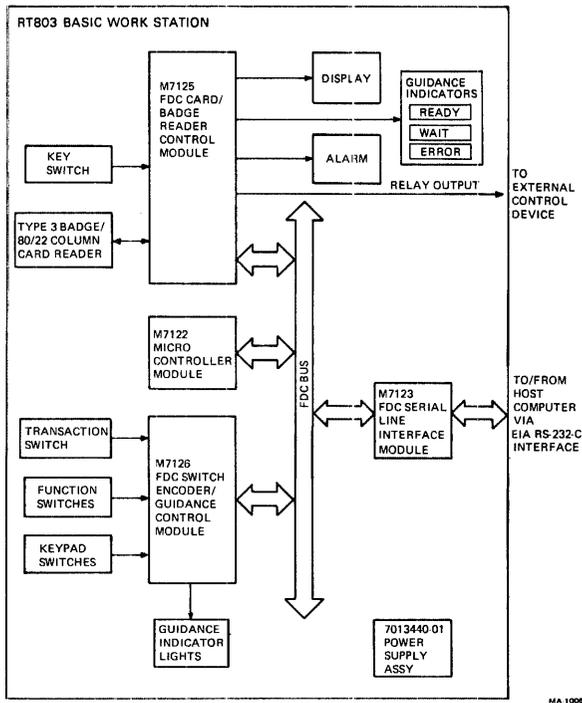
Figure 1-18 RT803-BA/BB (EIA RS-232-C) – Block Diagram
