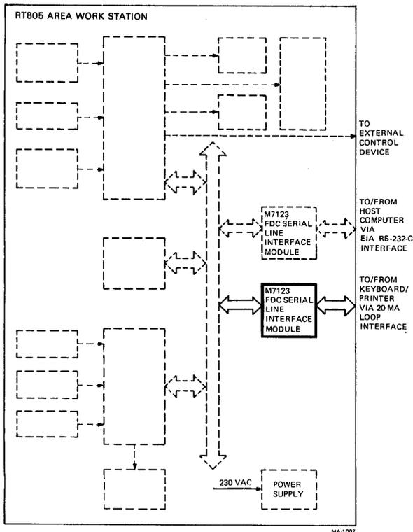
Figure 1-26 RT805-BA/BB (EIA RS-232-C) with XC (20 mA) Option – Block Diagram
