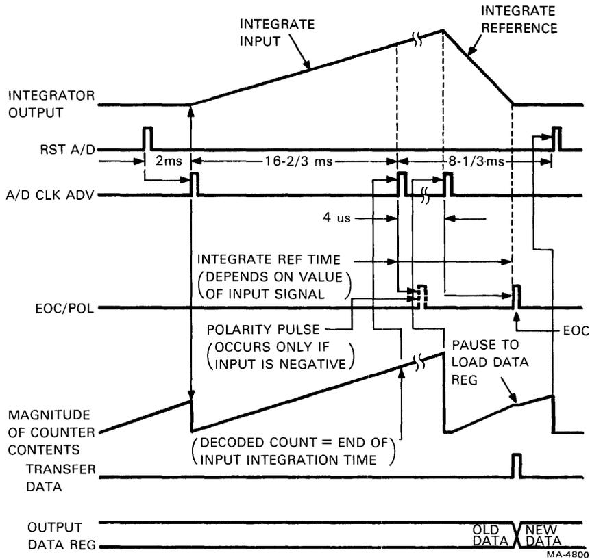
Figure 6-21-7 Conversion Cycle Timing (60 Hz Timing Shown)
