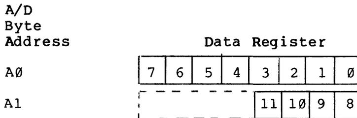
The eight LSBs, D(0-7), are in byte A0 and the four MSBs, D(8-11), are in the first four bit positions of byte A1.
