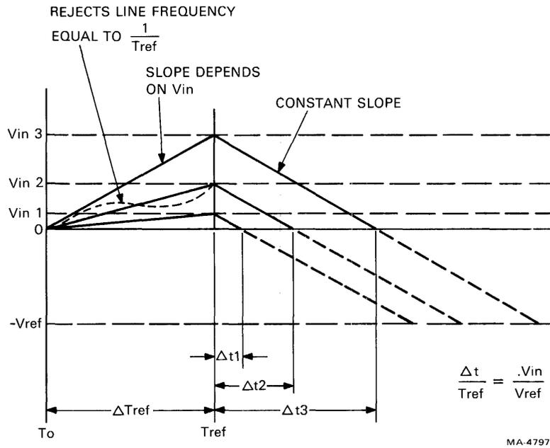
Figure 6-21-4 Dual Slope Converter Time Voltage Relationships
