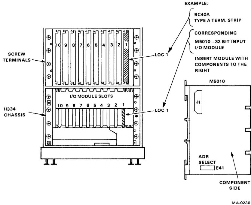
Figure 3-11 Module and Screw Terminal Configurations
