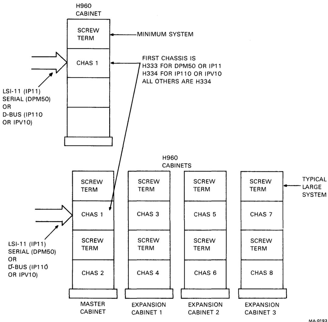
Figure 2-2 UNIBUS or Serial Bus Based Configurations
