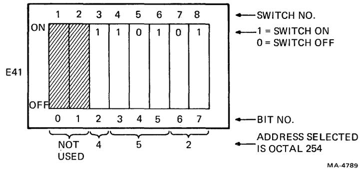
Figure 6-9-3 Address Selection Switch
