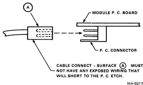
Figure 3-32 I/O Cable Connector Interface
