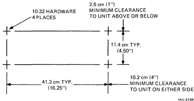
Figure 6-22-6 Rear Mounting Dimensions
