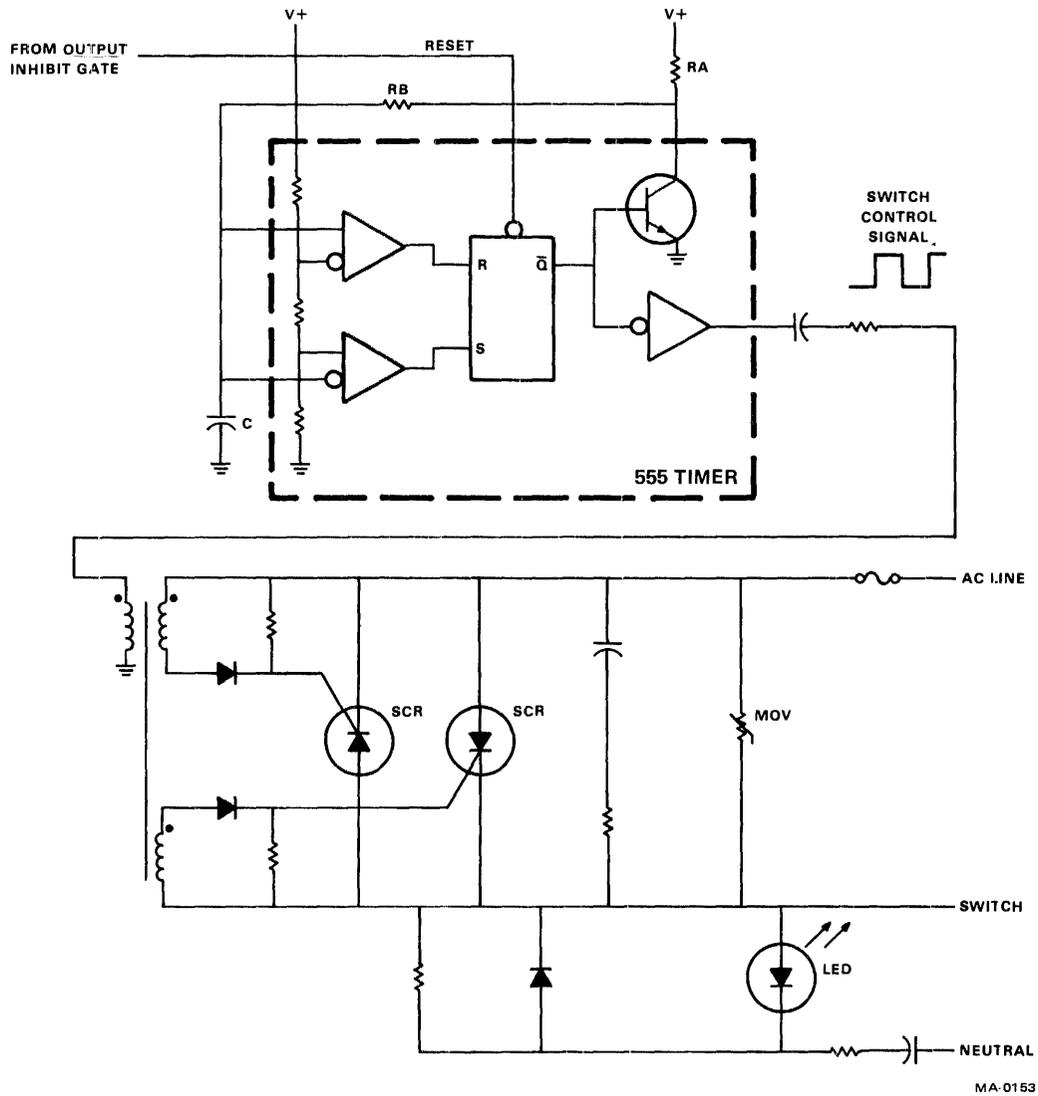
Figure 6-14-2 Output Switch and Control Oscillator
