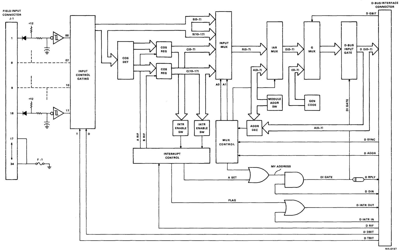
Figure 6-3-1 16-Bit COS Input Module M5011,
