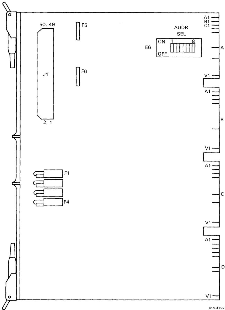
Figure 6-16-3 M6015 16-Bit Retentive DC Output
