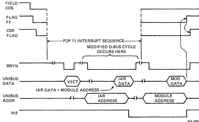
Figure 5-20 I/O Subsystem PDP-11 Based Interrupt Timing
