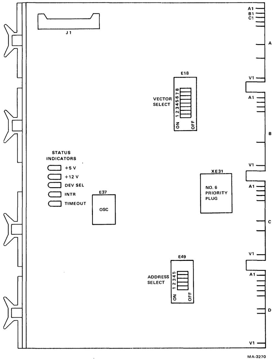
Figure 3-23 M8719 UNIBUS I/O Control Module
