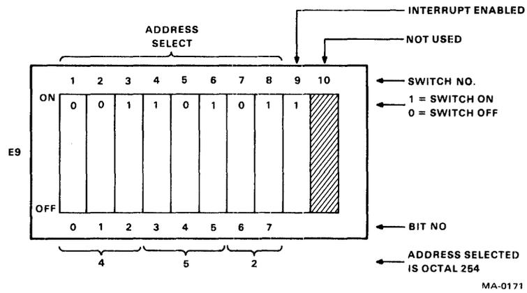
Figure 6-6-3 Address Selection and Interrupt Enable
