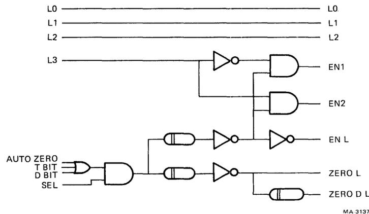
Figure 6-20-2 Channel Select and Auto-Zero Control
