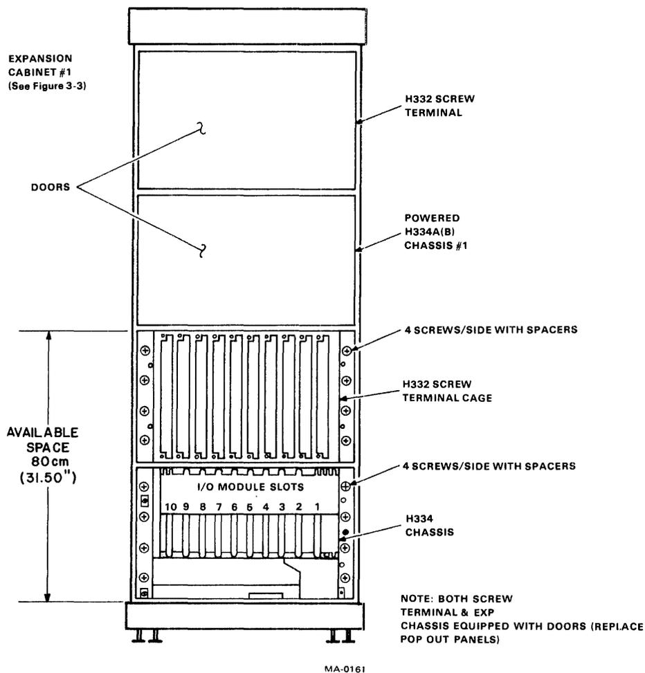
Figure 3-8 Example of I/O Expansion
