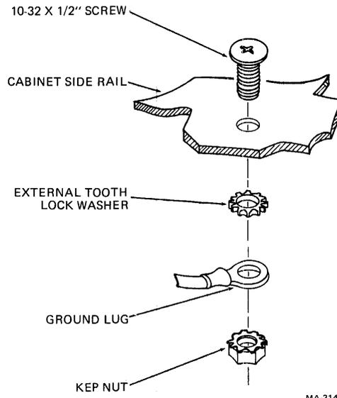
Figure 3-10 Ground Wire Fastening
