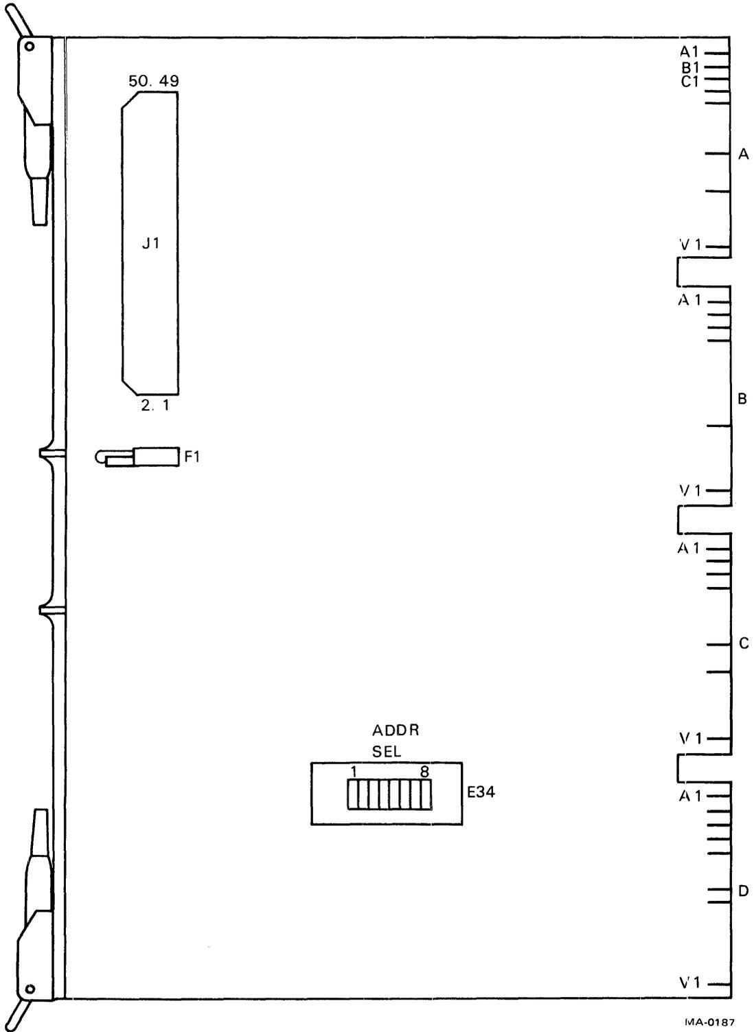
Figure 6-10-2 M6010 32-Bit DC Output
