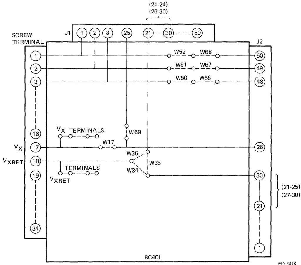
Figure 6-25-4 BC40L Simplified Schematic
