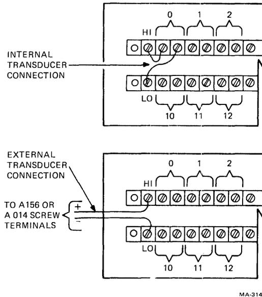
**Figure 6-22-9 Transducer Output Connection Options**
