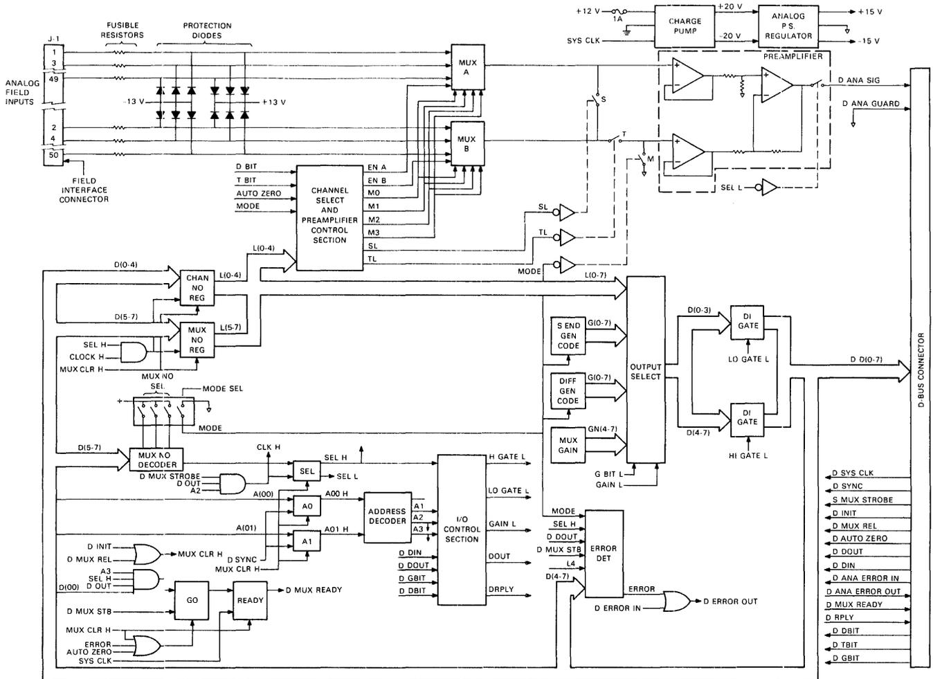
Figure 6-19-1 A156 Analog Multiplexer, Block Diagram
