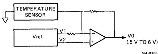
Figure 6-22-4 Temperature Transducer Circuit
