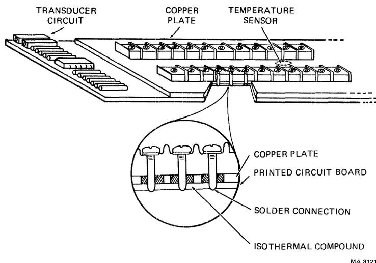
Figure 6-22-3 Isothermal Assembly
