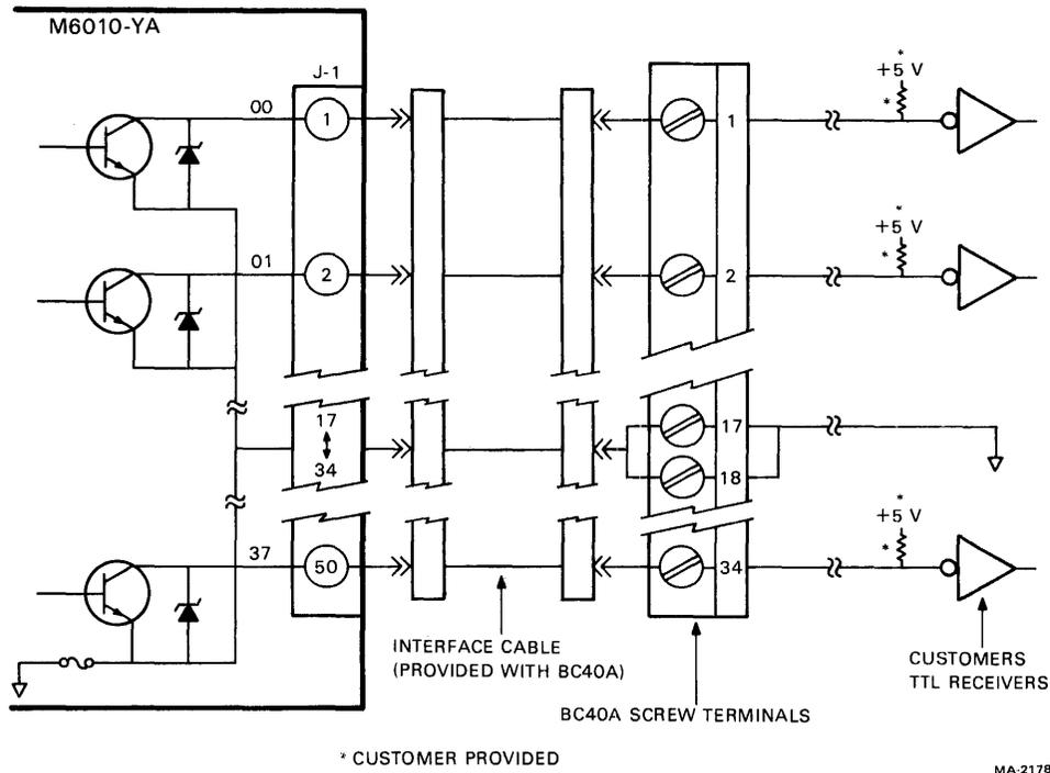
Figure 6-11-4 M6010-YA Typical TTL Field Interface
