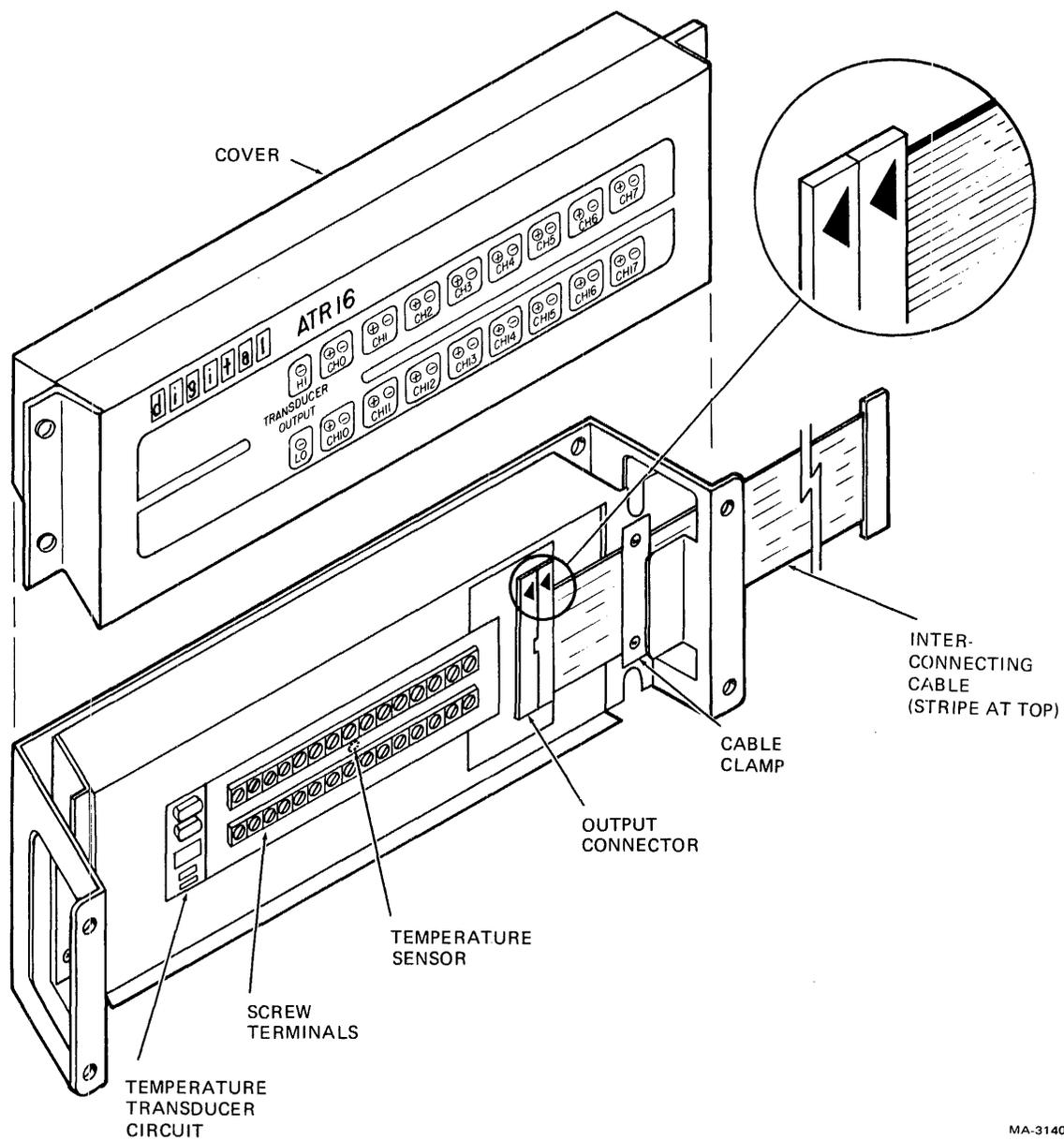
Figure 6-22-1 ATR16 Chassis Assembly
