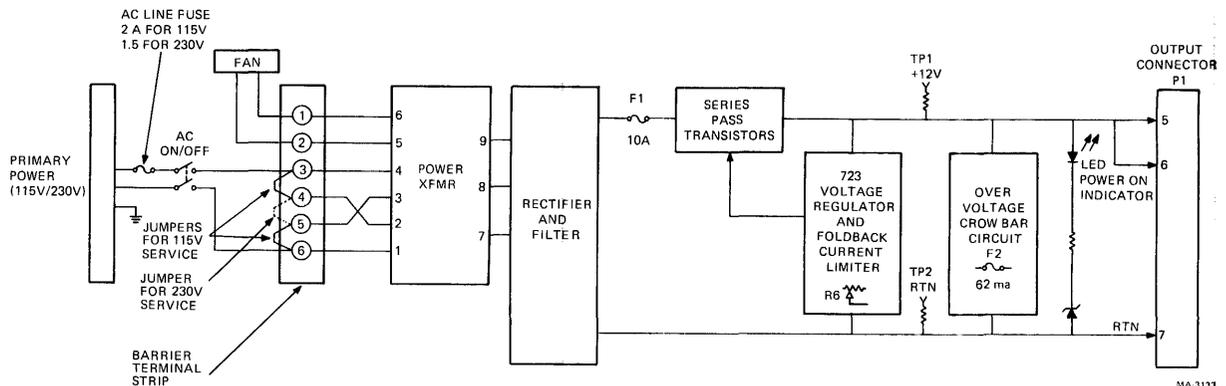
Figure 5-24 H7872 Power Supply Block Diagram
