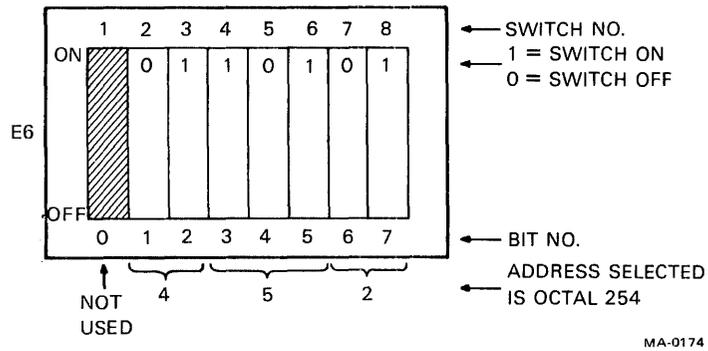
Figure 6-16-4 Address Selection Switch
