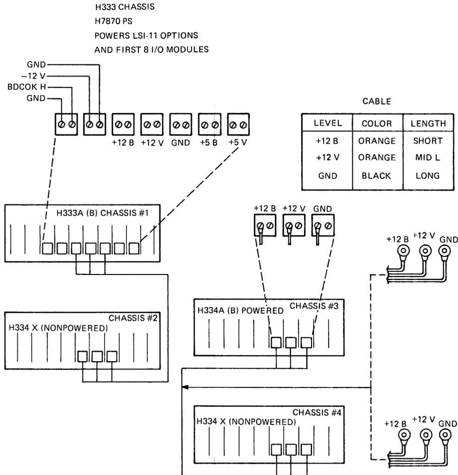
1. EACH NONPOWERED H334 IS PROVIDED WITH A 6 FT POWER INTERCONNECT CABLE.
