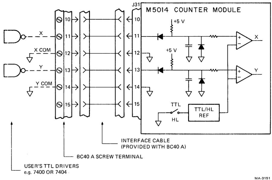
Figure 6-7-13 M5014 Nonisolated TTL Input Application
