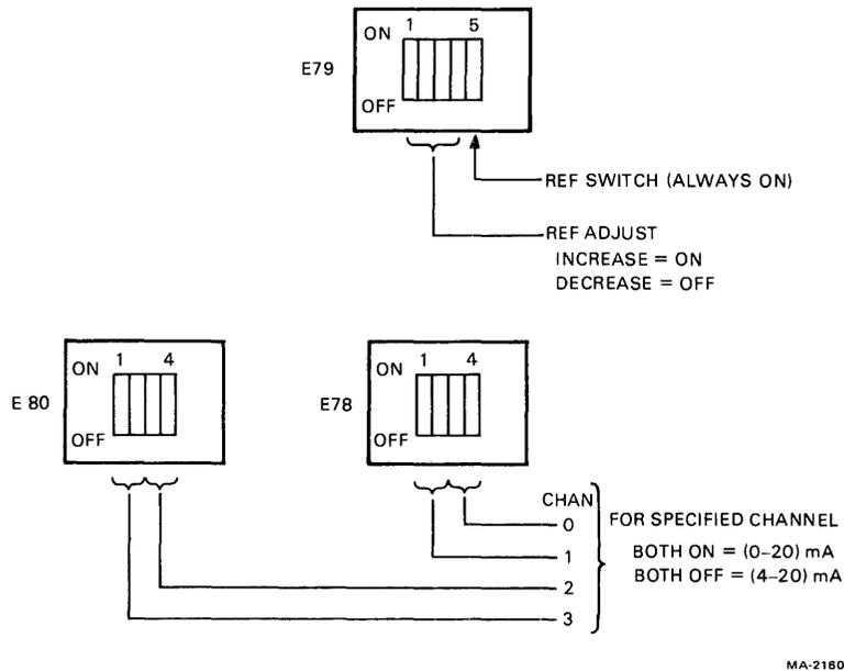
Figure 6-23-9 Voltage Reference and Current Mode Switches
