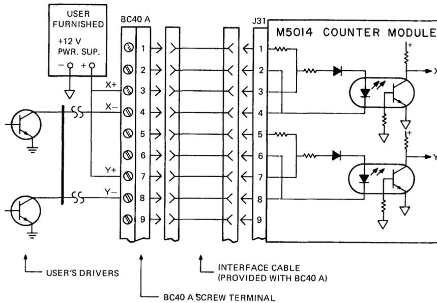
Figure 6-7-12 M5014 Isolated Low Level Input Application
