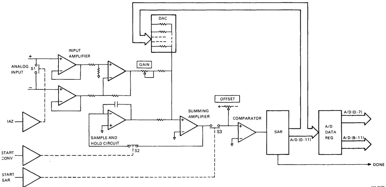
Figure 6-18-6 A/D Converter Section, Simplified Circuit Diagram
