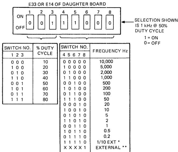
\* OUTPUT FREQUENCY IS 1/10 EXTERNAL INPUT FREQUENCY.
