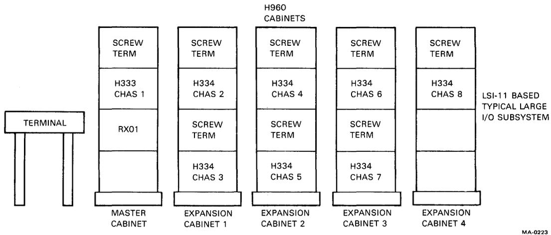
Figure 2-1 IP300 LSI-11 Based Configurations
