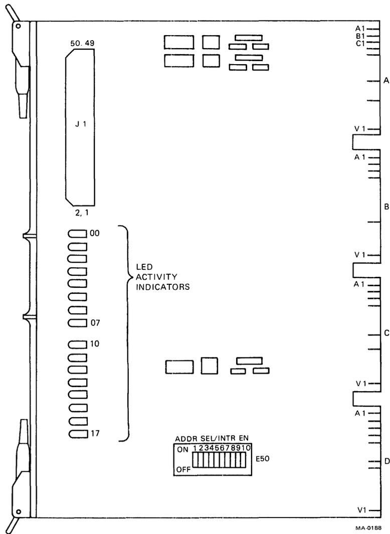
Figure 6-4-2 M5012 16-Bit Isolated DC Input
