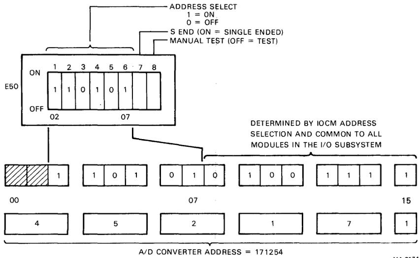
Figure 6-18-9 A014 Module - Address, S END, and Manual Test Selection
