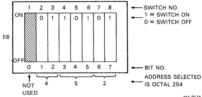
Figure 6-12-5 Address Selection Switch
