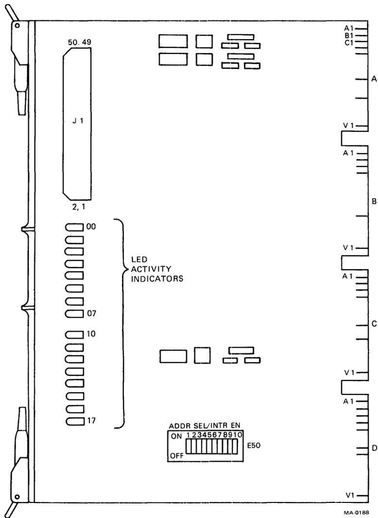
Figure 6-5-2 M5012-YA 16-Bit TTL Compatible Input Module
