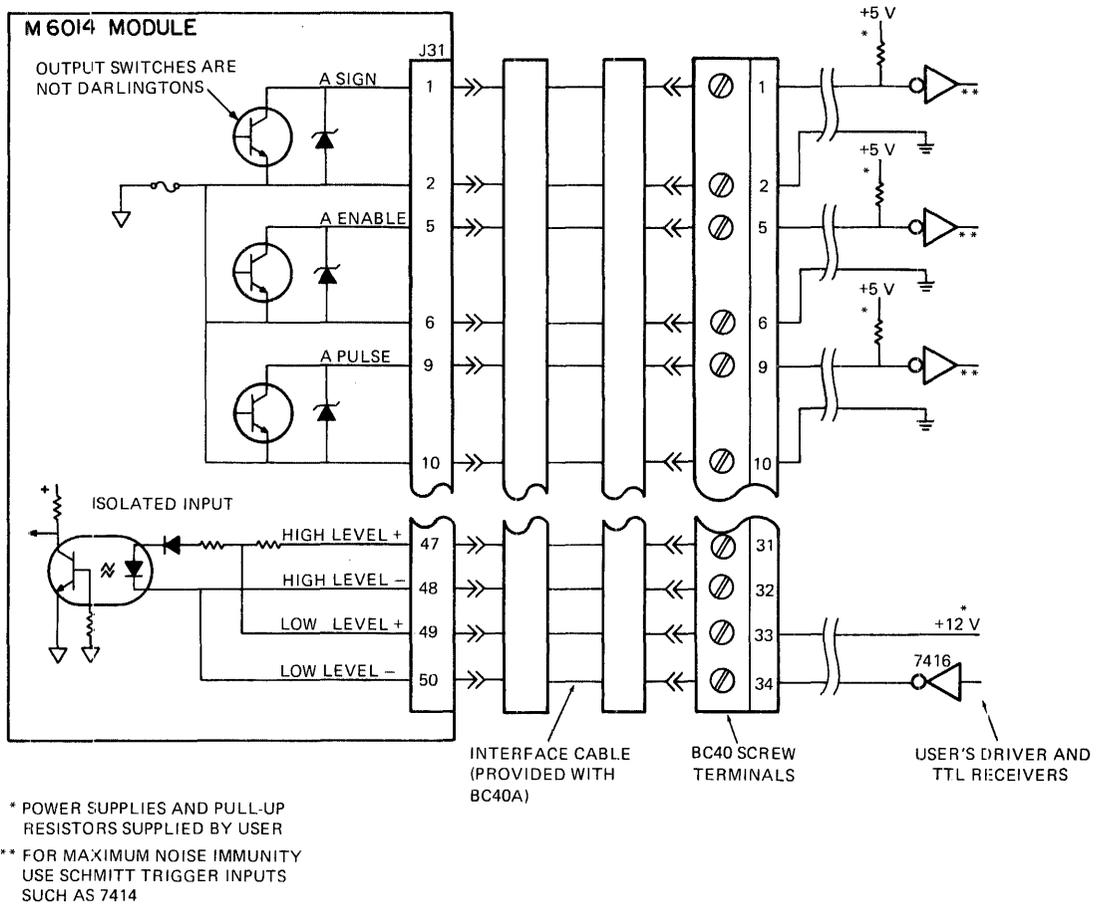
Figure 6-15-8 M6014 Typical TTL Interface
