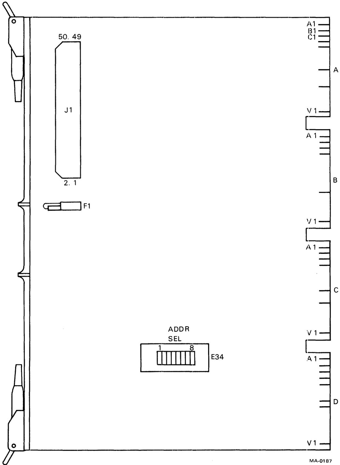
Figure 6-11-2 M6010-YA 32-Bit TTL-Compatible Output Module
