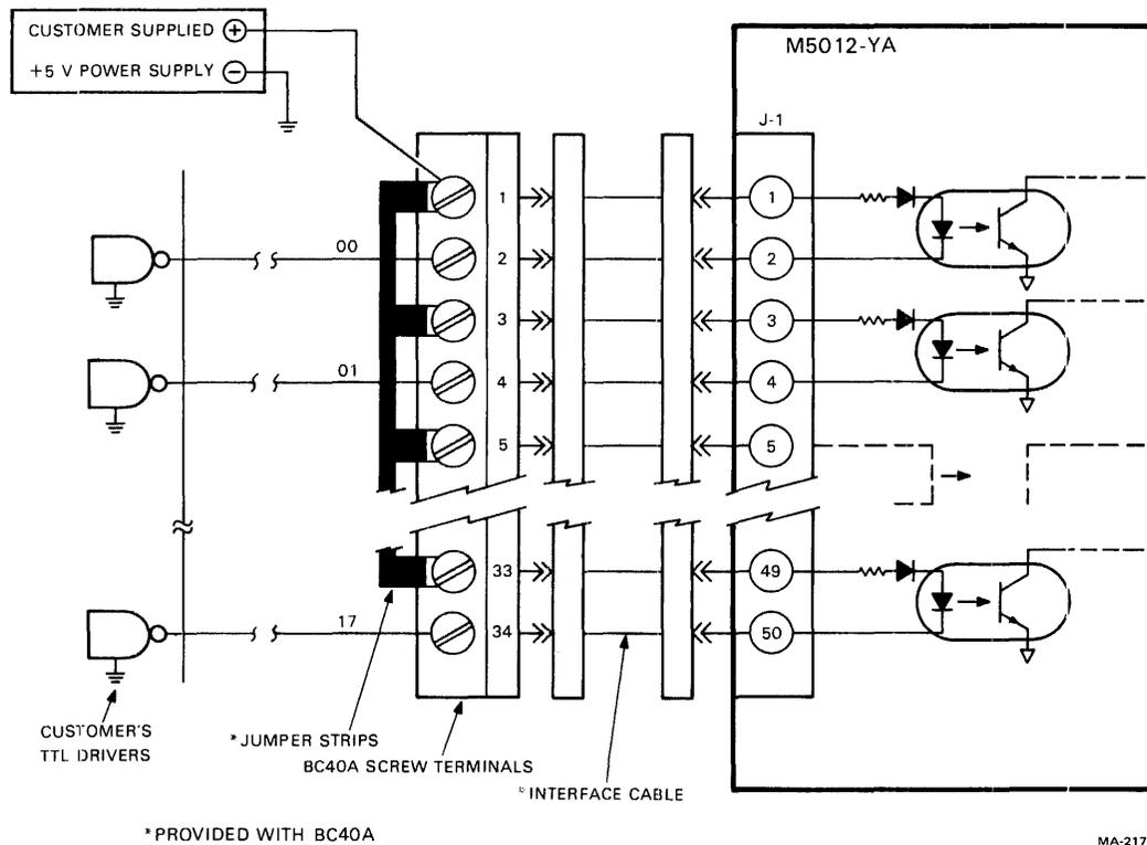
Figure 6-5-4 M5012-YA Typical TTL Field Interface
