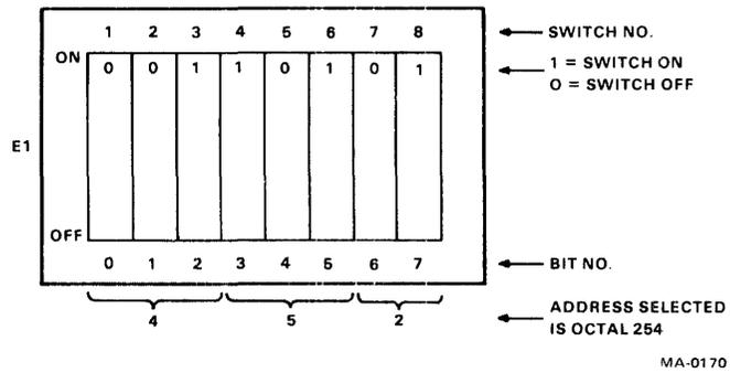
Figure 6-14-4 Address Selection Switch
