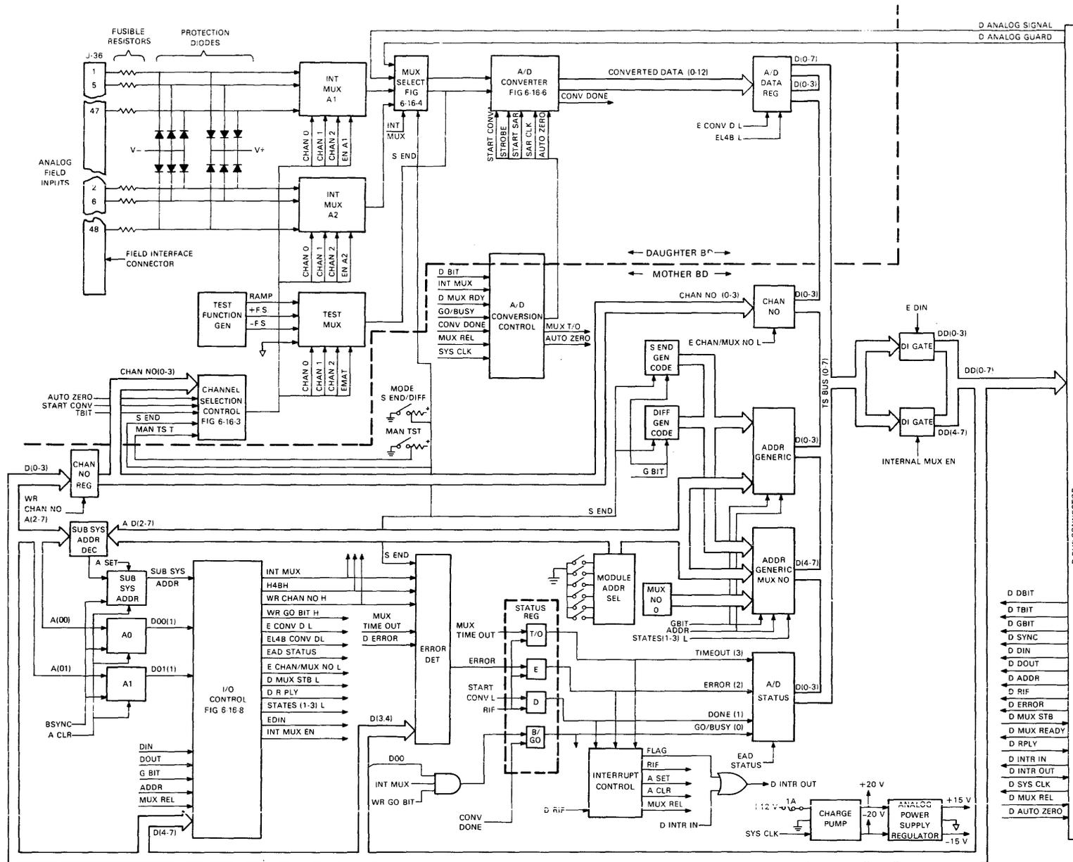
Figure 6-18-1 Module A014 A/D Converter, Block Diagram
