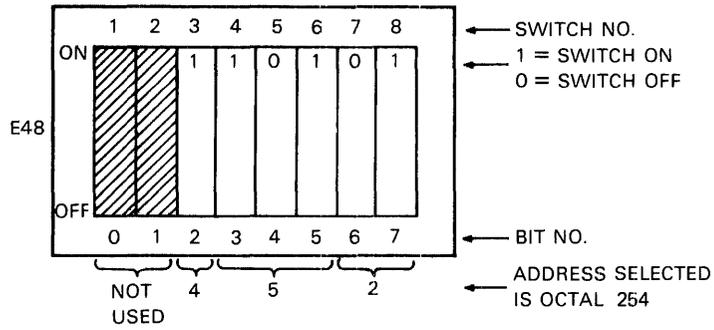
Figure 6-3-3 Address Selection Switch
