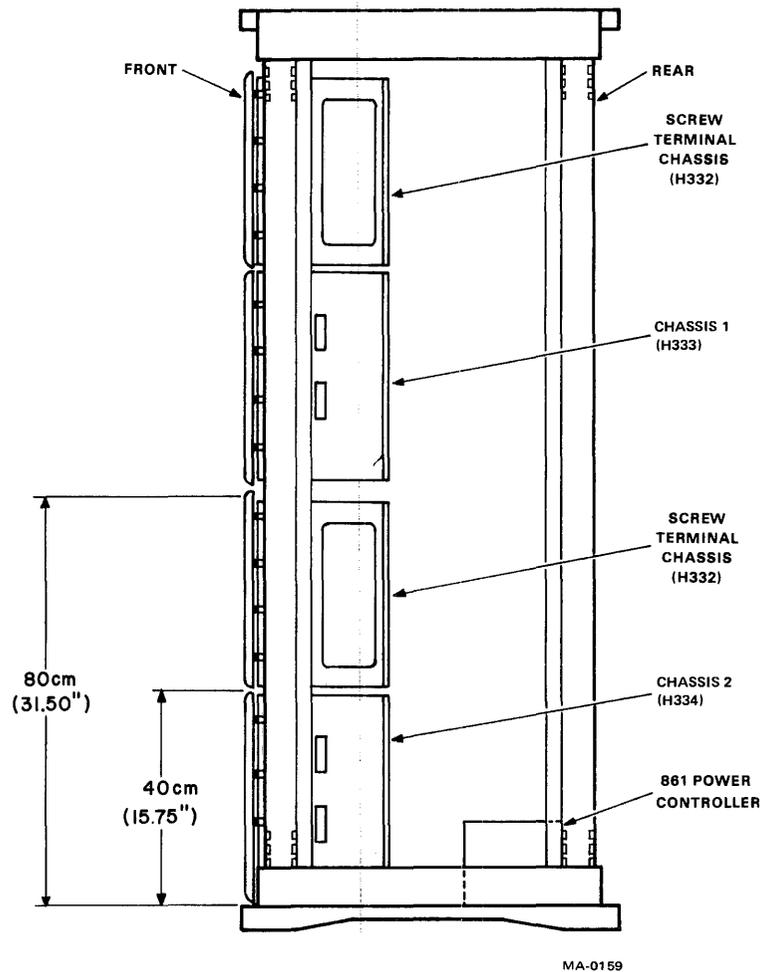
Figure 2-4 Expanded I/O Subsystem
