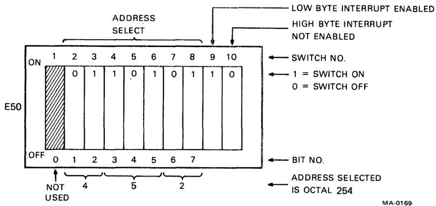
Figure 6-5-3 M5012-YA Address Selection and Interrupt Enable Switch
