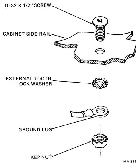
Figure 6-22-5 Ground Wire Fastening
