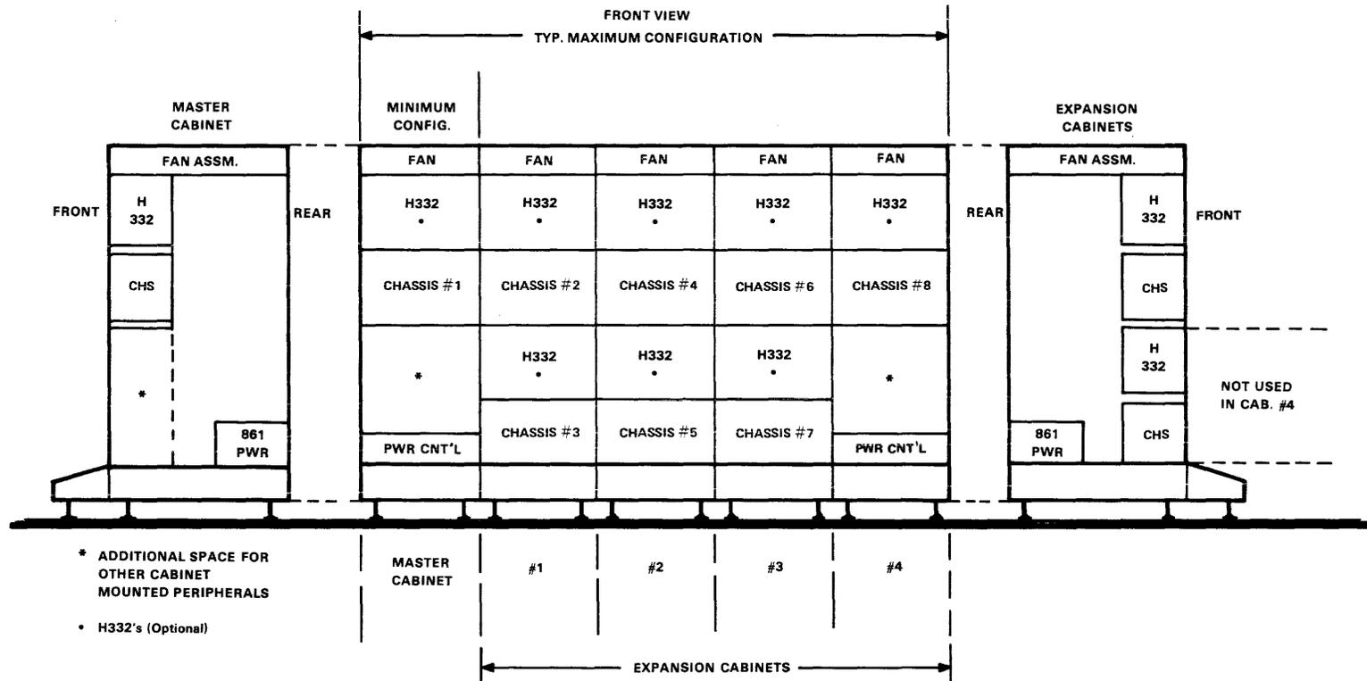
Figure 3-3 I/O Subsystem Front View
