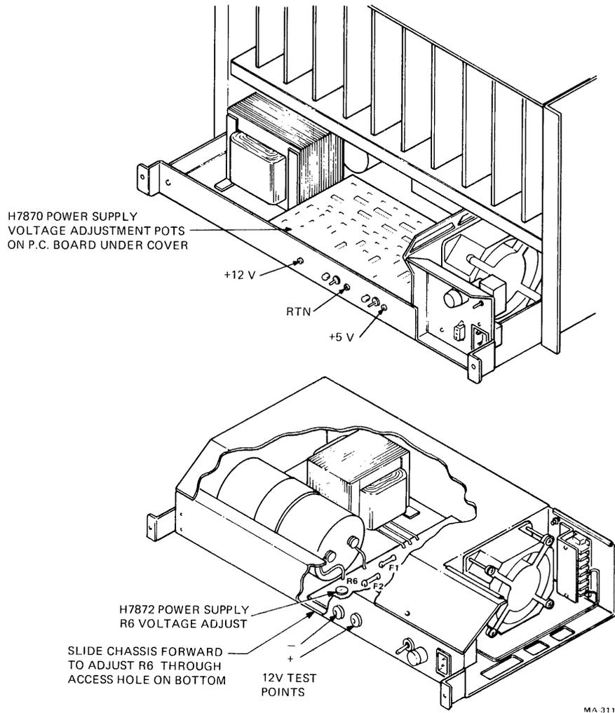
Figure 7-1 Power Supply Adjustments
