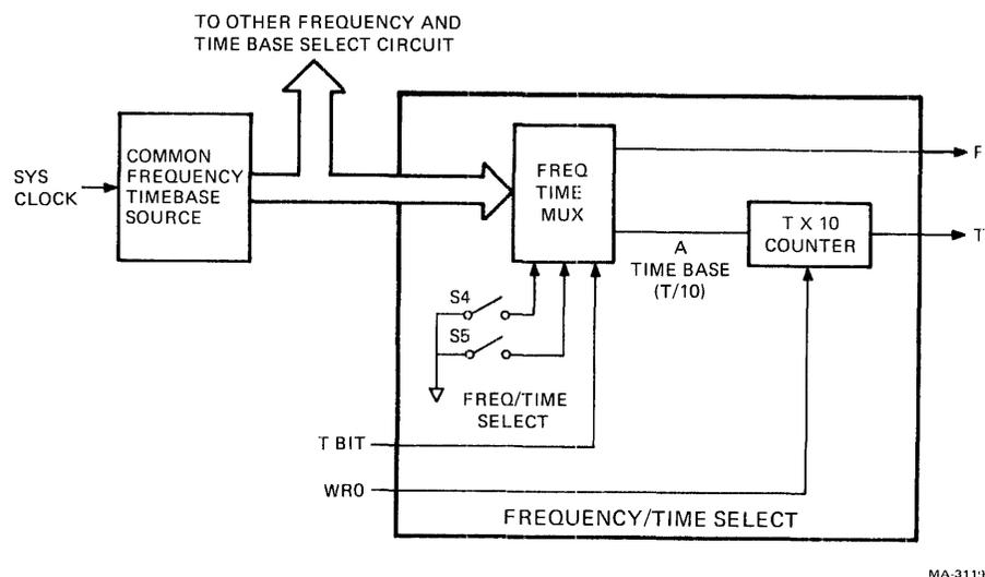
Figure 6-7-7 Frequency and Time-Base Select Circuit
