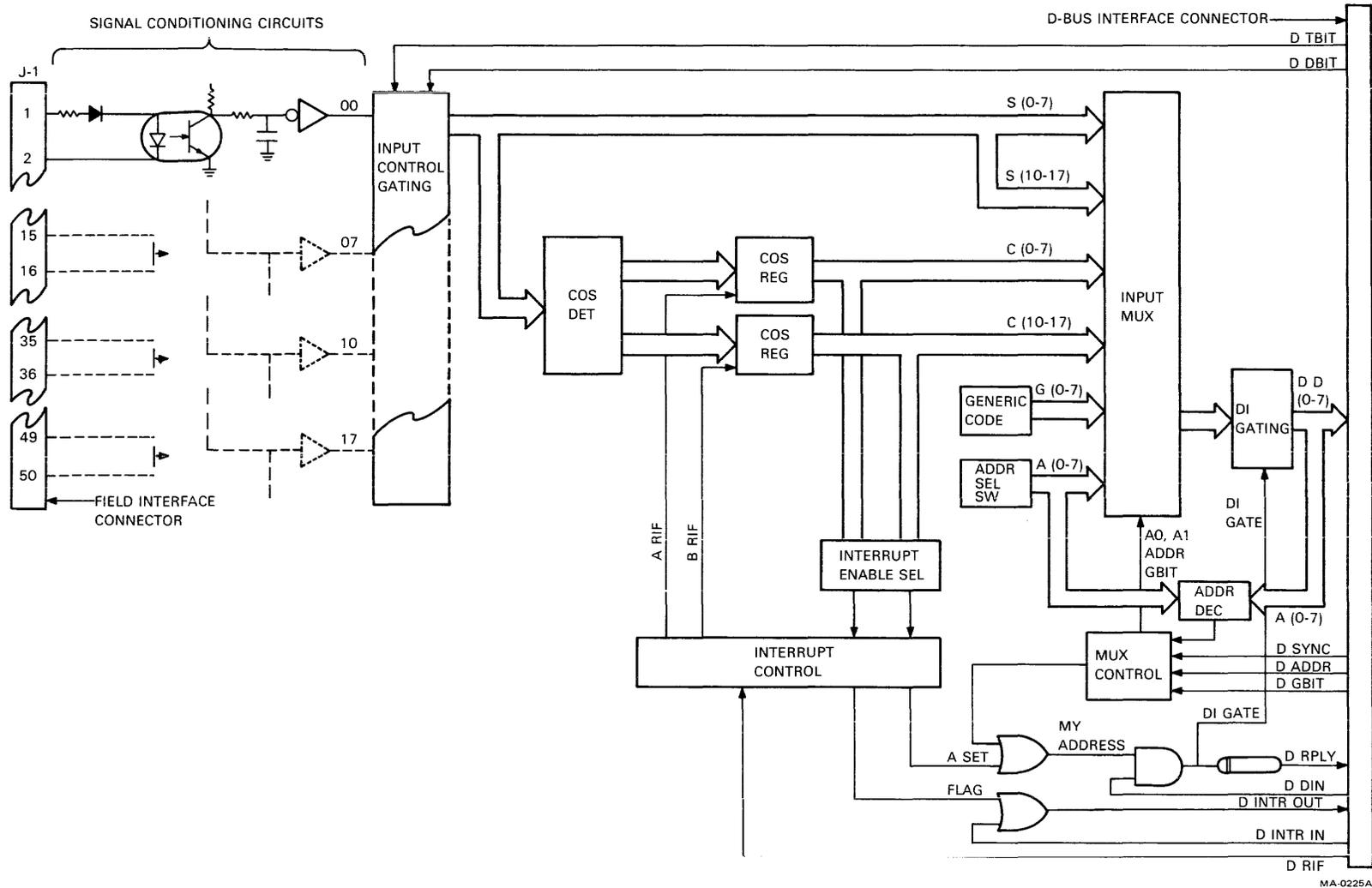
Figure 6-9-1 M5031 16-Bit Isolated COS Input Module Simplified Block Diagram
