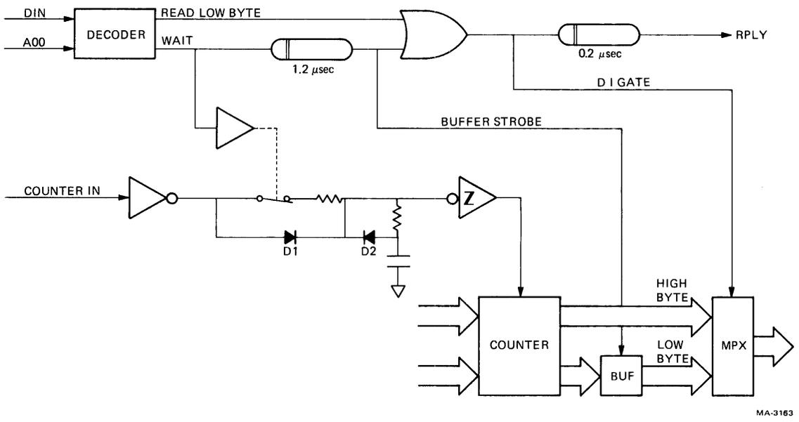
Figure 6-7-3 Anticoincidence Circuit
