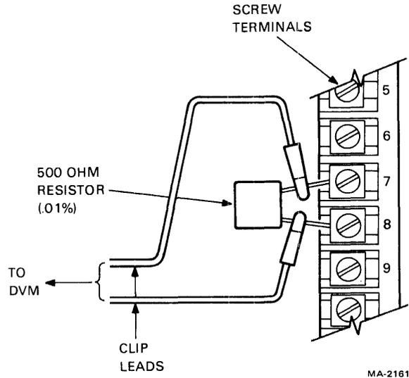
Figure 6-23-10 Calibration Resistor and Meter Lead Placement
