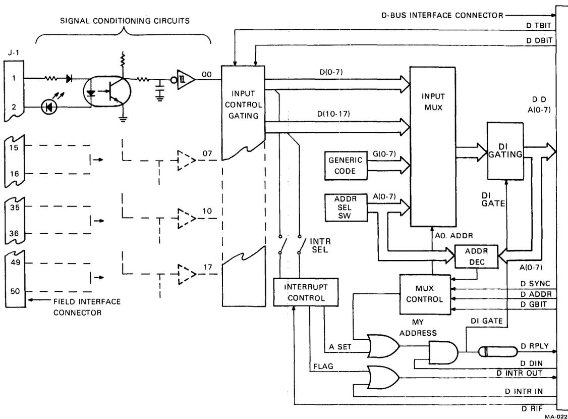
Figure 6-4-1 Module M5012, 16-Bit Isolated DC Input Module, Simplified Block Diagram
