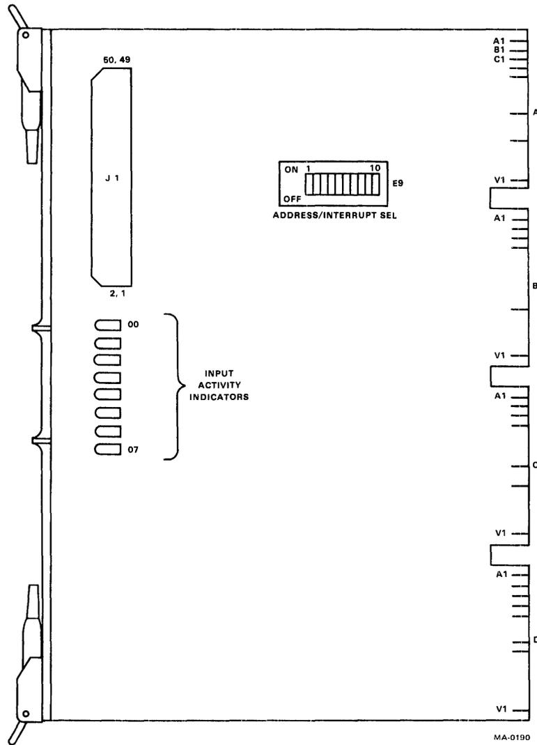
Figure 6-6-2 M5013 AC Input Module
