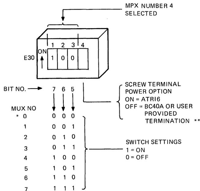
\* CODE ZERO IS USED ONLY FOR THE A014 MODULE'S INTERNAL MULTIPLEXER, THEREFORE, THIS IS AN ILLEGAL CONFIGURATION.
