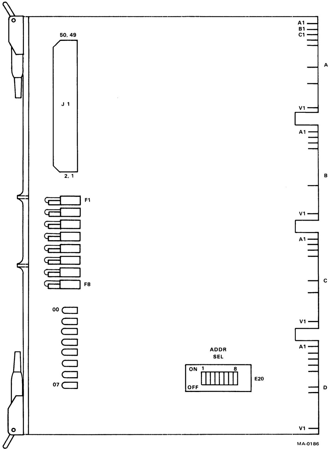
Figure 6-13-2 M6012 8-Bit Isolated DC Output
