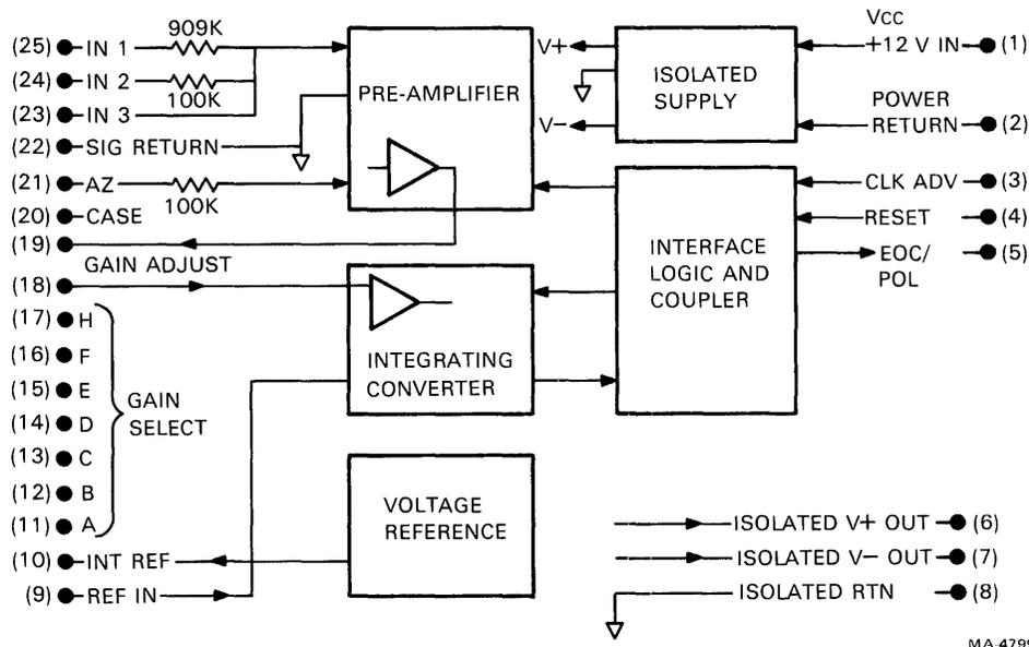
Figure 6-21-6 Isolated, Selectable Range Integrating Converter
