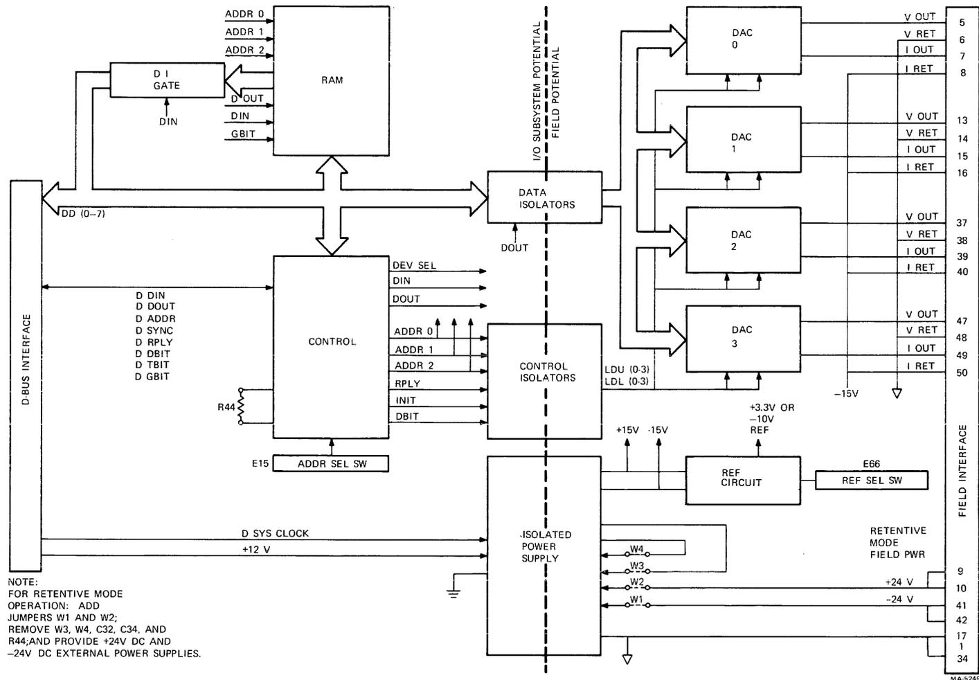
Figure 6-24-1 A631 DAC Block Diagram
