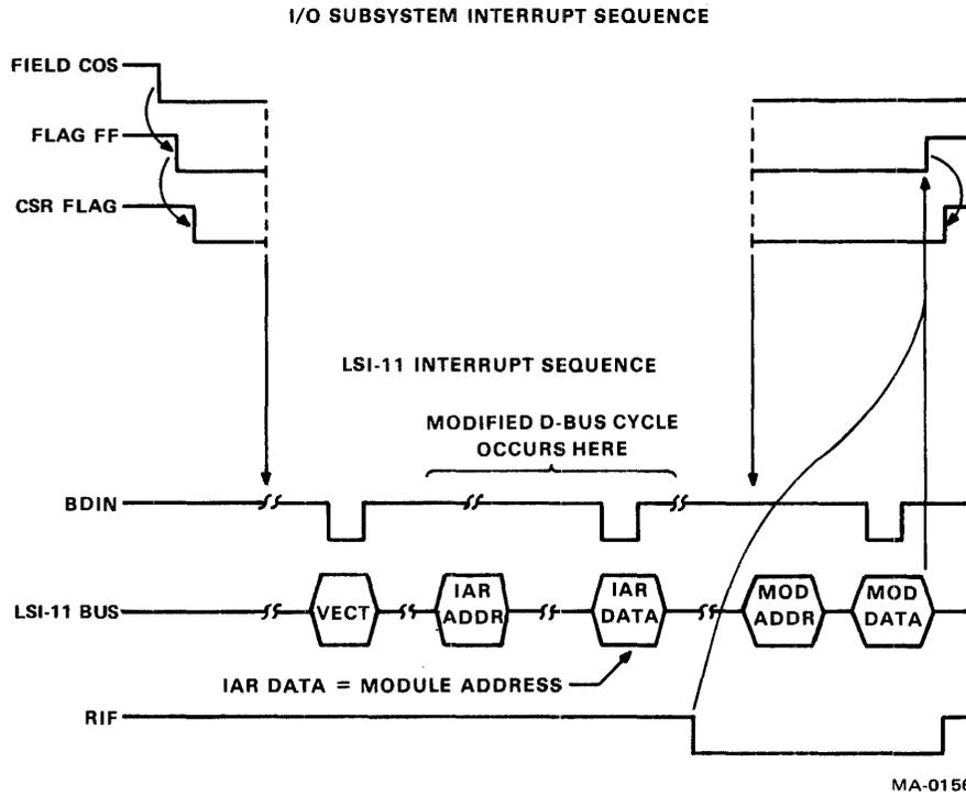
Figure 5-10 Interrupt Timing
