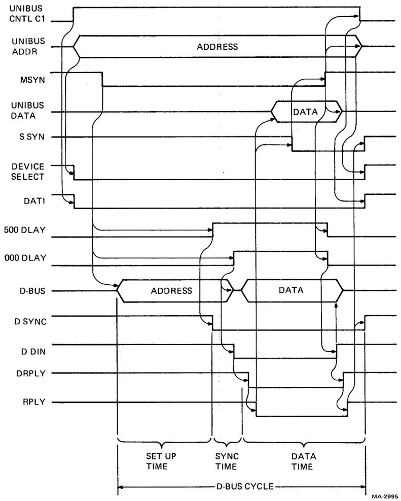
Figure 5-13 DATA I Cycle Timing
