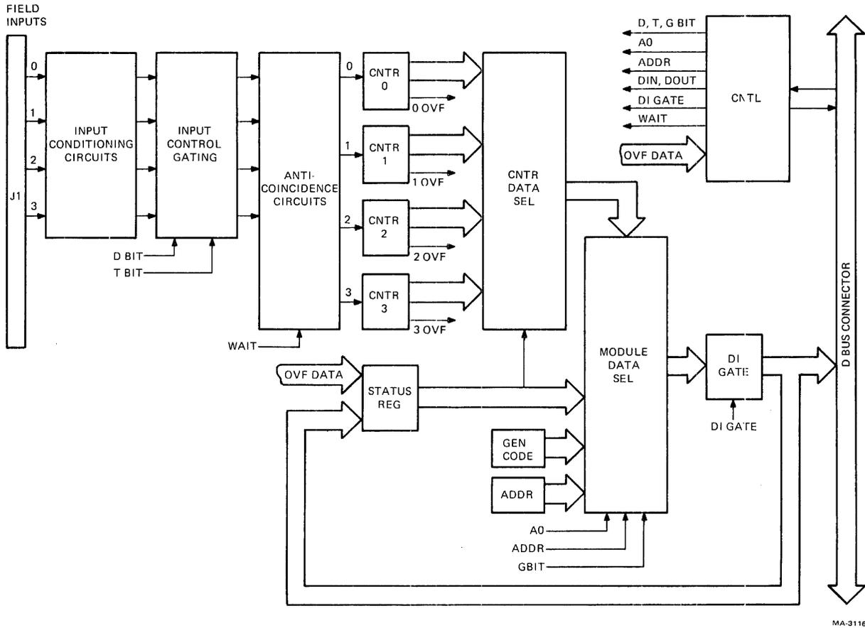
Figure 6-8-1 M5016 Quad Input Counter/Prescaler Block Diagram
