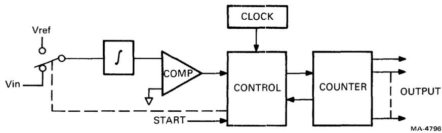
Figure 6-21-3 Simplified Dual Slope Converter
