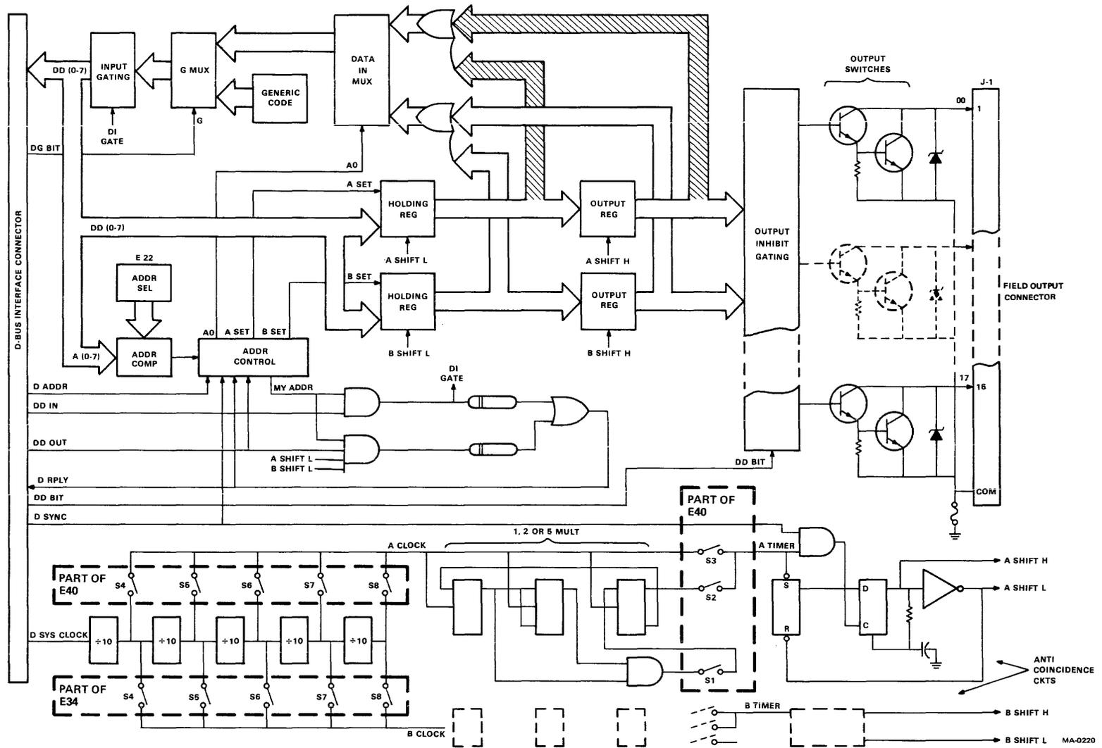
Figure 6-12-1 M6011 16-Bit One-Shot Output Simplified Block Diagram
