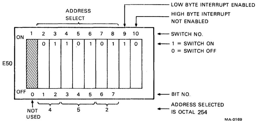
Figure 6-4-3 Address Selection and Interrupt Enable
