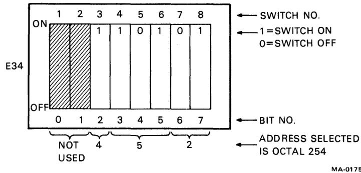
Figure 6-10-3 Address Selection Switch
