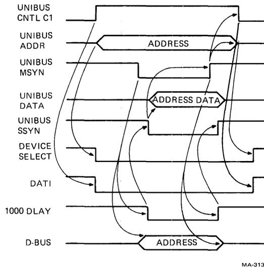
Figure 5-22 Maintenance Cycle Timing
