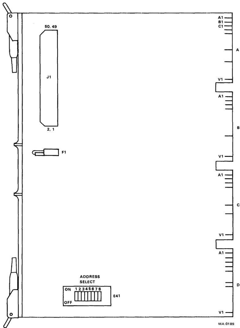
Figure 6-2-2 M5010 32-Bit DC Sense Module
