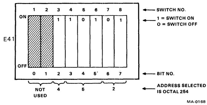
Figure 6-2-3 Address Selection Switch
