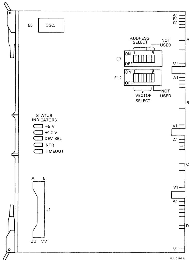
Figure 3-27 M7959 I/O Control Module
