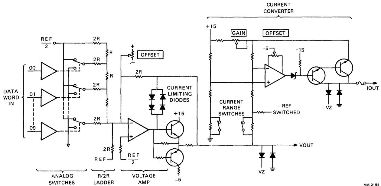
Figure 6-23-4 DAC Circuit
