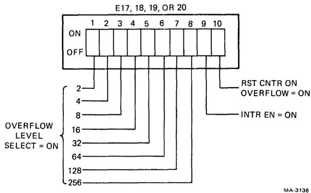
Figure 6-8-8 Function Selector Switches
