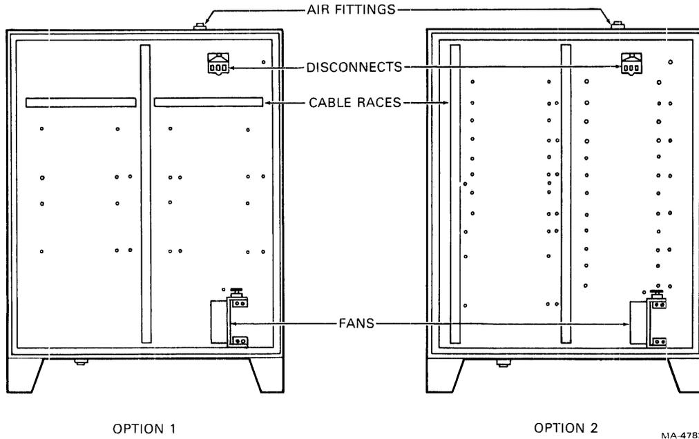
Figure 3-19 NEMA-12 Type Enclosures
