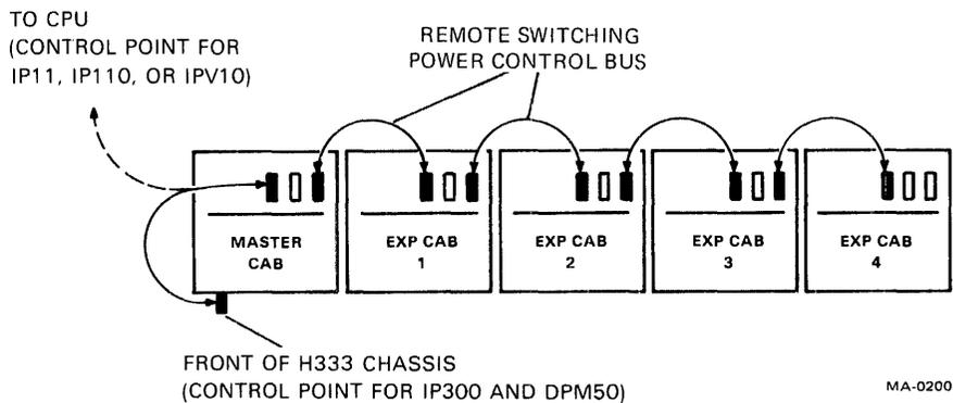
Figure 3-5 Remote Power Connections
