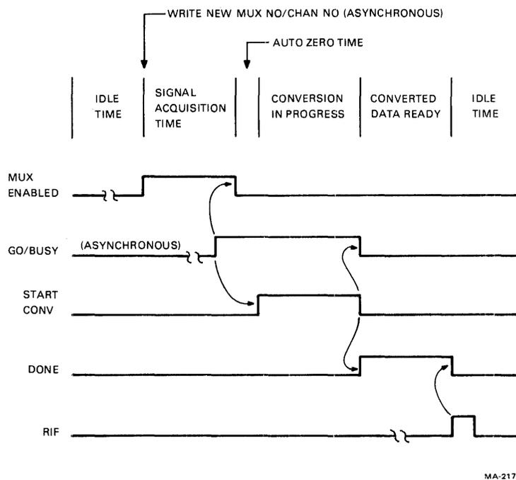
Figure 6-18-7 Analog Subsystem Timing
