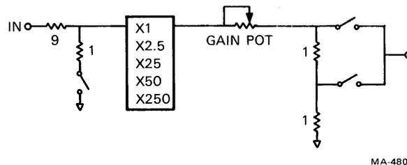
Figure 6-21-11 Analog Input Configuration
