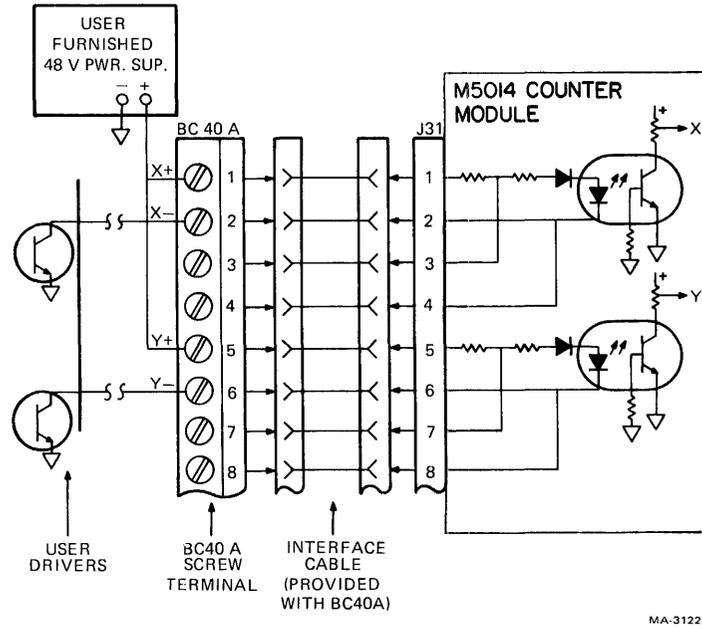
Figure 6-7-11 M5014 Isolated High Level Input Application
