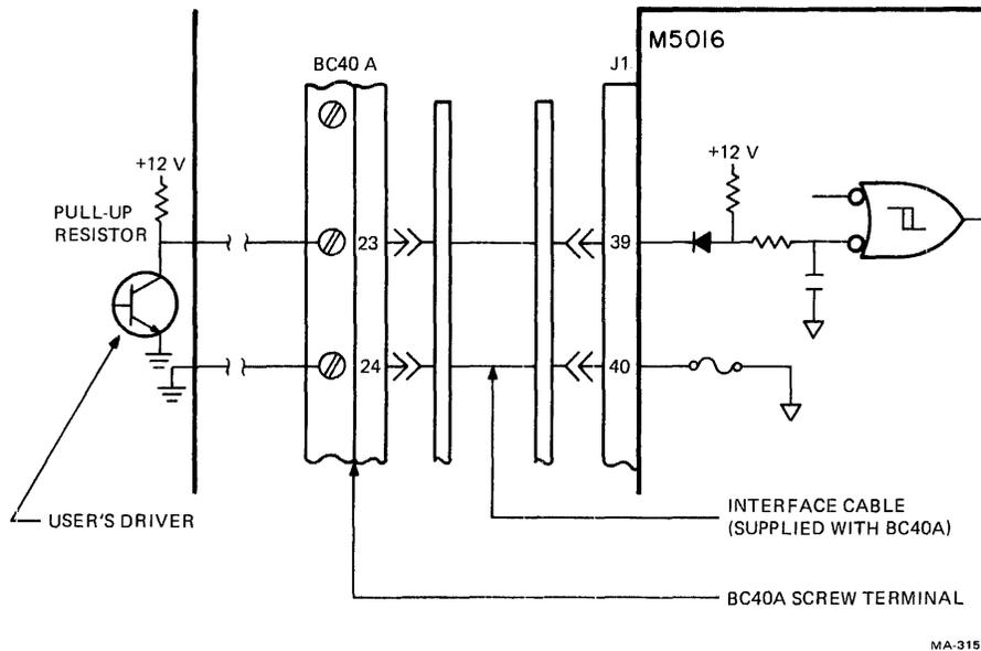
Figure 6-8-7 Counter 2 Nonisolated Input Application
