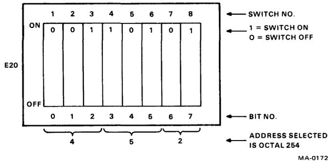
Figure 6-13-3 Address Selection Switch
