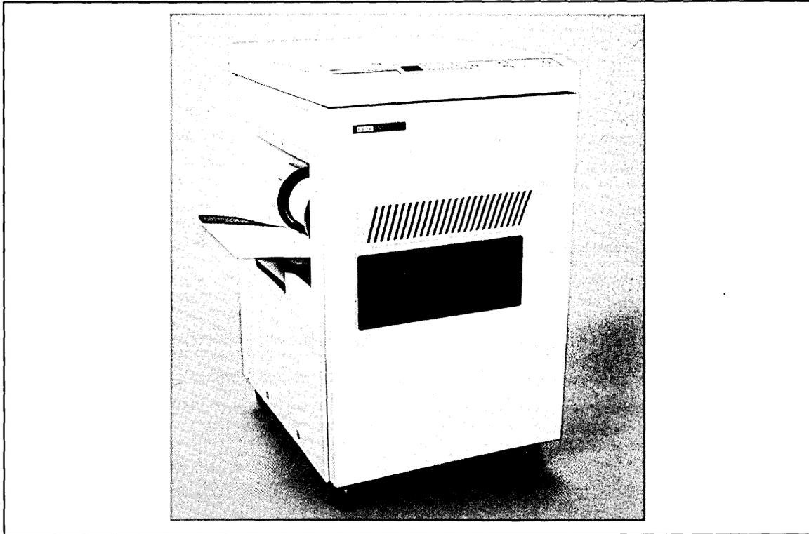
The LNO1 page printer is a high-quality nonimpact printer that employs laser technology. The LNO1 provides the speed of a lineprinter with exceptional print quality. Using electrophotographic imaging and xerographic printing, the LNO1 prints one page at a time, twelve pages per minute. The print resolution of 300 x 300 dots per square in produces perfectly formed characters of even density and alignment. Since every page is an original, every copy is as crisp and clear as the first.
