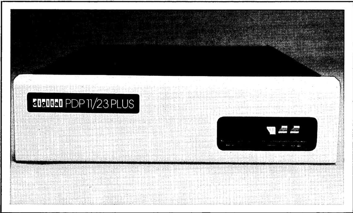
The PDP-11/23-PLUS is available in two rack-mountable variations: a standard 13.3 cm (5.25 in) PDP-11/23-PLUS and an 8.8 cm (3.5 in) PDP-11/23-S.
