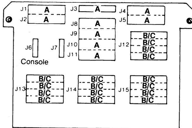
An adapter plate is also included to convert four size A inserts (J8-J11) to one size C insert.
