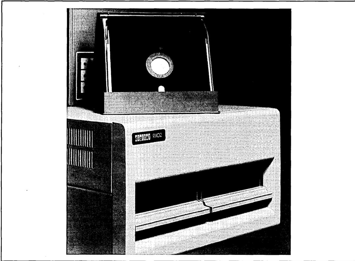
The RX02 double-density floppy disk drive provides an industry-compatible format and highly reliable operation. Direct memory access (DMA) is used to provide rapid data transfer and efficient utilization of the host processor. These subsystems include two RX02 0.5 MB drives (for a total of one MB) and a controller with interconnect cabling. The dual drives are packaged as a cabinet-mountable or tabletop unit.
