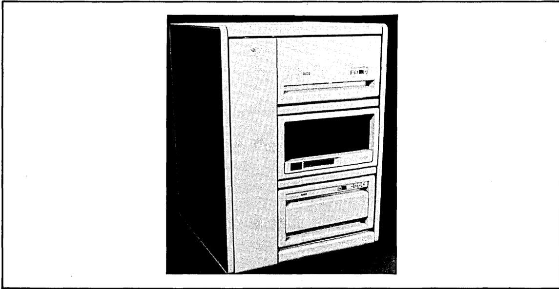
The PDP-11/44 RA80/RL02 system provides all the standard features of the PDP-11/44-DA(DB) box product plus an expansion backplane and 121 MB fixed and 10.4 MB removable disk storage.
