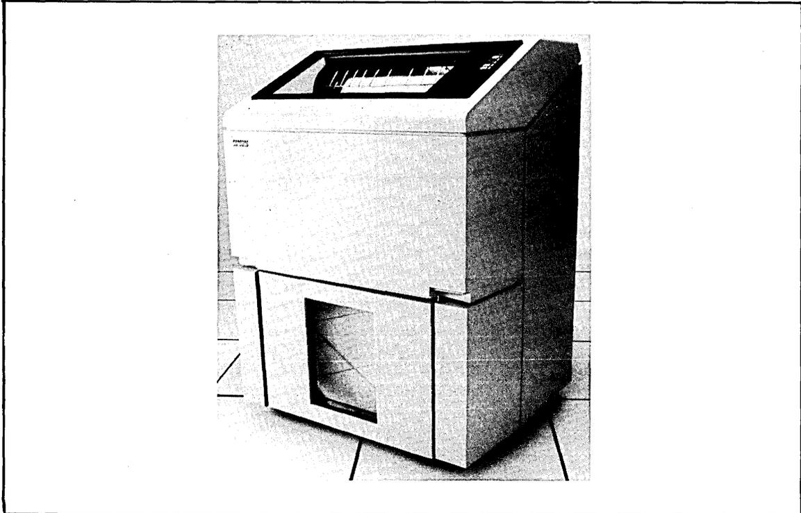
The LP27 is a 132-column, fully formed character, impact lineprinter. It includes both 64 and 96 character American print bands as standard on all versions. Maximum print throughput is 1200 lines per minute using the 64 character band or 800 lines per minute with the 96-character band.
