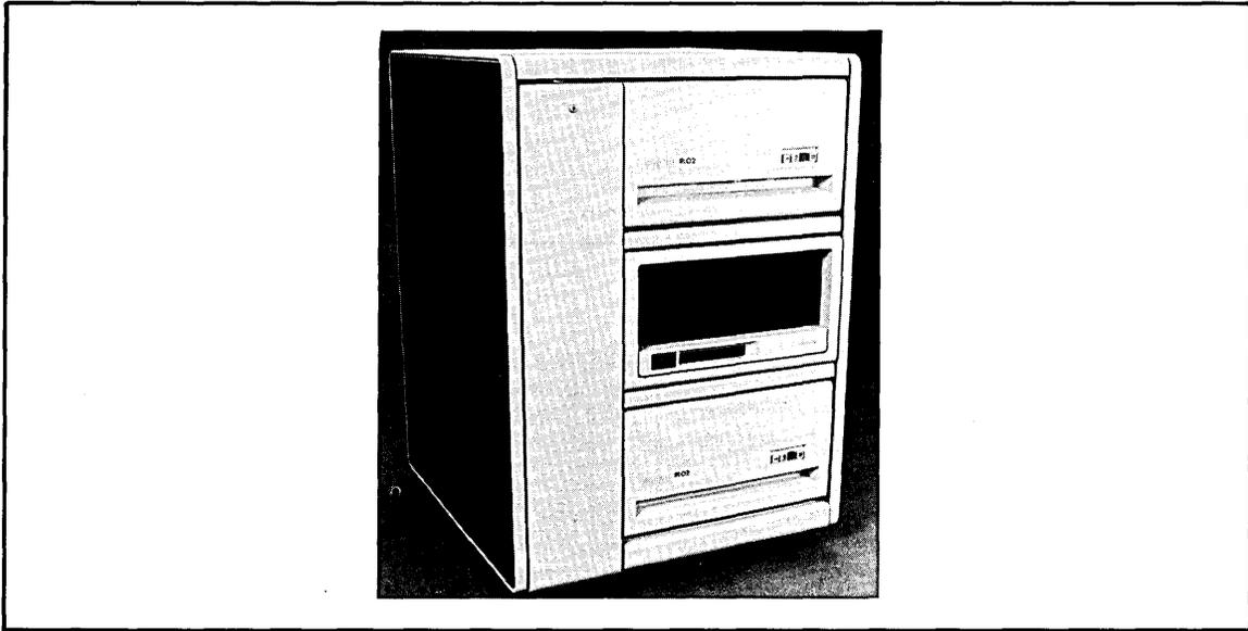
The PDP-11/44 Dual RLO2 system configuration provides all the standard features of the PDP-11/44-DA(DB) and 20.8 MB of removable mass storage capacity.
