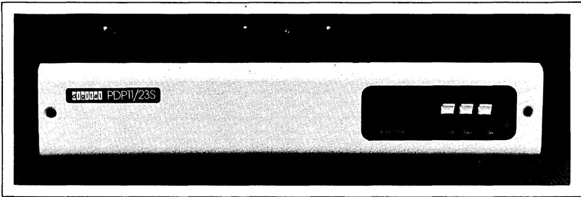
The PDP-11/23-S is an 8.8 cm (3.5 in) high, rack-mountable processor offered in two versions, one with NMOS RAM memory, the other with non-volatile CMOS RAM memory. The I/O Connection panel (H3012) for this model accepts the same system options as the MICRO/PDP-11 and the PDP-11/23-PLUS. The PDP-11/23-S is not orderable in a system configuration.
