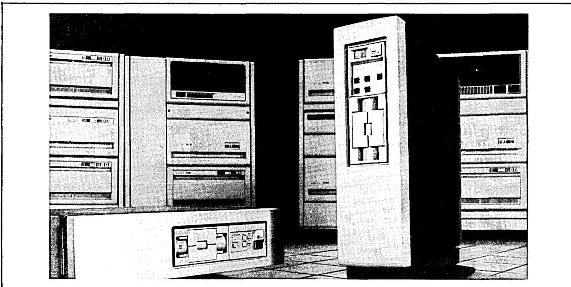
The MICRO/PDP-11 family of small, multiuser computers consists of both floppy-disk and fixed-plus-floppy systems. They are packaged to fit easily under a desk or worktable, on a tabletop, or as a rack mountable box enclosure, and can be expanded to support up to 10 users.
