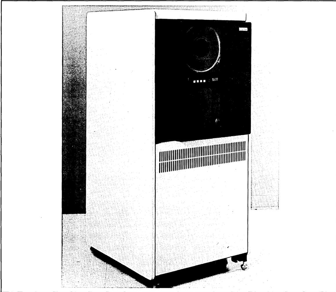
The TU77 UNIBUS magnetic tape subsystem includes the controller, a tape formatter, and one nine-track TU77 tape transport. The TU77 tape transport uses industry-compatible recording densities of 1600 b/in (Phase Encoded) and 800 b/in (Non-Return to Zero Inverted) selectable under program control. The subsystem is available with controllers for UNIBUS PDP-11 systems. The TU77 tape transport is available mounted in a 152.4 cm (60 in) H9602 single-width highboy cabinet.
