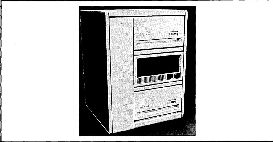
The PDP-11/24 Dual RLO2 system configuration provides all the standard features of the PDP-11/24 DC(DD) box product plus 20.8 MB of disk storage capacity.
