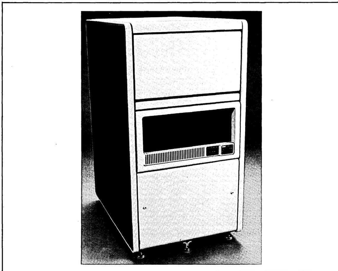
The PDP-11/24 is available in a cabinet-mounted model. It provides a foundation for building tailored system configurations and includes the 11/24-DC(DD) box product housed in an H9642 CPU cabinet.
