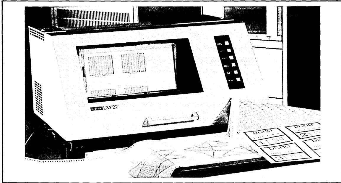
The LXY12 and LXY22 graphics lineprinters are versatile dot-matrix printers that combine the benefits of a line printer and a plotter in one product. These printers are compatible with all other Digital lineprinters, requiring no special software to use them as lineprinters.
