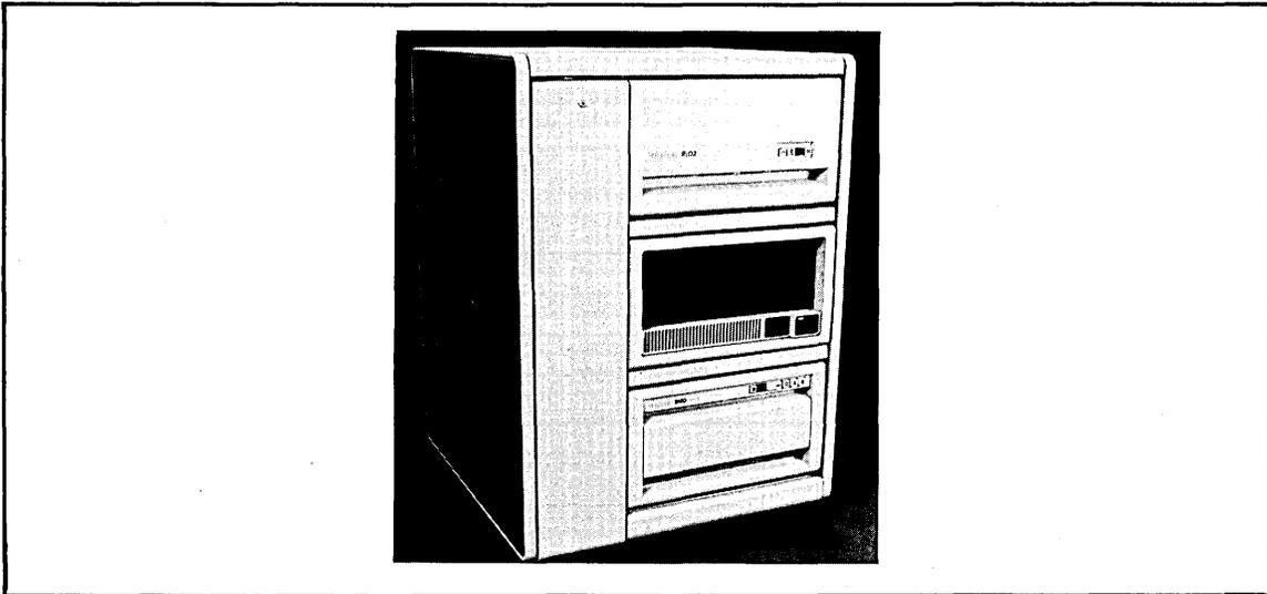
The PDP-11/24 RA80/RL02 configuration provides all the standard features of the PDP-11/24-DC(DD) box product and 121 MB fixed and 10 MB removable disk storage.
