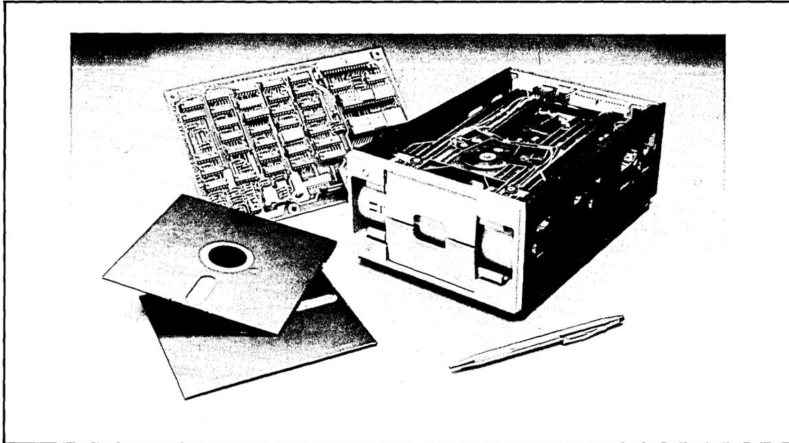
The RX50 dual diskette drive is a low-cost, compact, random access diskette drive. It stores data in fixed-length blocks on two 5.25-in flexible diskettes using preformatted industry-standard headers. Since the drive can accommodate two diskettes simultaneously, one diskette can be used for system programs, and the other allocated as a file device. The drive mechanism is packaged in a single compact housing, and its dimensions conform to the industry standards for 5.25-in disk media.
