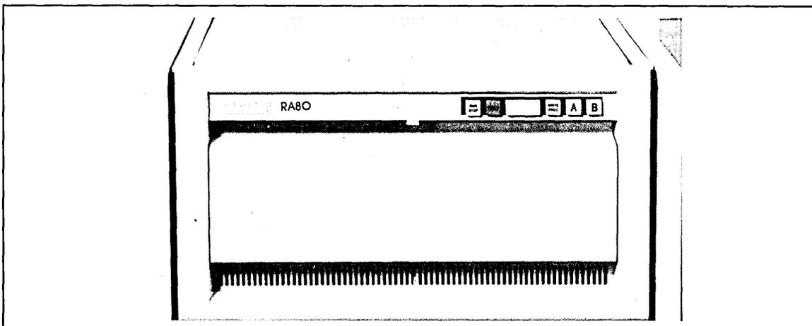
The RA80 disk subsystem uses Winchester fixed-disk technology to provide 121 MB of storage in a 26.6 cm (10.5 in) high package. The RA80 attaches to the high-performance, high-reliability microprocessor-based controller, the UDA50. The RA80 disk offers exceptional throughput performance, the result of an advanced mechanical design, which incorporates a rotary positioner-motor, computer-designed positioner arms, and lightweight Winchester head suspension.
