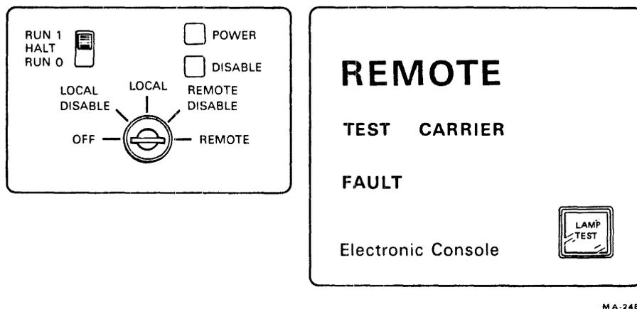
Figure 2-1 Electronic Console Panel Controls and Indicators
