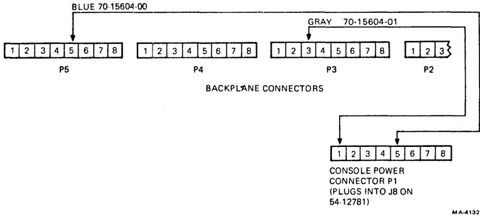
Figure 6-12 Power Jumper Installation
