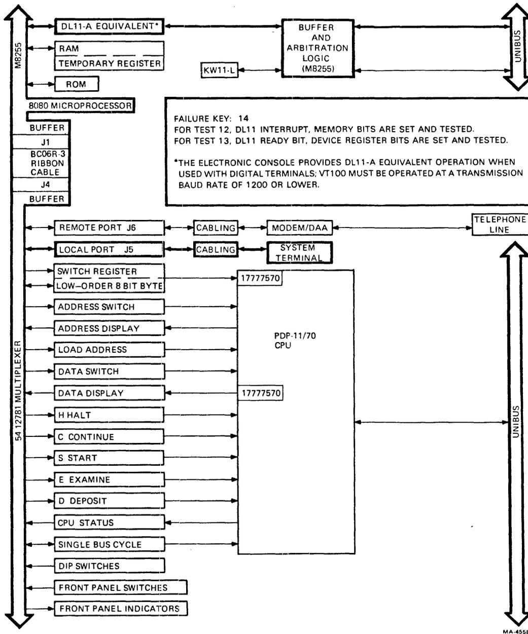
Figure 7-14 Failure Key 14
