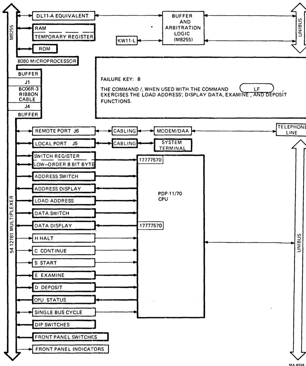
Figure 7-8 Failure Key 8
