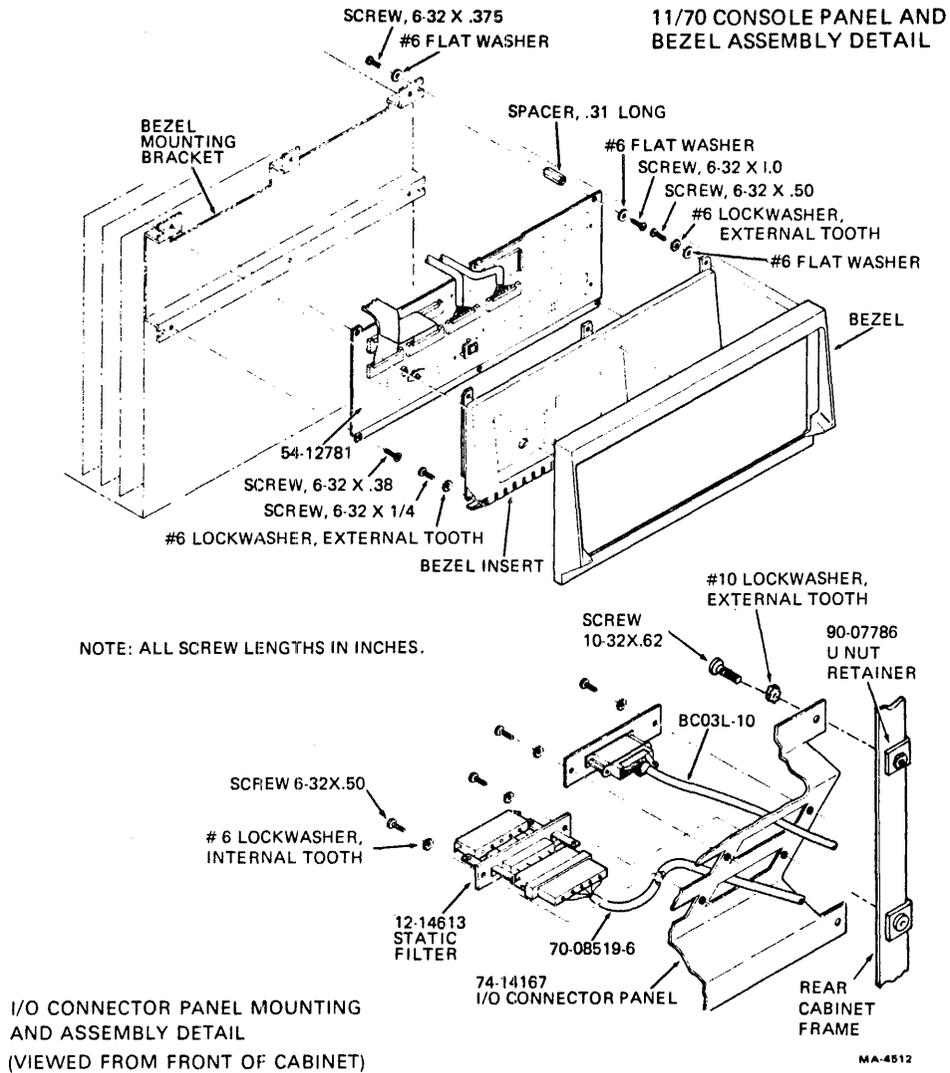
Figure 6-9 KY11-RB/KY11-RE Mechanical Assembly
