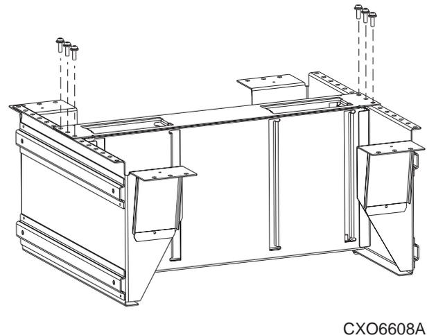
4. Using six (10-32 x 5/8 in) screws, secure the front of the ECB bracket to the upper and lower rear-mount shelf supports.
