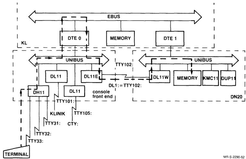
Figure 5-1 Path from Terminal to DN20
