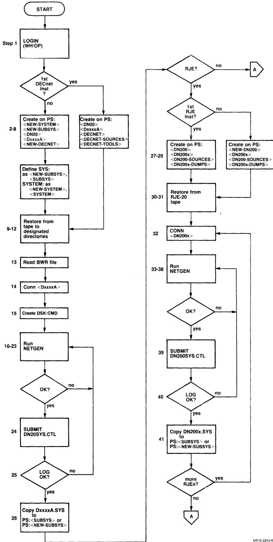
Figure 1-2 Installing DECnet-20 V3.0
