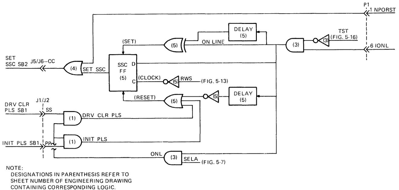
Figure 5-14 Slave Status Change Block Diagram
