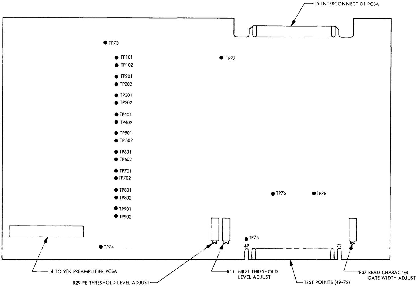
Figure 6-6 Data L PCBA Adjustments and Test Points
