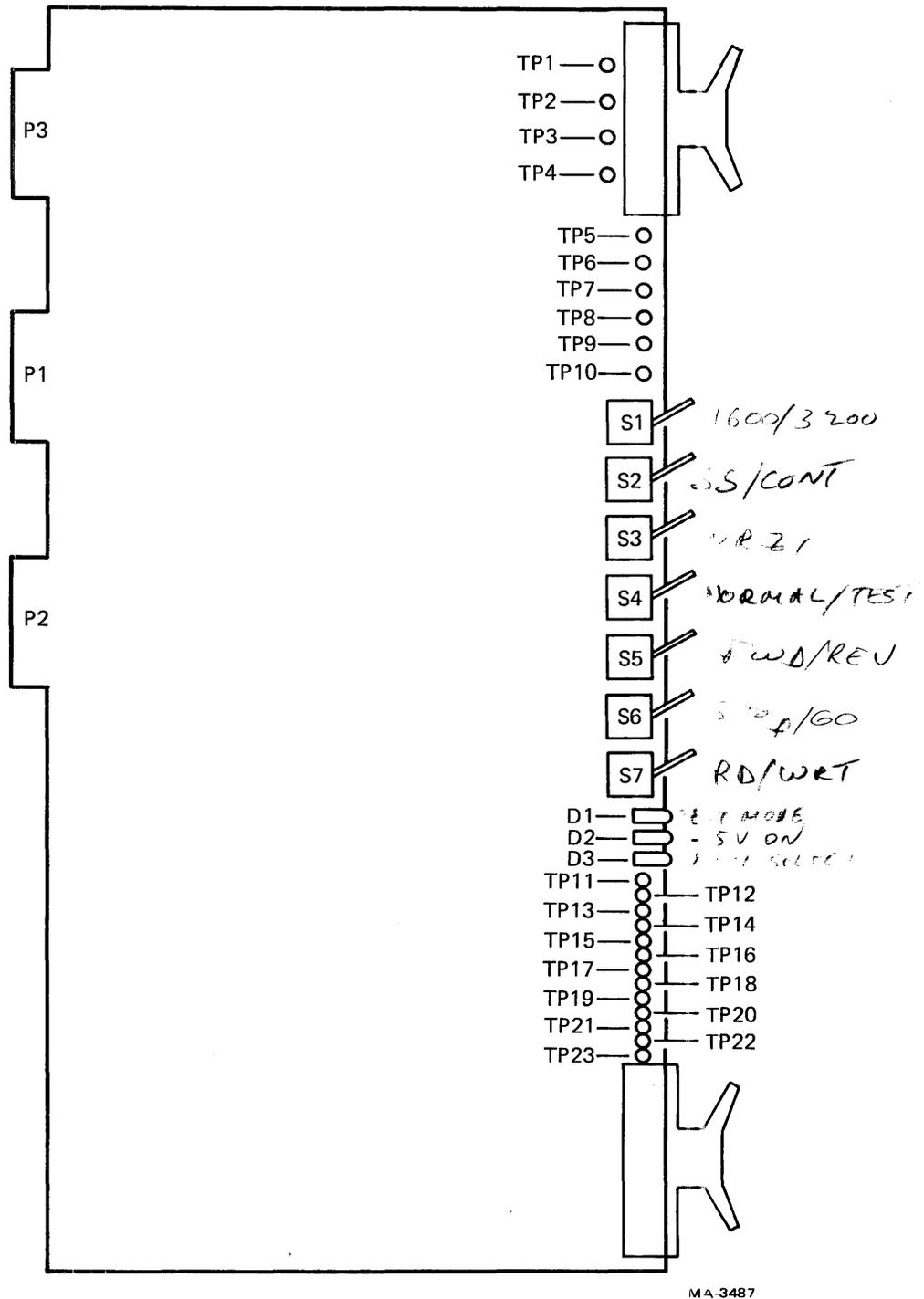
Figure 6-18 M8940 MTA Switches and Test Points
