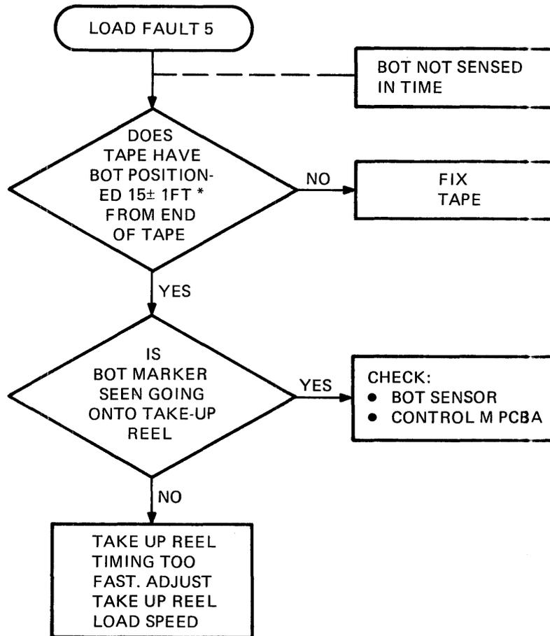
\*15 FT. IS OPTIMUM. TRANSPORT WILL LOAD AT UP TO 30 FT. IF PROBLEMS ARE EXPERIENCED DUE TO LEADER BEING TOO LONG, CUT IT DOWN TO 15 FT.
