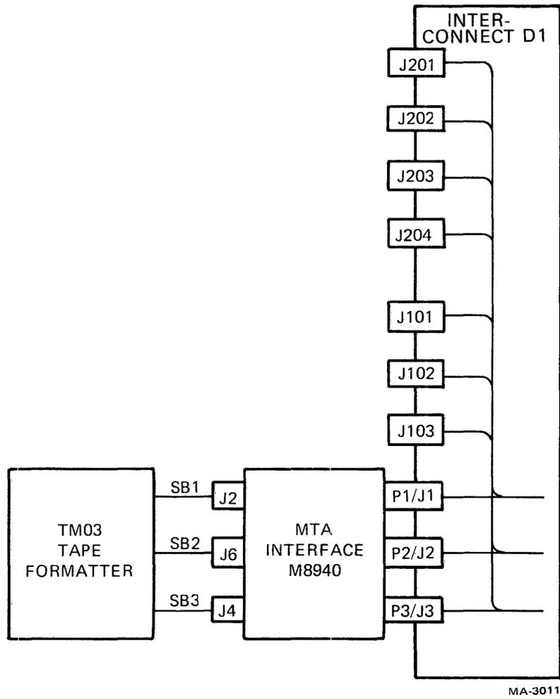
Figure 5-3 TU77 Interface Connections
