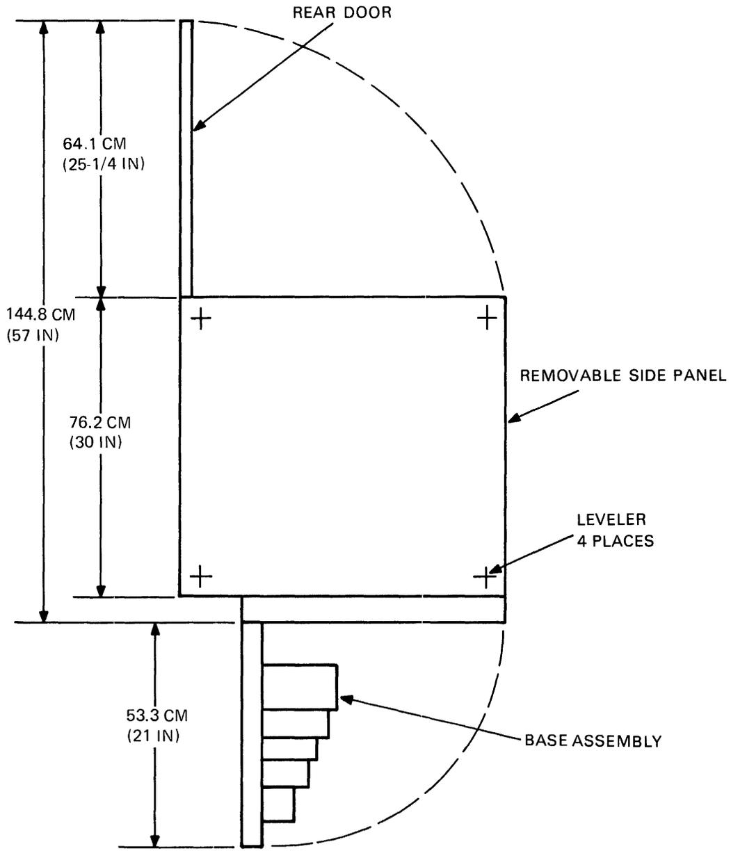
Figure 2-1 Space and Service Clearance, Top View
