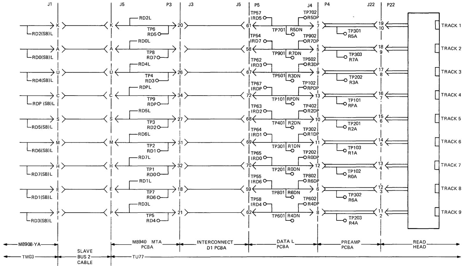
Figure 6-32 Read Data Path Test Points
