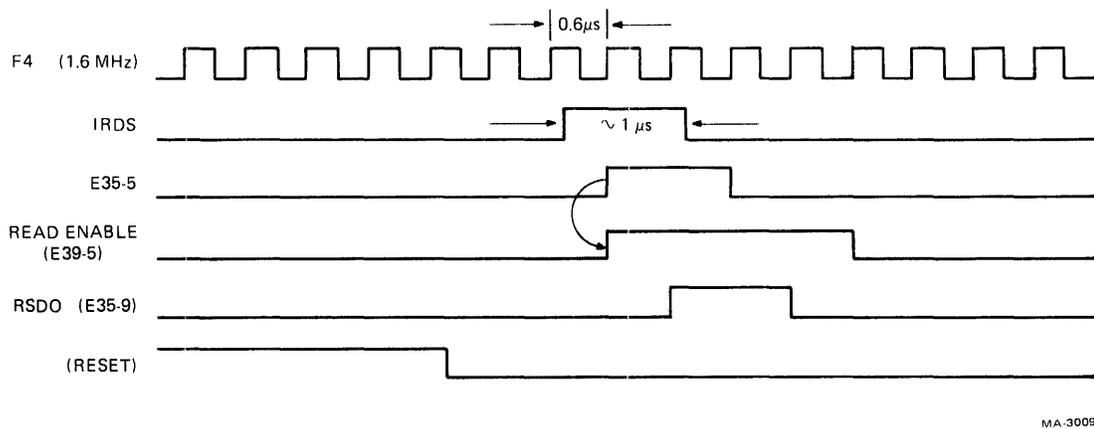
Figure 5-12 Timing of Read Strobe Sync Logic
