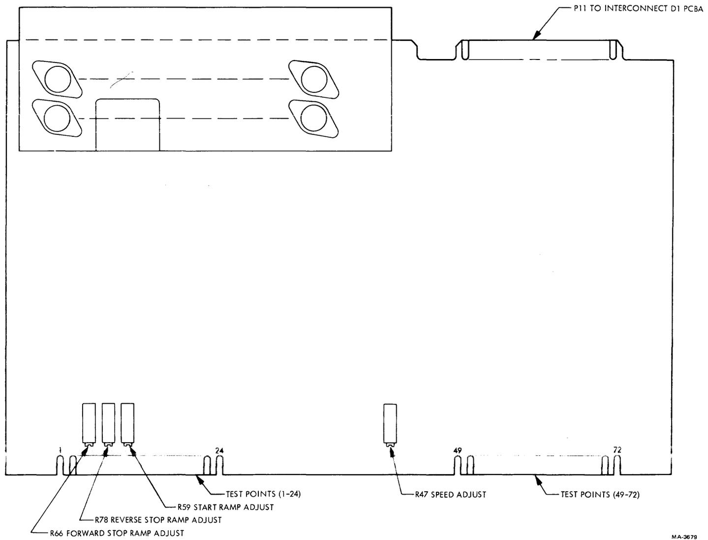
Figure 6-2 Capstan/Regulator PCBA Adjustments and Test Points
