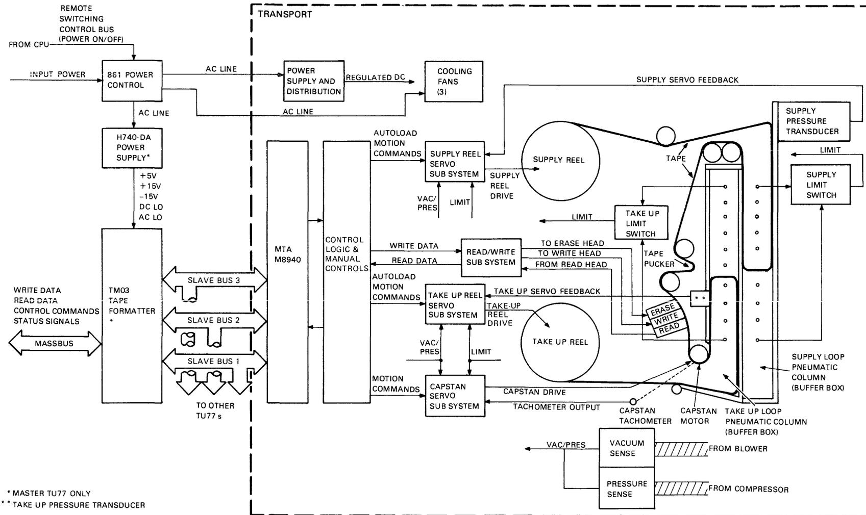
Figure 1-7 Master TU77 Functional Block Diagram
