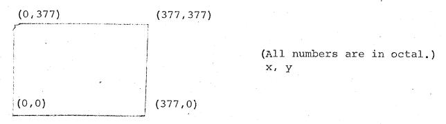
The X- and Y-Axis registers are loaded with data as indicated by the contents of the control fields in the Status Register. A point is then intensified as indicated by the contents of the BRIGHTNESS bits of the Status Register.
