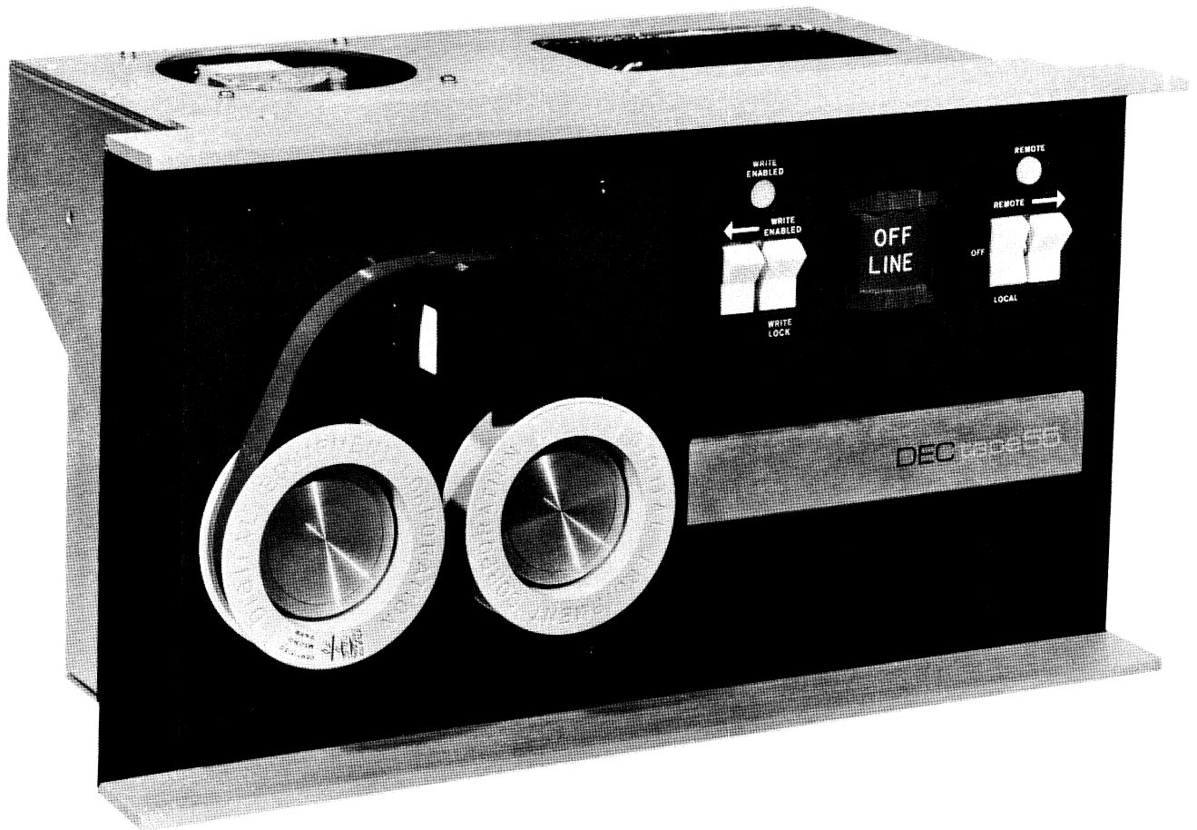
Figure 1-1 Type TU55 DECtape Transport
