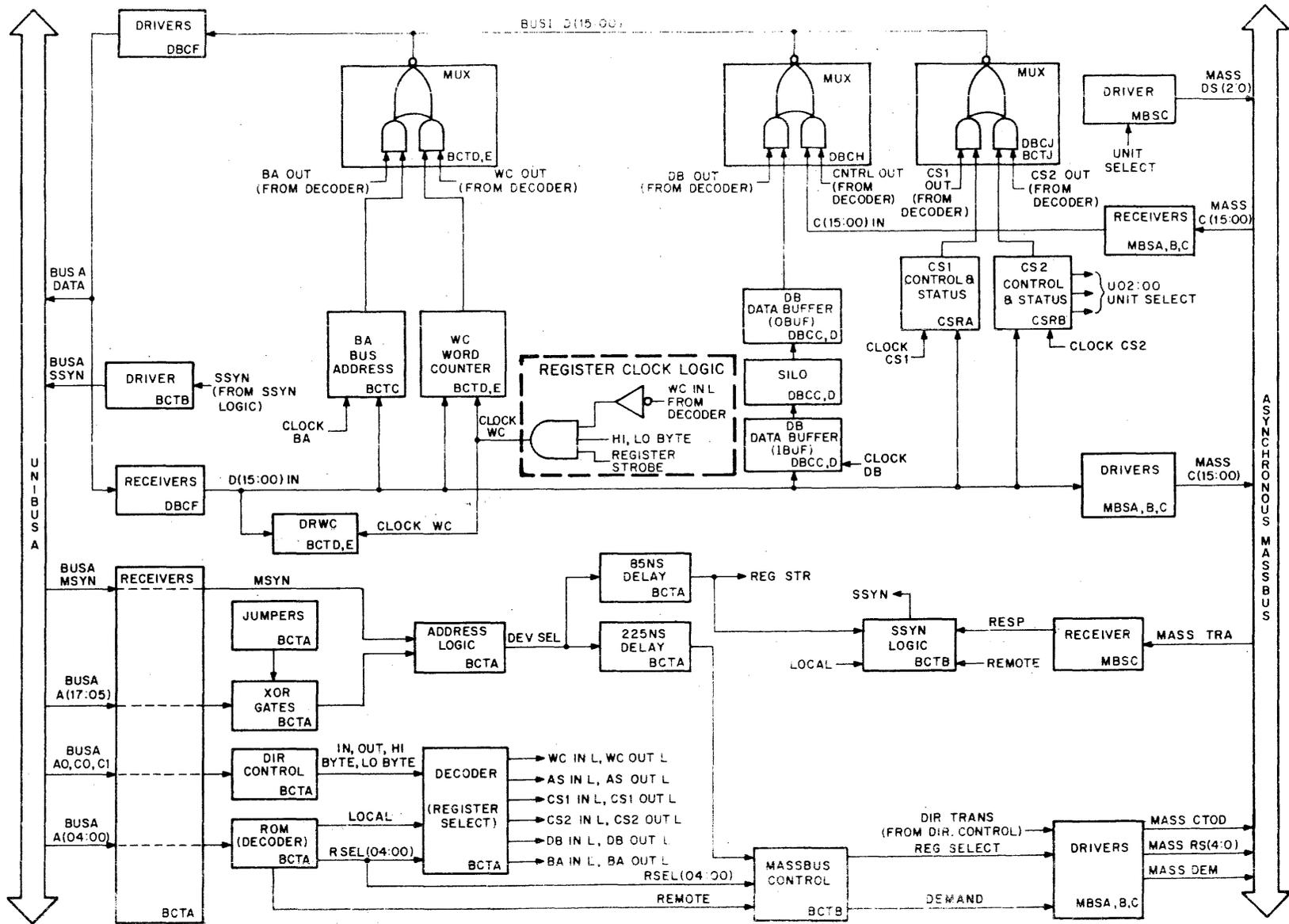
Figure 5-1 Register Control Path
