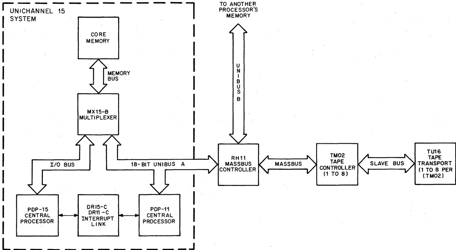
Figure 1-4 RH11 Combined with Unichannel 15 System
