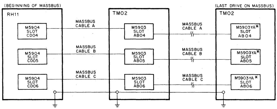
\*M5903YA terminating modules may be replaced by M5903 modules with H870 terminator cards which plug into the modules.
