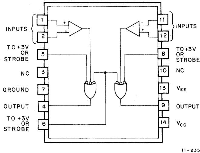
Figure 6-11 75107B Differential Receiver Pin Connection Diagram
