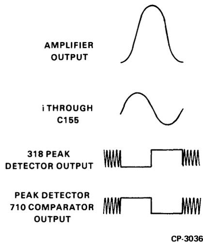
Figure 5-21 Peak Detector Waveforms
