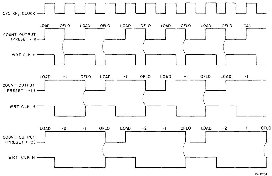
Figure 5-25 WRT CLK Generation Timing
