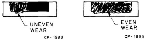
**B. Unacceptable Erase Head Assembly Wear**
