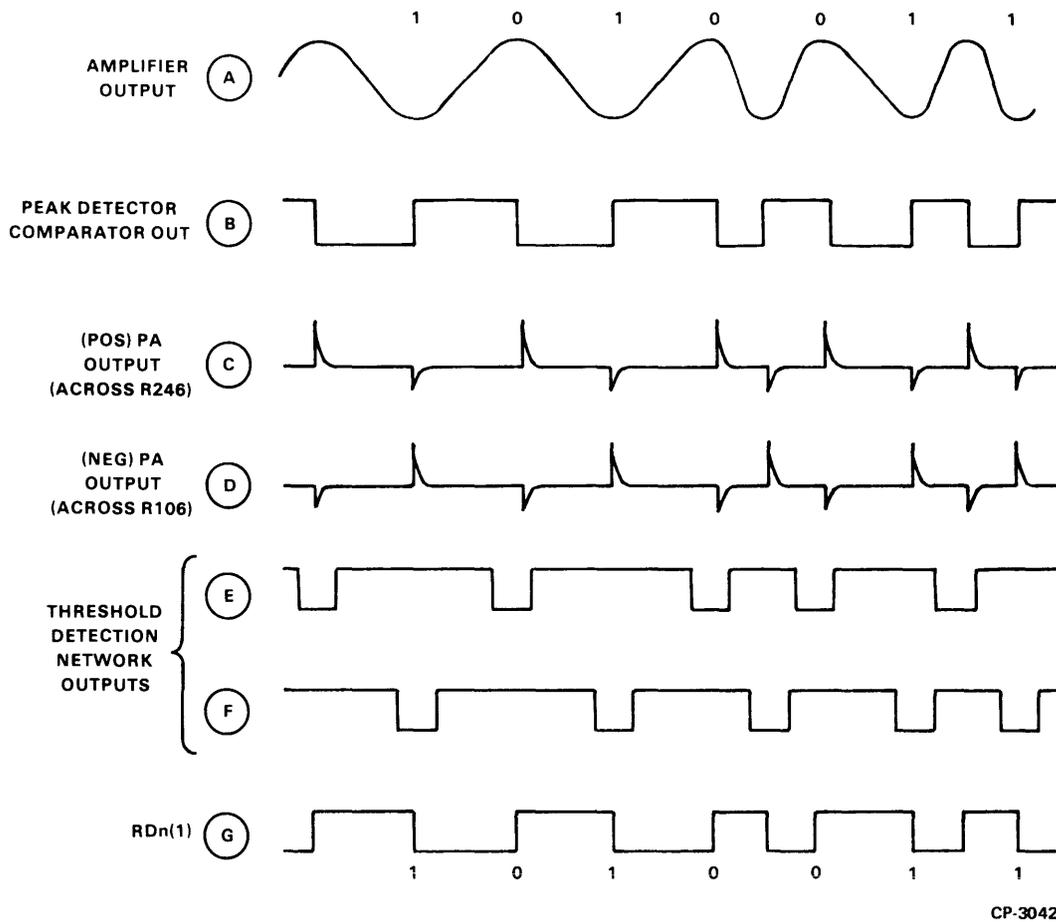
Figure 5-24 Read Amplifier Waveforms (PE)
