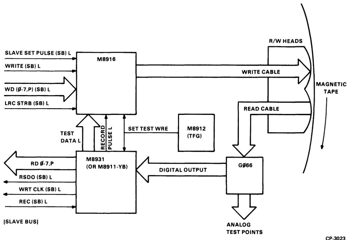
Figure 5-5 Read/Write Functional Block Diagram
