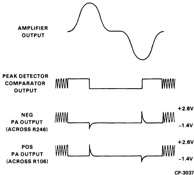
Figure 5-22 POS and NEG Waveforms
