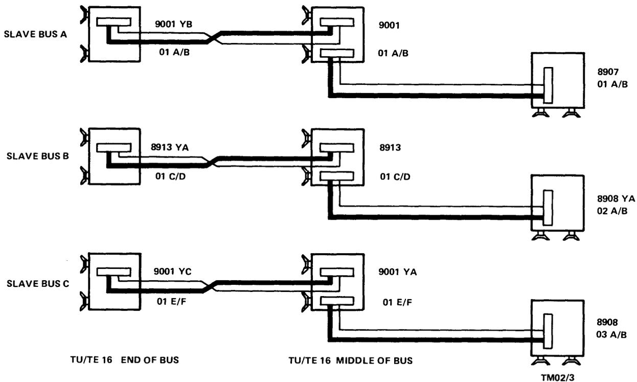
Figure 2-15 Overview of System Cabling
