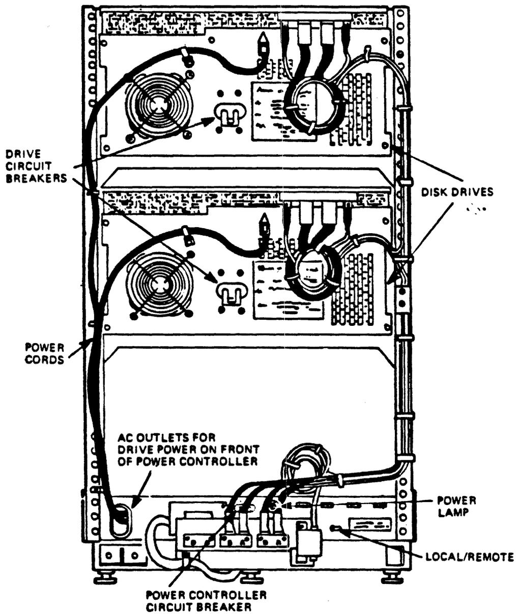
Figure 2 BACK OF AN RA81 DRIVE
