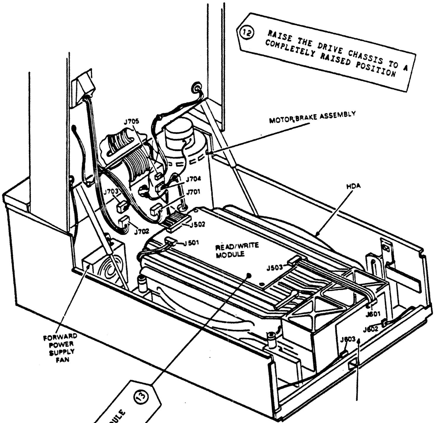
12 RAISE THE DRIVE CHASSIS TO A COMPLETELY RAISED POSITION
