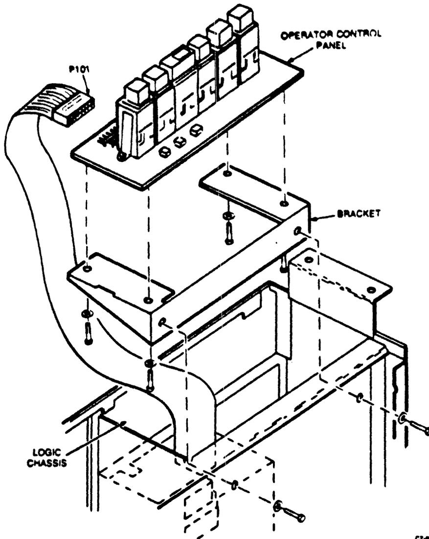
OPERATOR CONTROL PANEL REMOVAL FIGURE 11
