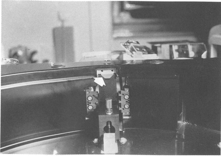
Fig. 1-27 Make sure that rail touches rail bracket
