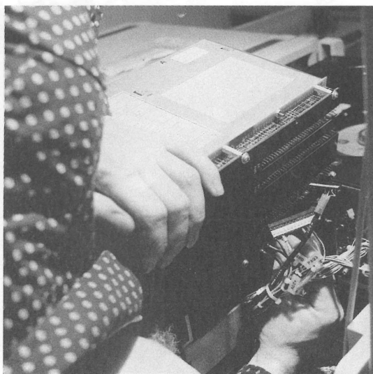
Fig. 1-6 Remove all the cables from logic chassis and remove chassis (Fig. 1-6/1-7/1-8).
