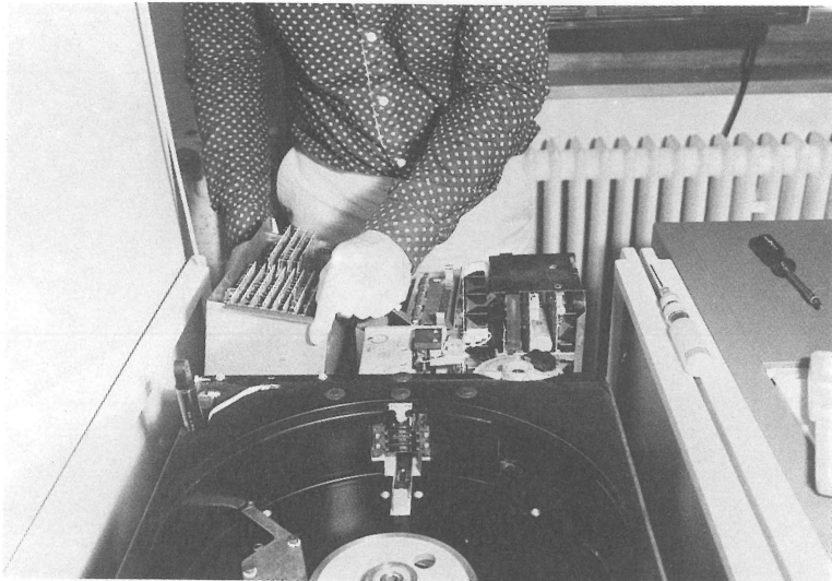
Fig. 1-5 Lift the logic chassis assembly to the maintenance position.
