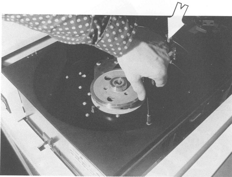
Fig. 1-19 If you have to replace the lower carriage rail (Fig. 1-18) lift the drive deck by removing the two screws in the shroud (Fig. 1-19)
