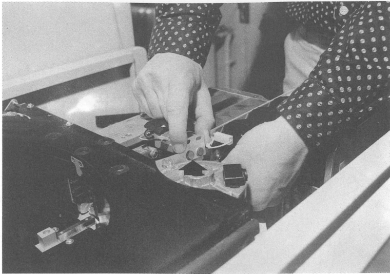
Fig. 1-11 Remove upper carriage stop. Remove head assemblies and flex lead assembly.
