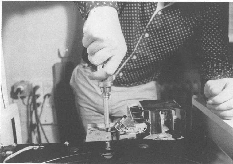
Fig. 1-28 Torque upper rail screws to 10 \pm 2 in. lbs. Remove rail alignment tool and reinstall the remaining two screws of the lower carriage rail.
