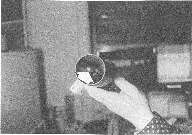
Fig. 1-29 Change tachometer rod from old carriage assembly to the new one. The tachometer rod has to be centered.
