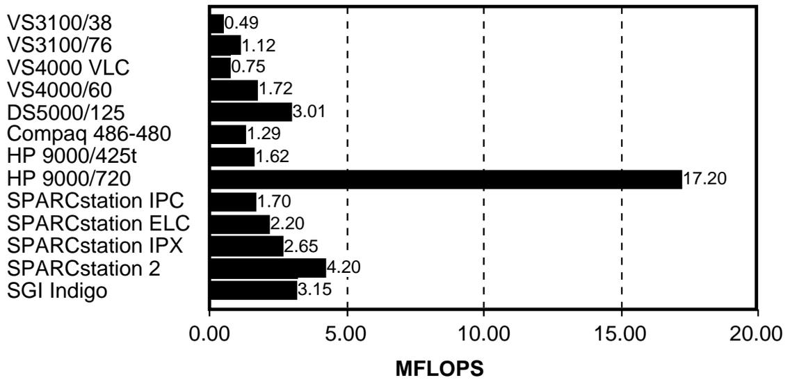
**Figure 4-12: Linpack Double Precision MFLOPS Ratings**
