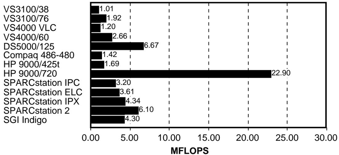
Figure 4-11: Linpack Single Precision MFLOPS Ratings
