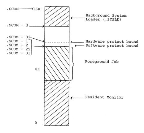
When a BACKGROUND keyboard command requests loading of a system or user program, the Non-resident Monitor brings in the System Loader, overlaying itself. Note that the BACKGROUND System Loader and the FOREGROUND Linking Loader are physically the same program, except that SYSBLK is also read into core when the BACKGROUND system program to be loaded is other than the Linking Loader or Execute.
