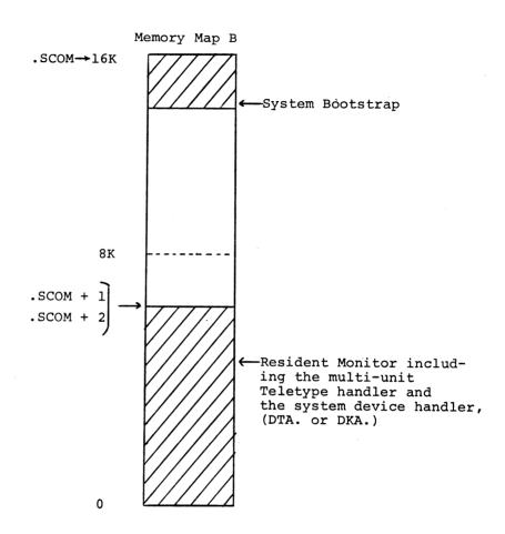
The System Bootstrap automatically loads the Resident Monitor from the system device into lower core.
