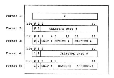
Formats 1 through 3 are the <u>pre-setup</u> stage (I/O handler linkage not established); Formats 4 and 5 are <u>setup</u> (I/O handler linkage established, handler is in core and I/O calls to such .DAT slots will be honored by the Monitor). Bit  $\emptyset$  distinguishes Formats 1 through 3 from 4 and 5.
