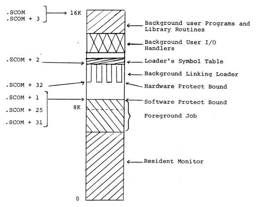
The BACKGROUND Linking Loader overlays the System Loader by loading user programs down from the top of core. User I/O handlers, presuming that they cannot fit in core between the FOREGROUND job and the bottom of the Loader, are loaded into upper core but relocated to run just above the FOREGROUND job so that the memory protect bound can be set above them. Common blocks and I/O buffers are not shown in this memory map.
