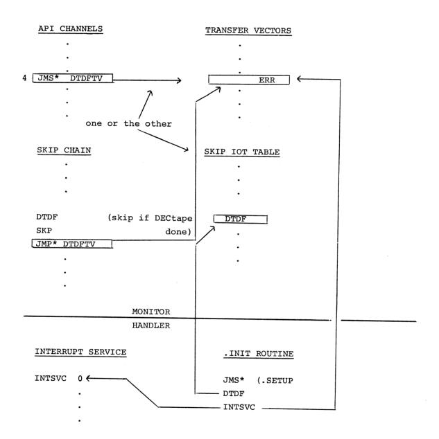
FIGURE 8-1 INTERRUPT LINKAGES FOR I/O DEVICES
