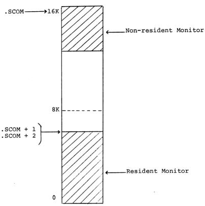
The Resident Monitor loads the Non-resident Monitor (via the resident system device handler) into upper core, overlaying the System Bootstrap. Within itself the Resident Monitor contains a simpler copy of the bootstrap which is used whenever the Resident Monitor is to be reloaded. The bootstrap restart address is location 1118.
