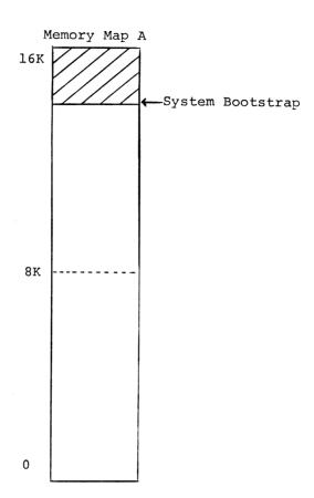
The System Bootstrap is loaded at the top of core via the paper tape reader in HRM format.
