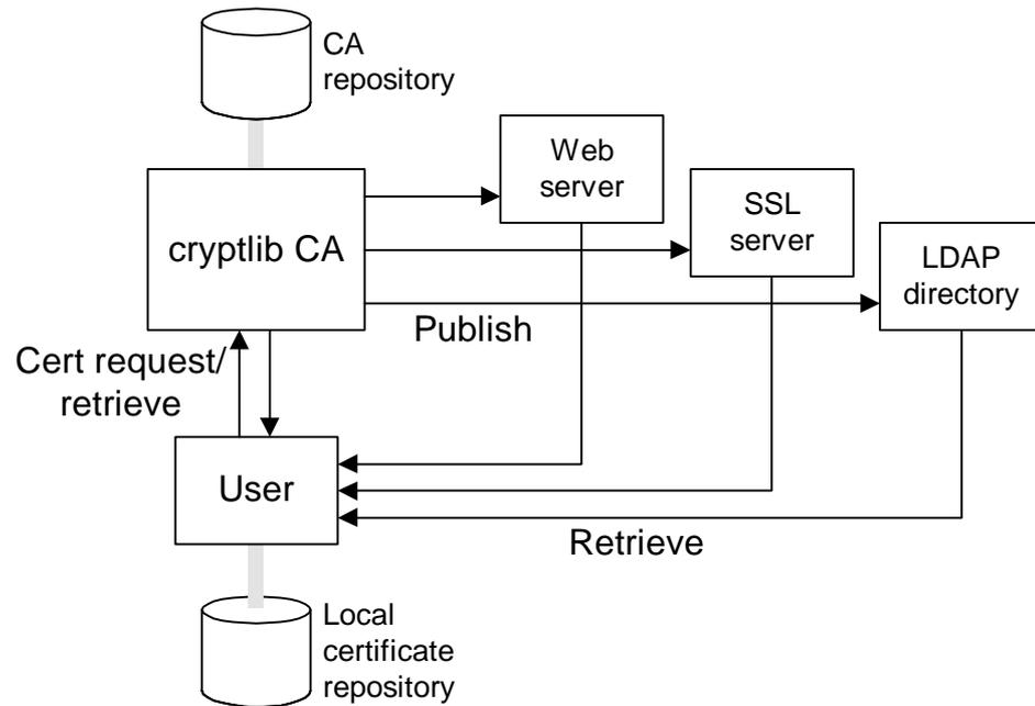
To handle certificate trust and revocation issues, cryptlib includes a certificate trust manager that can be used to automatically manage CA trust settings. For example a CA can be designated as a trusted issuer that will allow cryptlib to automatically evaluate trust along certificate chains. Similarly, cryptlib can automatically check certificates against RTCS and OCSP responders and CRLs published by CAs, removing from the user the need to perform complex manual checking.
