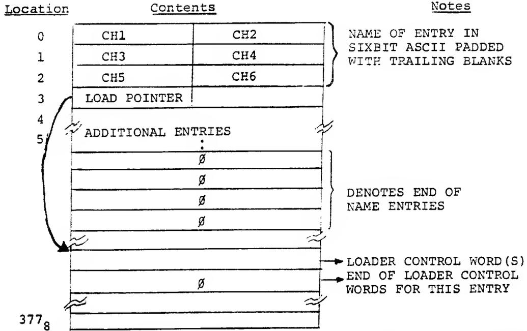
The Load Pointer is a number between 0 and 377 (octal) which points (relative to the beginning of the block) to an array of Loader Control Words. The Loader Control Words have the following information:
