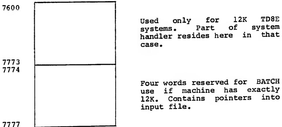
If the machine has more than 12K, the top 4 location (7774-7777) of the last field are reserved for use by BATCH.
