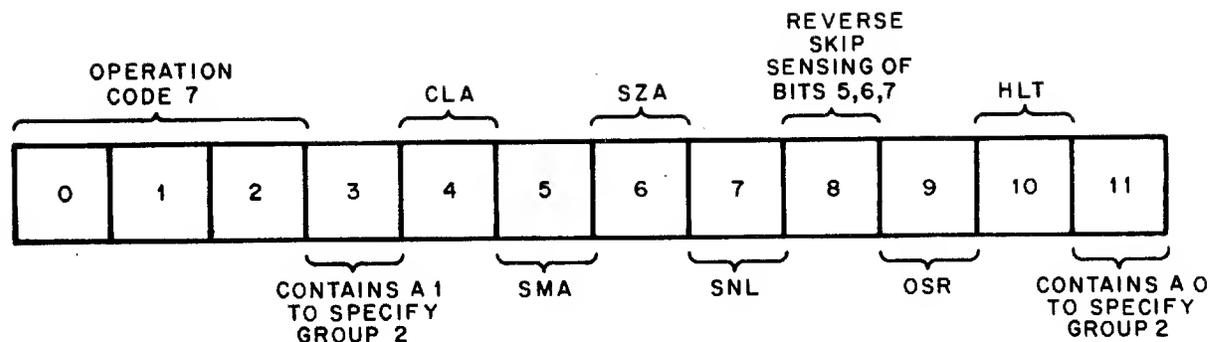
Figure 4-5 Group 2 Operate Instruction Bit Assignments
