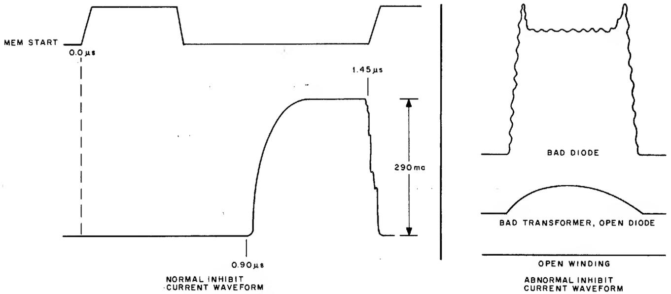
Figure 5-5 Representative Inhibit Current Waveforms
