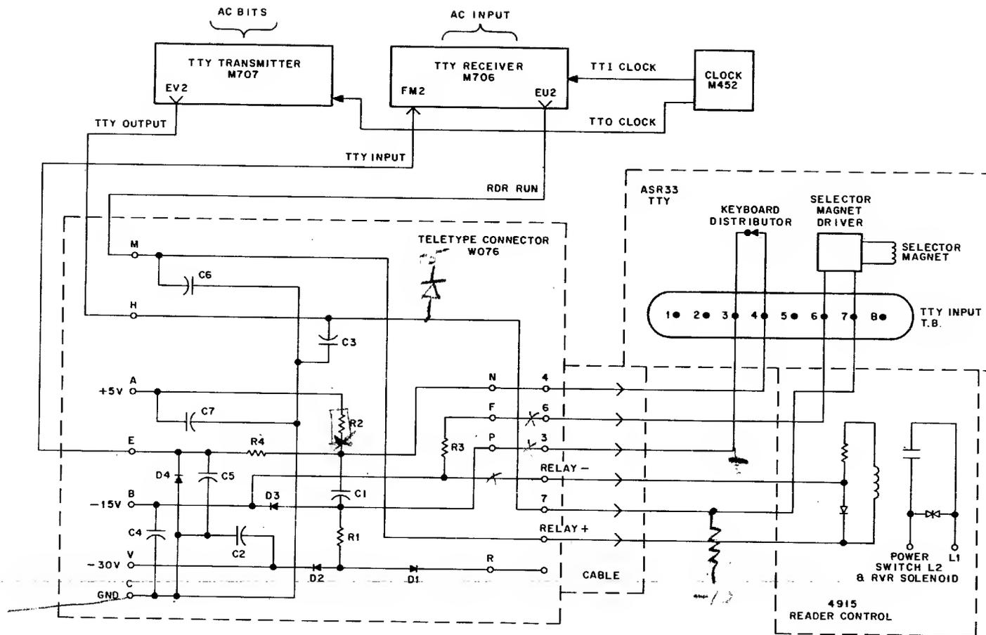
Figure 5-7 Teletype Connections
