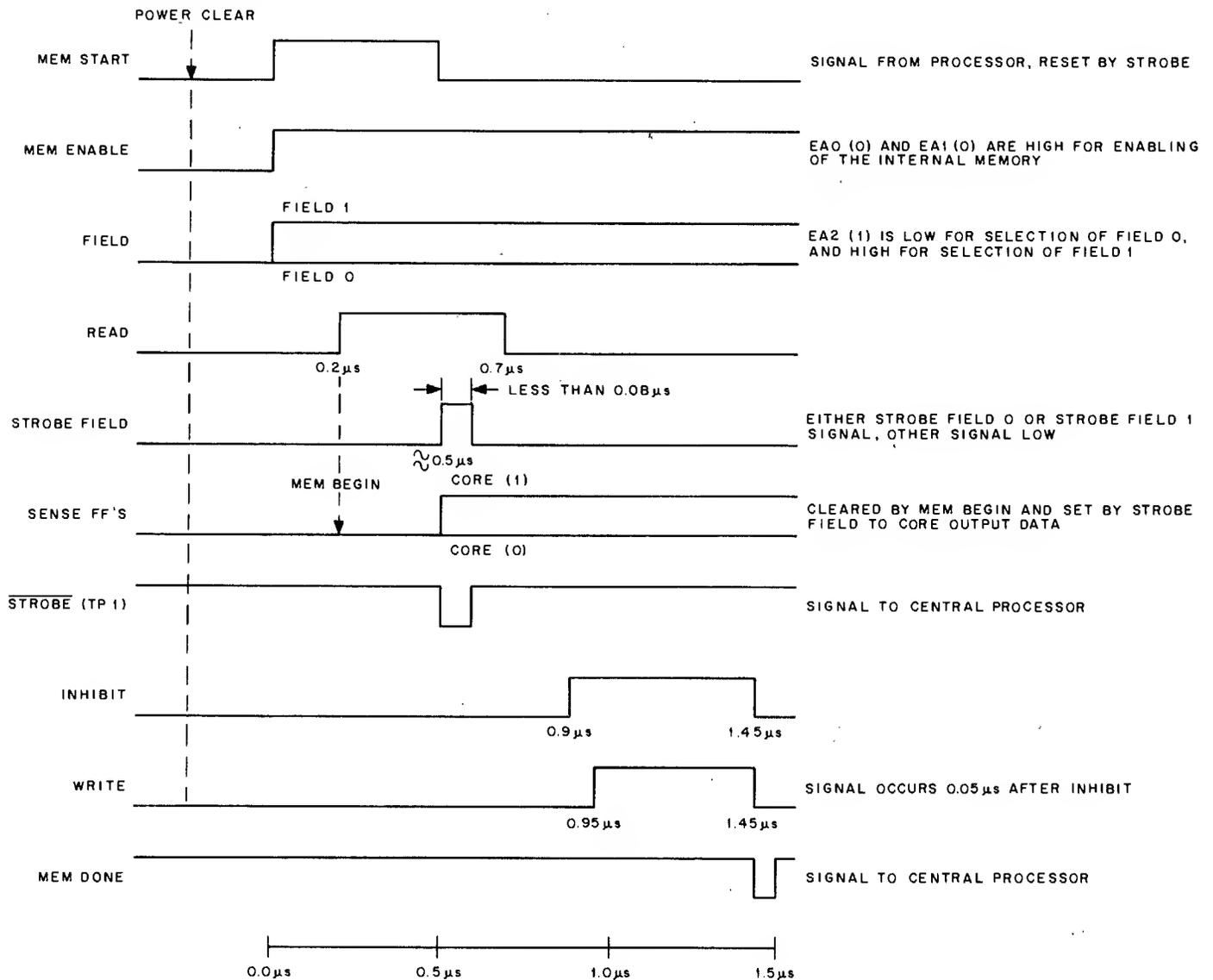
NOTE: TRANSITION TIMES ARE MEASURED FROM THE POSITIVE TRANSITION OF MEM START AND ARE APPROXIMATE.
