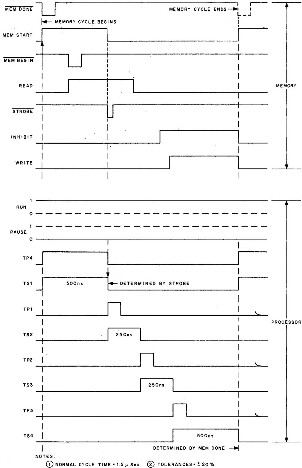
Figure 4-11 System Timing Diagram
