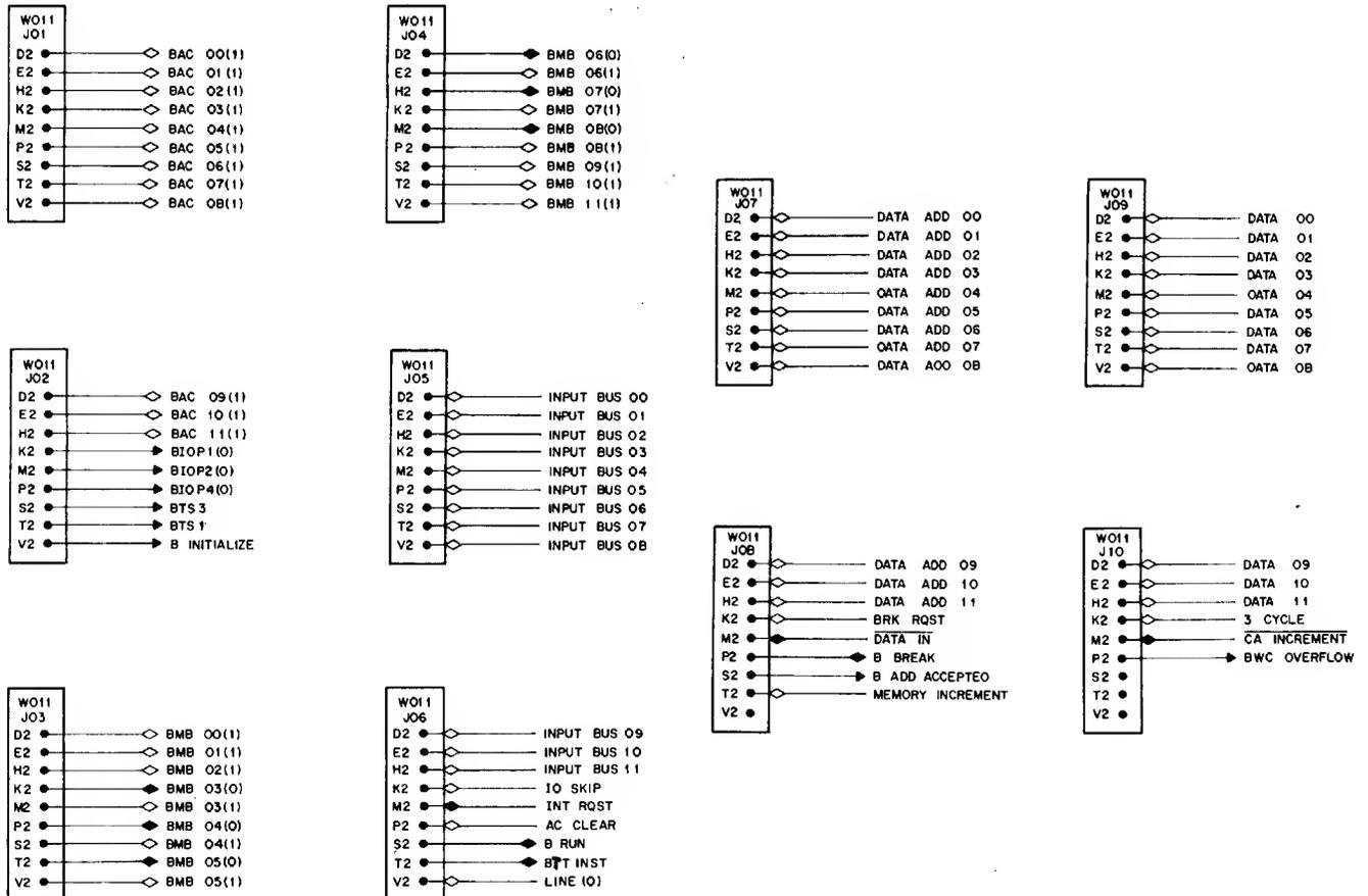
Figure 2-8 I/O Signal Connections
