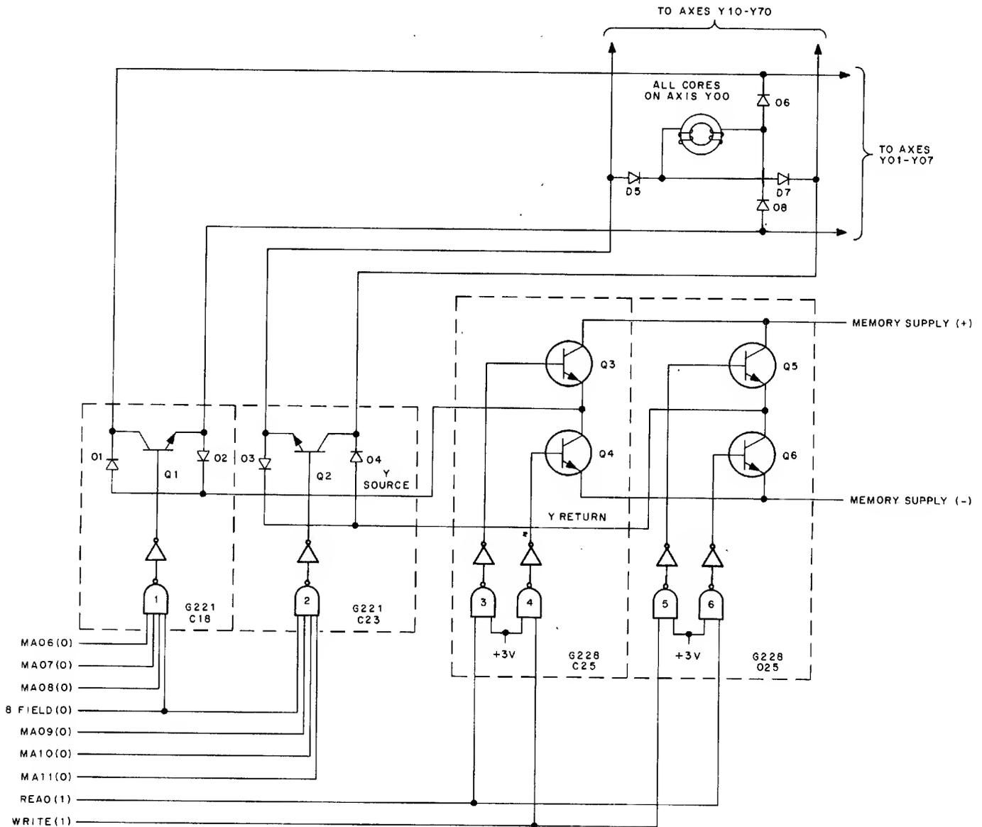
Figure 4-9 Memory Address Selector and Read/Write Current Control
