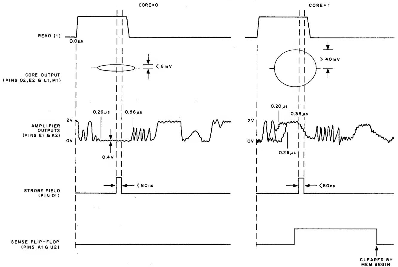
NOTE: CORE OUTPUTS ARE OBSERVED DIFFERENTIALLY AT THE PINS NOTED.
