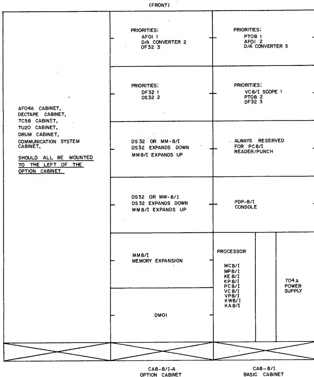
Figure 2-6 System Configurations
