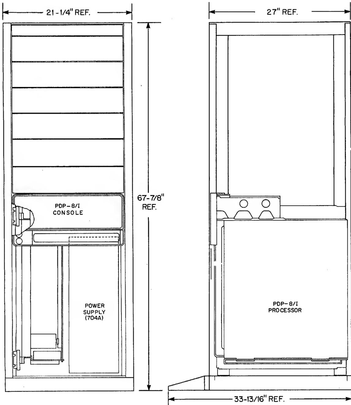
Figure 2-3 PDP-8/I Installation in Standard DEC Cabinet
