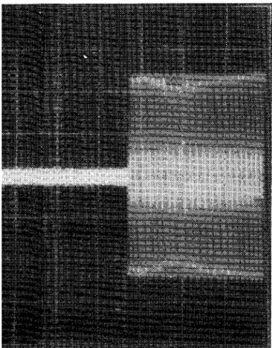
d. Head correctly aligned. Amplitudes are equal.
