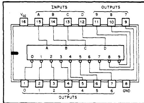
Figure A-1 7442 Package and Logic Diagrams
