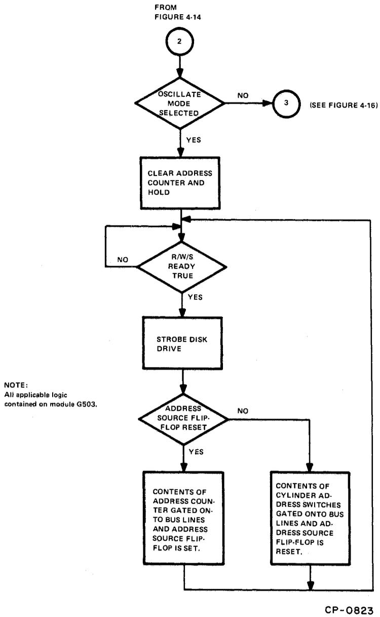
Figure 4-15 Positioner Exerciser Oscillate Mode Flow Diagram
