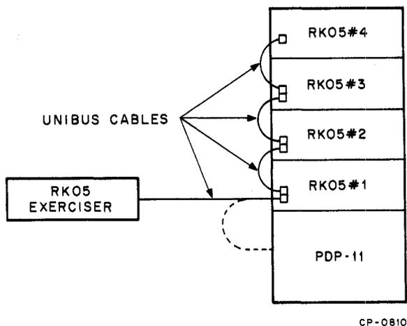
Figure 2-2 RK05 Exerciser to Multiple RK05 Disk Drives Connection Diagram
