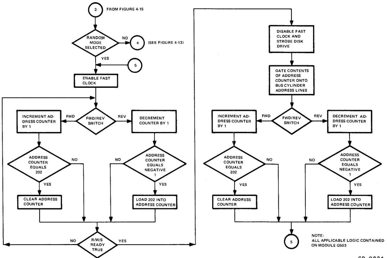
Figure 4-16 Positioner Exerciser Random Mode Flow Diagram
