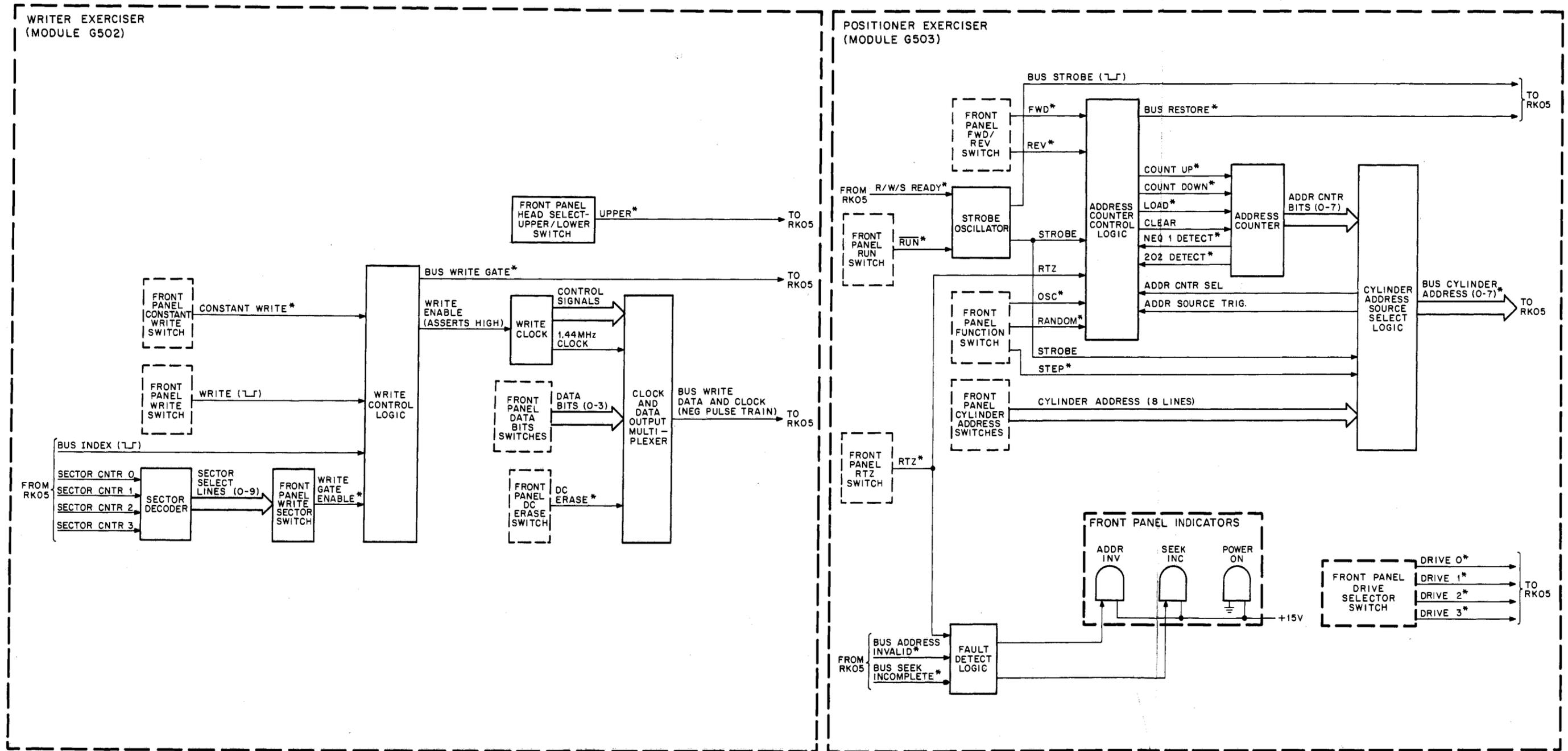
Figure 4-1 RK05 Exerciser Functional Block Diagram
