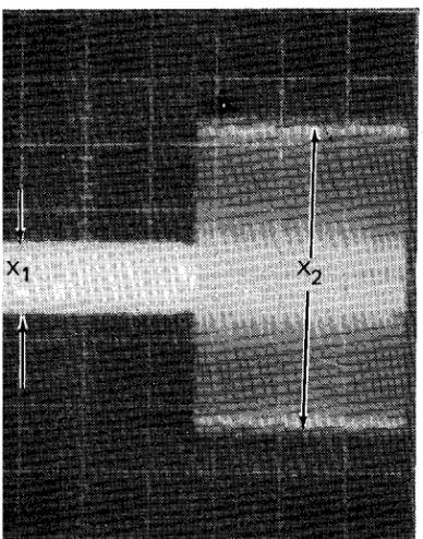
e. Heads slightly misaligned. Larger left amplitude indicates head inside of CYL 105 (toward 106).
