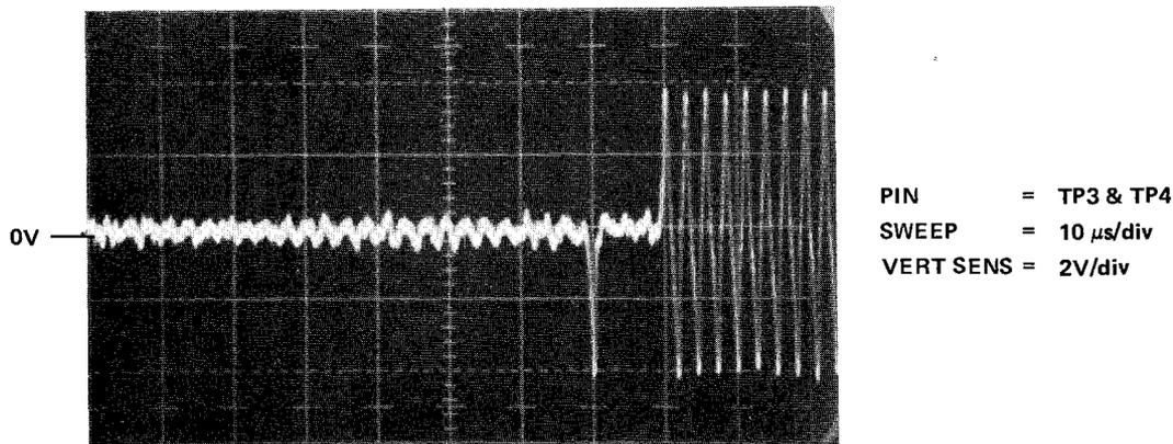
Figure 6-13 Index/Sector Waveform
