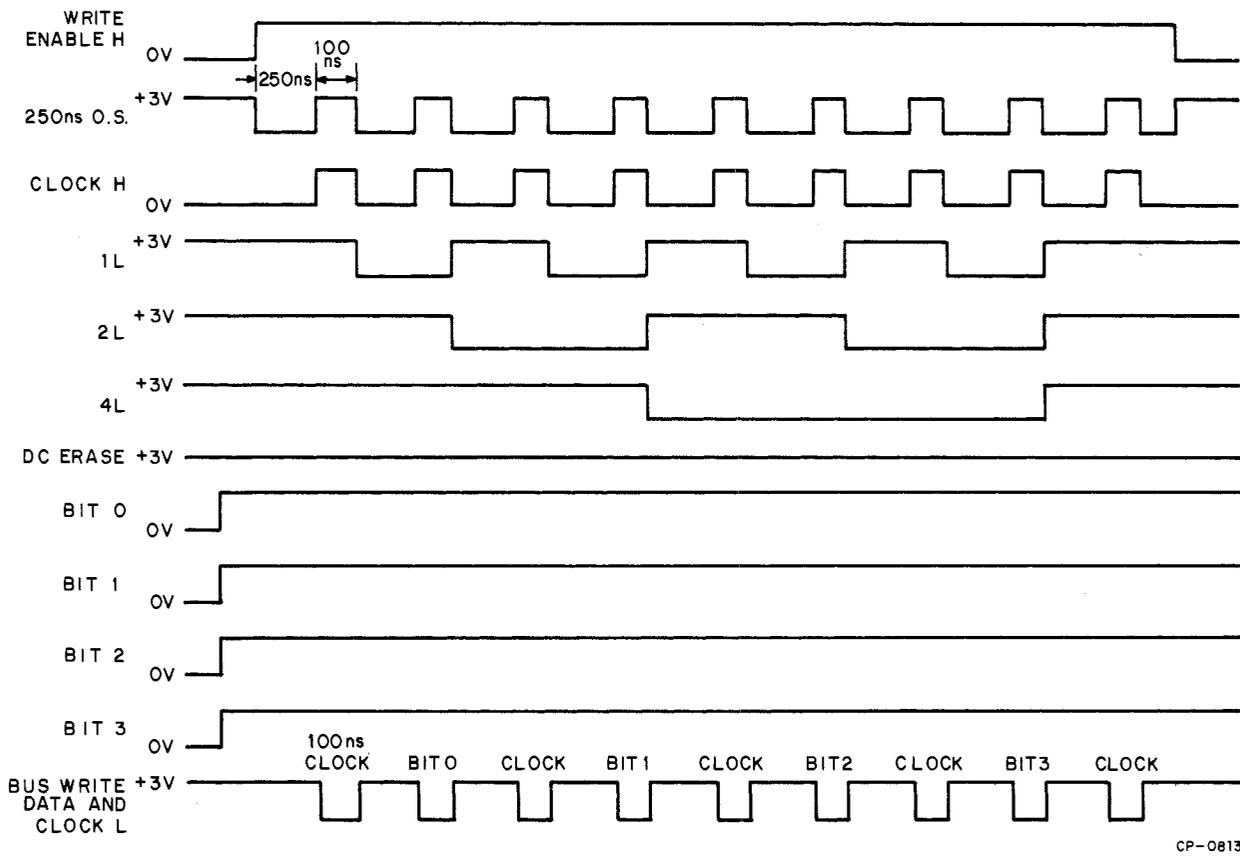
Figure 4-5 Write Clock and Multiplexer Timing Diagram
