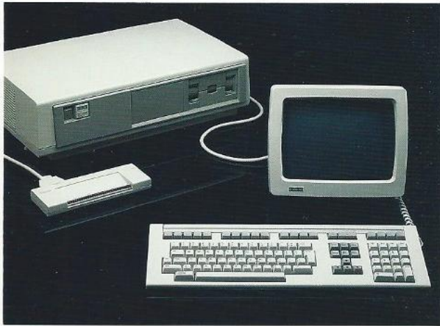
The Professional 350 with the RTI Connector Pod enables the researcher to use more than one I/O interface.
