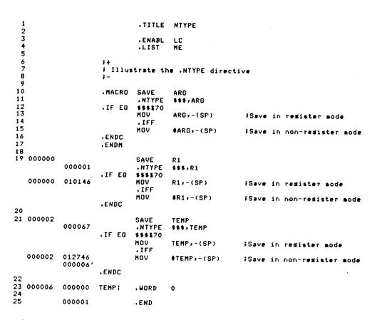
Figure 7-3 Example of .NTYPE Directive in Macro Definition
