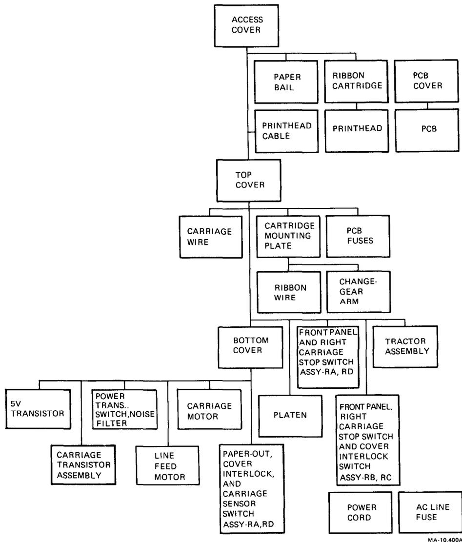
Figure 6-1 Assembly Removal Sequence
