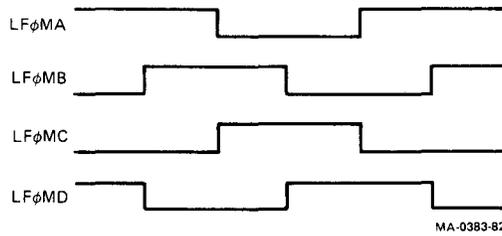
Figure 4-8 Line Feed Motor Phase Patterns
