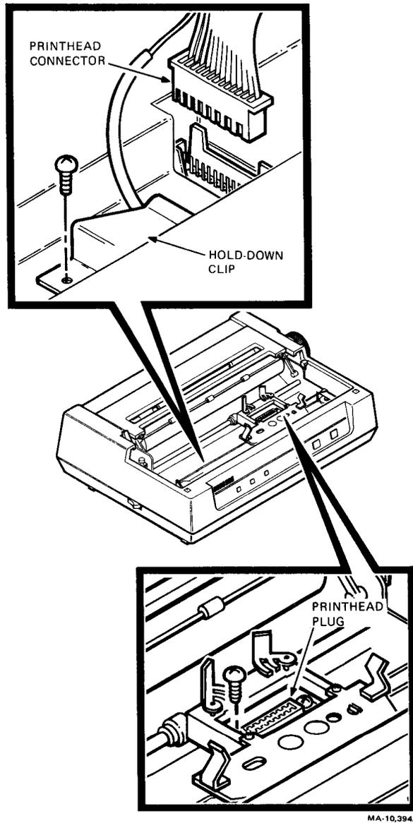
Figure 6-14 Printhead Cable
