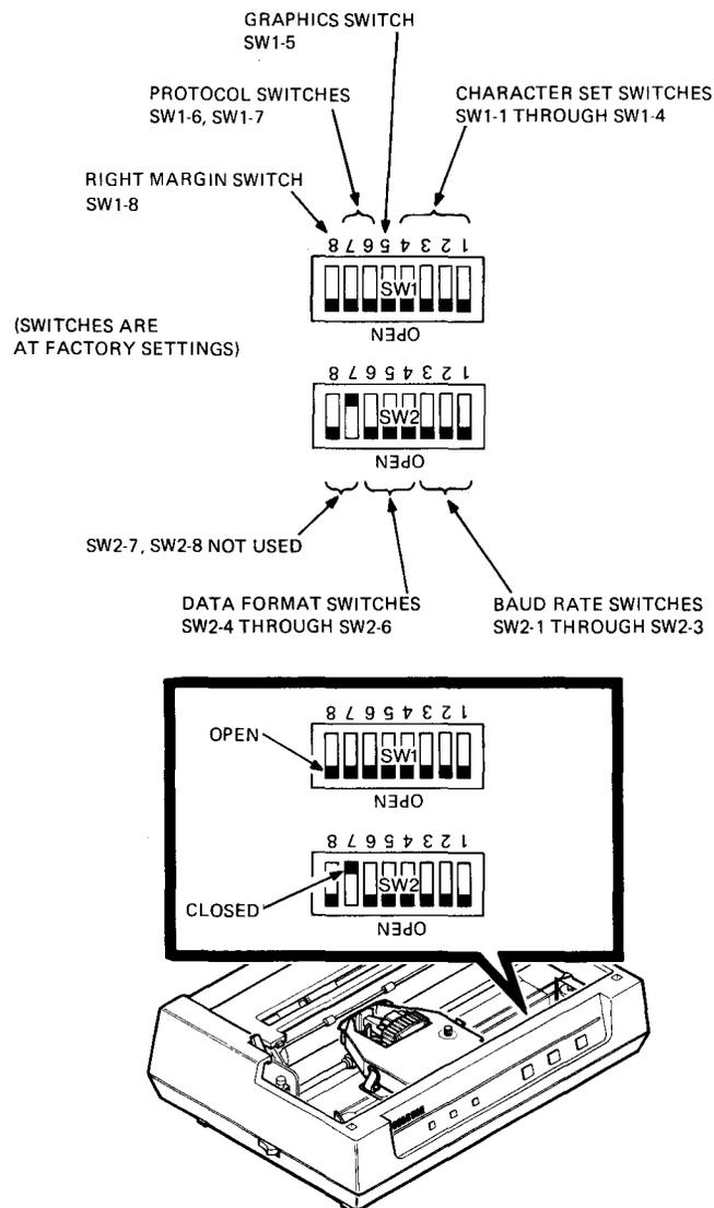
Figure 2-9 Configuration Switches
