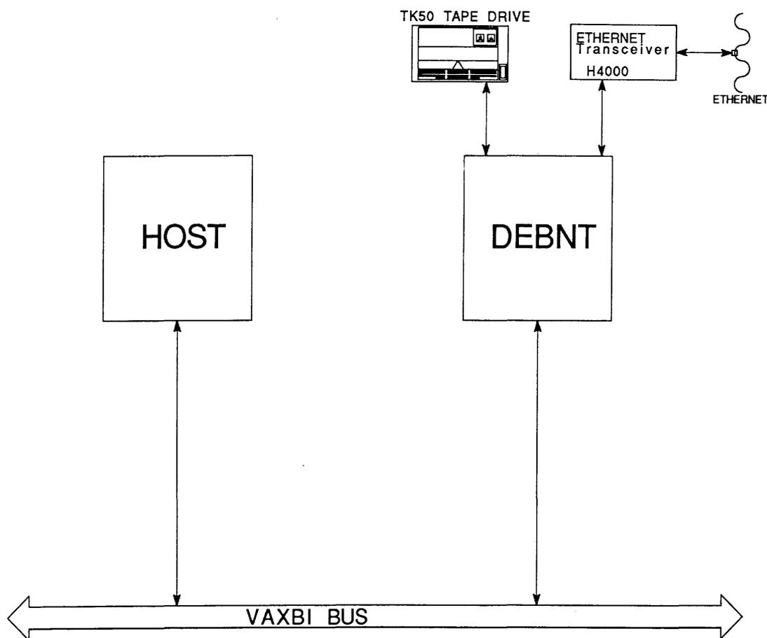
Figure 3-1 The DEBNT in a VAXBI System
