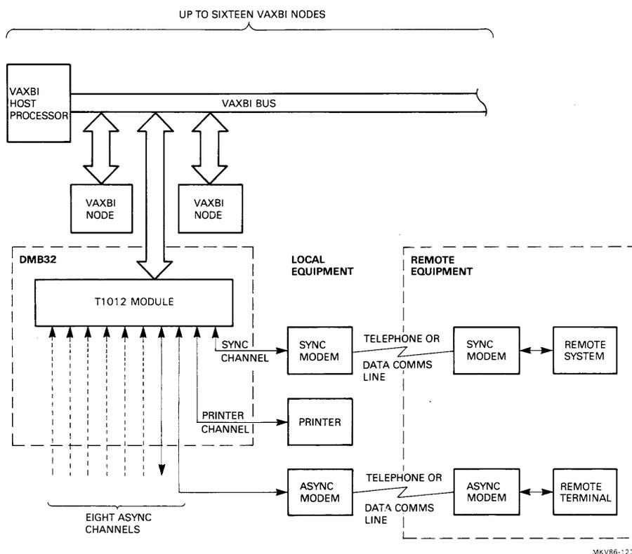
Figure 2-1 Typical DMB32 Configuration
