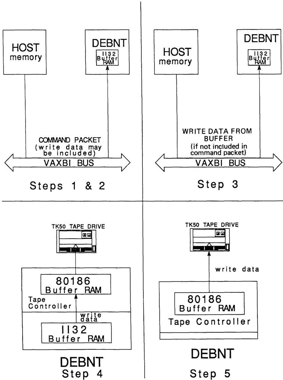
Figure 3-6 Tape Write Transaction (Sheet 1 of 2)
