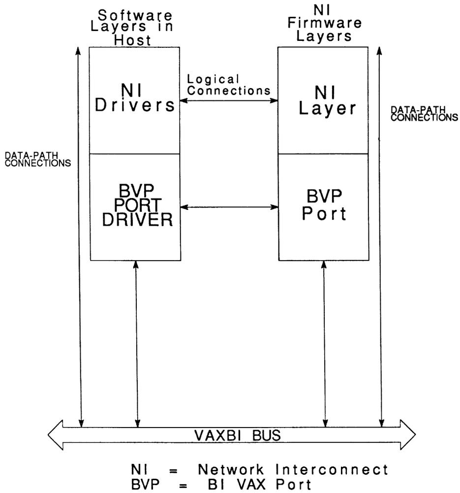
Figure 3-7 NI Firmware and Corresponding Software Layers in Host
