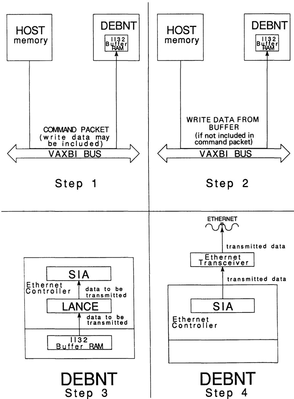
Figure 3-3 Ethernet Transmission
