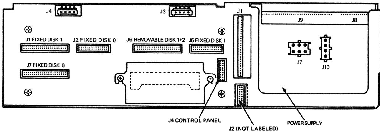
**Figure 3-12: BA23-A Internal Cabling**
