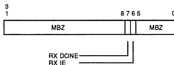
Figure 6-1 Console Receiver Control/Status Register - (IPR 32<sub>10</sub> 20<sub>16</sub>)
