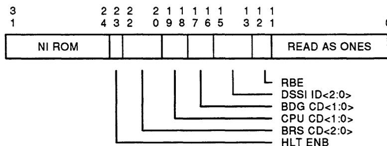
Figure 8-1 Boot and Diagnostic Register
