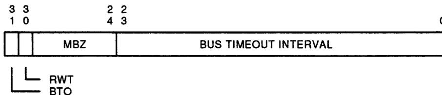
Figure 8-7 CP Bus Timeout Control Register (CBTCR)
