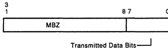
**Figure 6-4 Console Transmitter Data Buffer - (IPR 35<sub>10</sub> 23<sub>16</sub>)**
