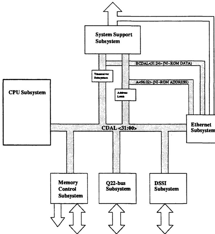
**Figure 1-4 KA660 Processor Module Major Functional Blocks**
