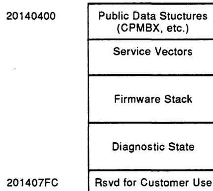
Figure H-1 KA660 SSC BBU RAM Layout
