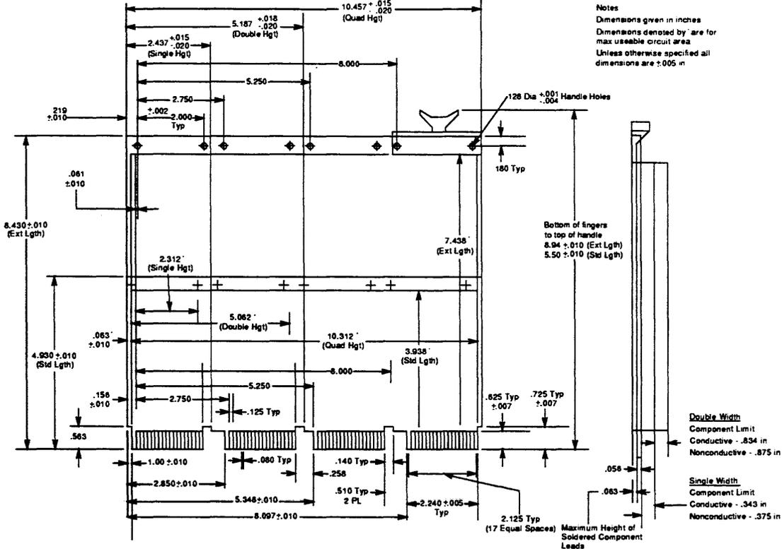
Figure A-20 Typical Q22-bus Module Dimensions
