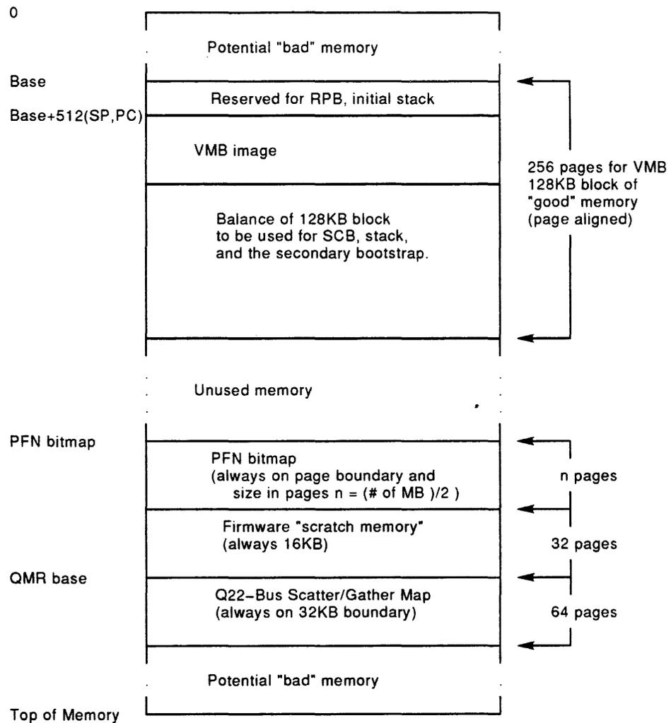
**Figure 12-8 Memory Layout Prior to VMB Entry**
