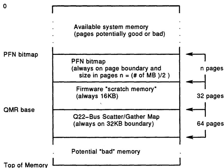
Figure E-1 Memory Layout after Power-up Diagnostics
