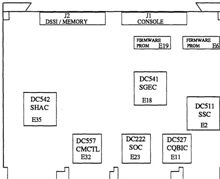
**Figure 1-3 KA660 CPU Module Component Side**
