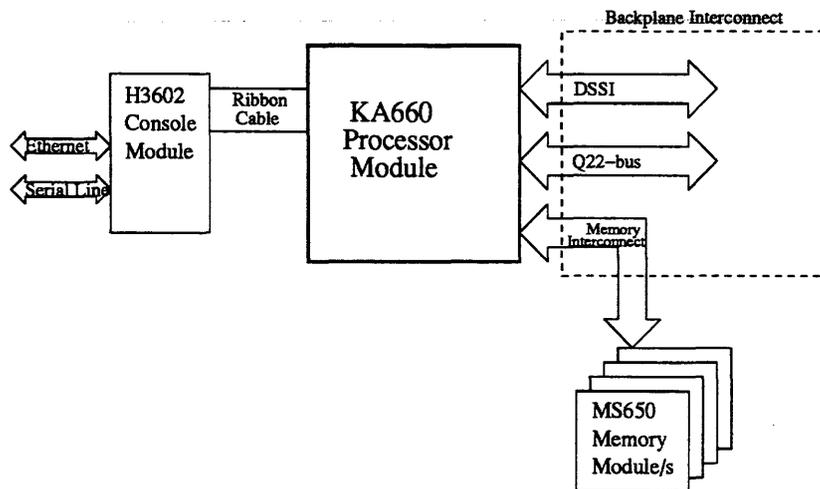
Figure 1-1 KA660 Module in a System
