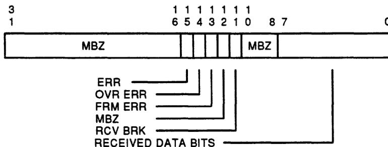
**Figure 6-2 Console Receiver Data Buffer - (IPR 33<sub>10</sub> 21<sub>16</sub>)****Table 6-3 Console Receiver Data Buffer**
