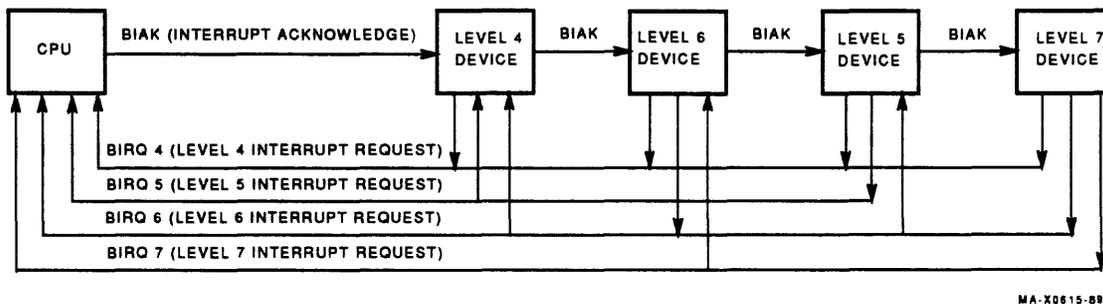
Figure A-13 Position-Independent Configuration
