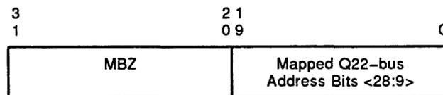
**Figure 9-9 DMA Error Address Register (DBEAR)**
