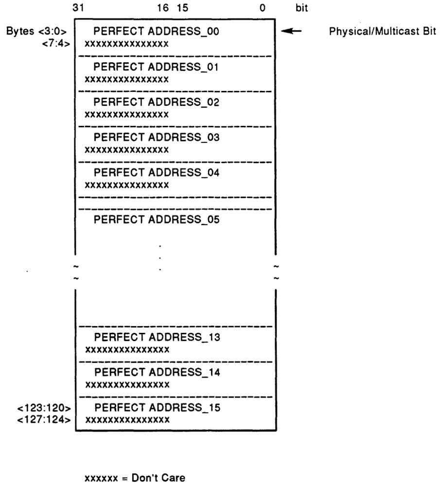
**Figure 10-17 Perfect Filtering Setup Frame Buffer format**
