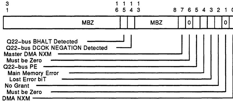
Figure 9-7 DMA System Error Register (DSER)
