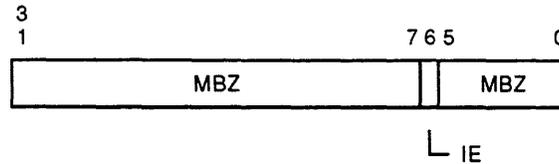
Figure 7-2 Interval Timer (ICCS) - (EPR 24<sub>10</sub> 18<sub>16</sub>)
