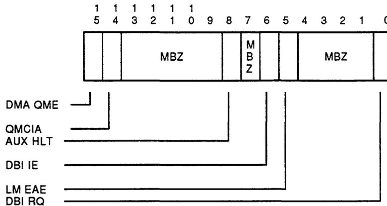
Figure 9-4 Interprocessor Communication Register (IPCR)
