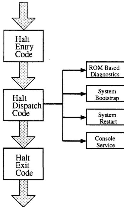
**Figure 12-1 KA660 Firmware Structural Components**
