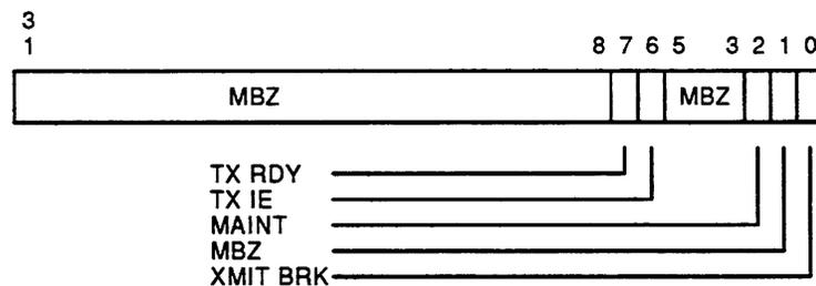
**Figure 6-3 Console Transmitter Control/Status Register - (IPR 34<sub>10</sub> 22<sub>16</sub>)**
