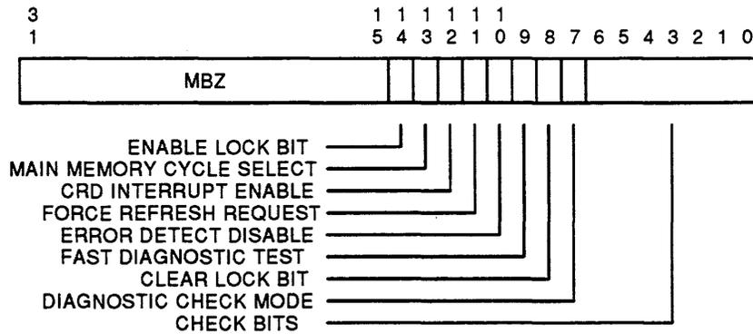
Figure 5-1 Main Memory Control and Diagnostic Status Register (MEMCSR17)
