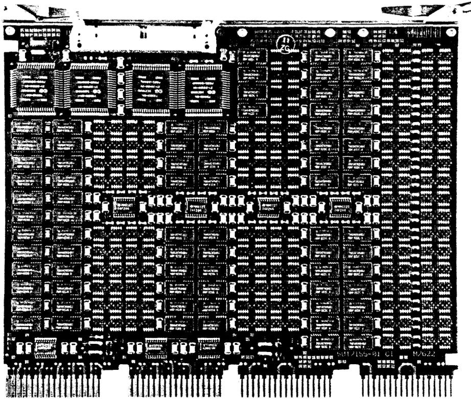
**Figure 1-6 MS650 Memory Module (8 MB)**
