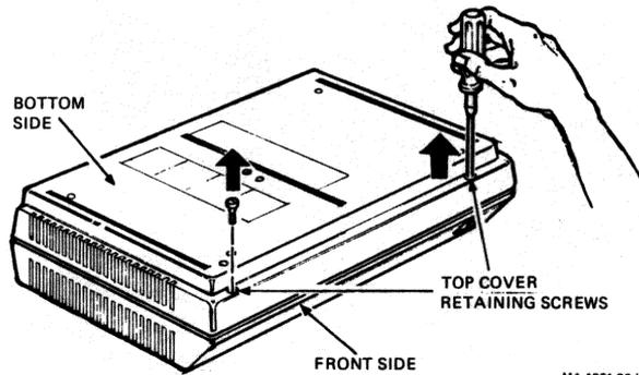
4. Reposition the system box as shown below. Lift the cover up from the front and pull forward to release the hinge hooks.
