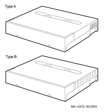
The type A cartridge shell has a smooth surface on the side, while type B has a slotted design. The type B cartridge was designed to provide a better grip surface. While a good ergonomic design for manually loading and unloading a DDS tape drive, the type B does not perform as reliably in the TLZ6L Autoloader as the type A. Because of the growing application of autoloaders, some manufactures will be phasing out the type B design.
