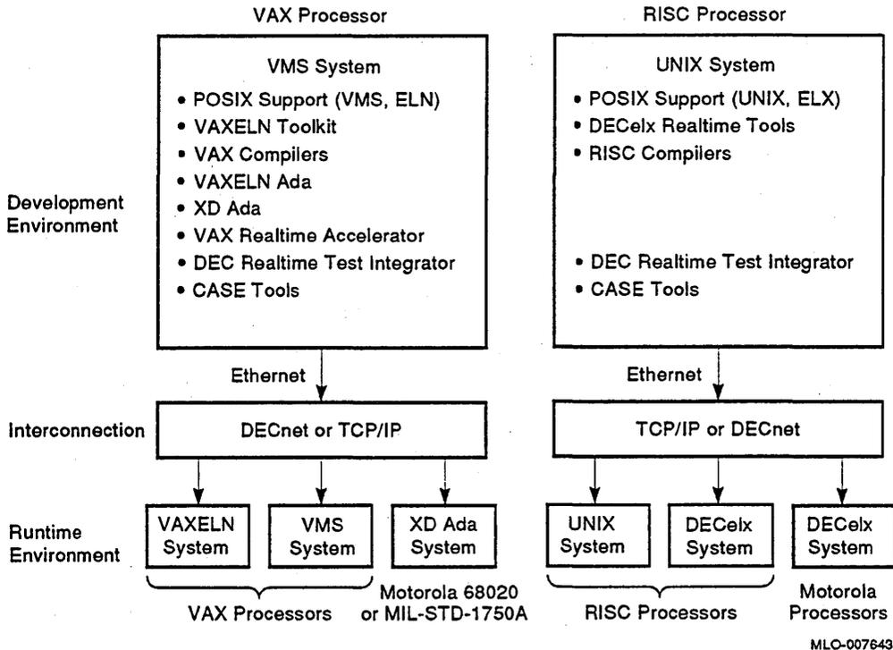
Figure 1-1 shows DEC Realtime Integrator graphical programming tools, UNIX CASE tools, and high-level language compilers also available for an ULTRIX on a MIPS-based system. As with OpenVMS on a VAX and VAXELN systems, your UNIX system can communicate with the rest of your enterprise using DECnet or TCP/IP networking software.
