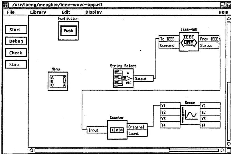
**Figure 22-3 IOtech WAVE488 Application Signal Flow View**
