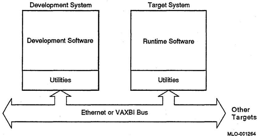
You develop a VAXELN application on a VMS development system by using a comprehensive set of VMS CASE and VAXELN development tools. The resulting VAXELN system image contains user and toolkit program images, and can be booted on the VAX target system from disk, tape, or read-only memory (ROM). If you have a DECnet-VAX license and the appropriate Ethernet hardware, you can down-line load the system image from a VMS, ULTRIX, or VAXELN system (serving as boot host) to the target processors.
