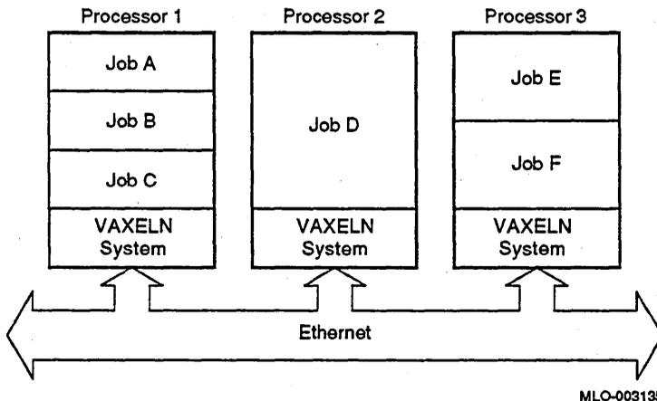
**Figure 5-3 Tightly Coupled Symmetric Multiprocessing Configuration**
