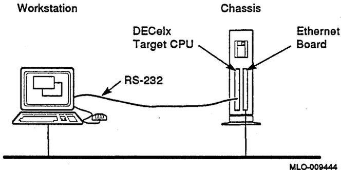
DECElX supports network communications between an ULTRIX host system and target systems connected to a common VME backplane. The ULTRIX backplane driver uses the TURBOchannel/VME adapter and provides a BSD socket interface between ULTRIX processes on MIPS-based DECstations and DECElX tasks running on the VMEbus.
