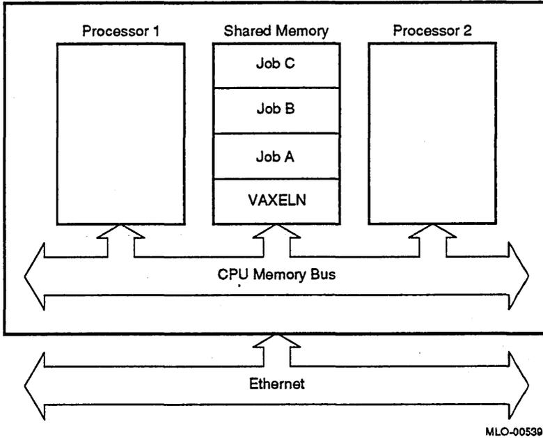
In a tightly coupled configuration, VAXELN supports multiple symmetric processors on the same processor bus, as shown in Figure 5-3.
