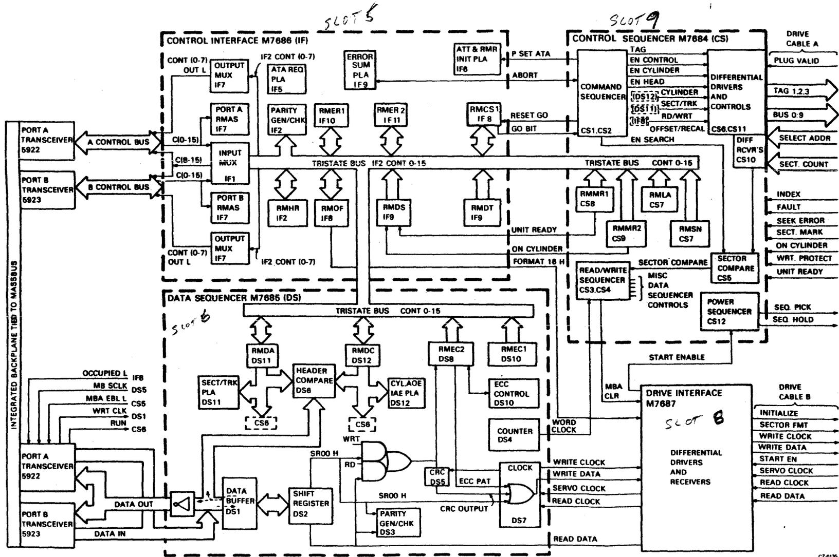
Figure 3-10 RM Adapter Block Diagram
