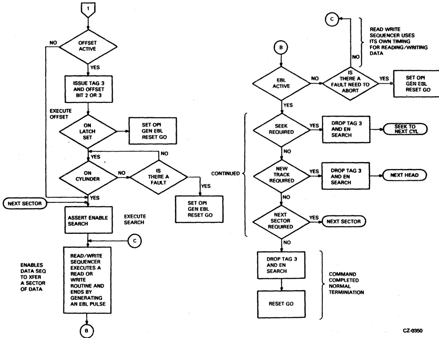
Figure 3-19 Data Transfer Command Flowchart (Sheet 2 of 2)
