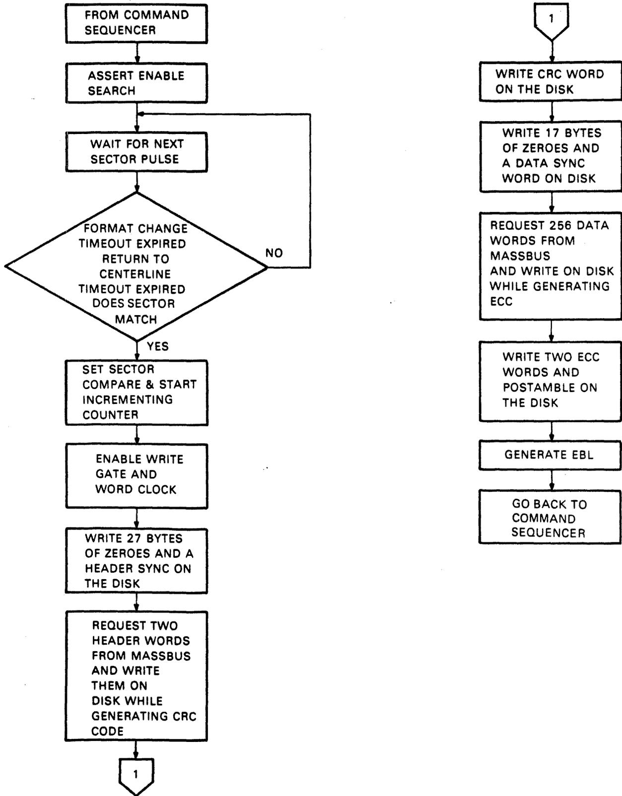
Figure 3-22 Write Header and Data Command Flowchart
