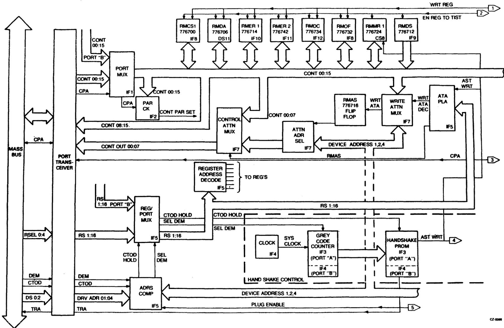
Figure 3-7 Register Read/Write Handshaking Block Diagram (Sheet 1 of 2)
