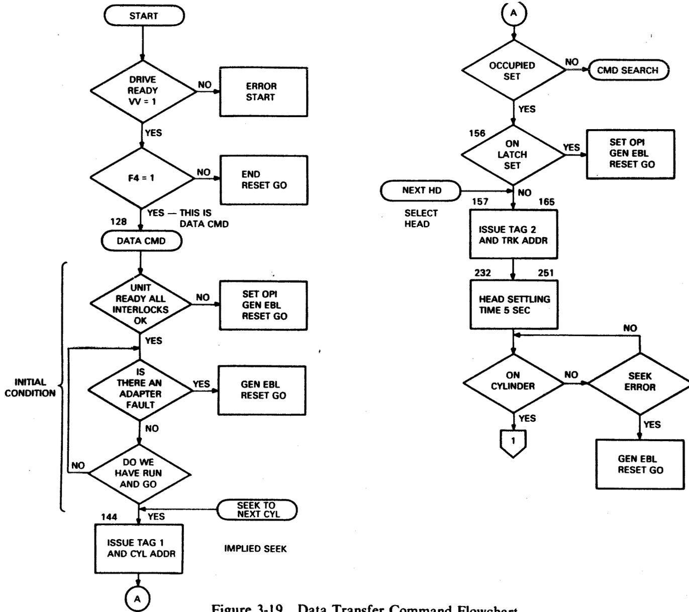
Figure 3-19 Data Transfer Command Flowchart
