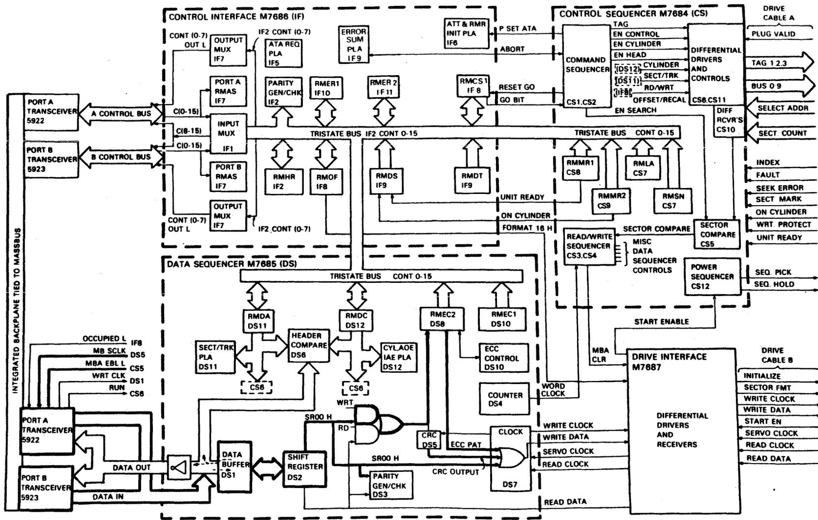
Figure 3-14 - Write Data Flow Path Diagram
