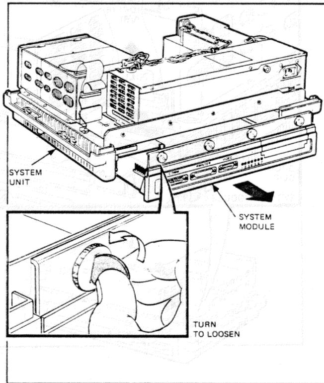
**Step 11.** If you are replacing the system module, remove and save any options that you have so that you can install them on the new system module.
