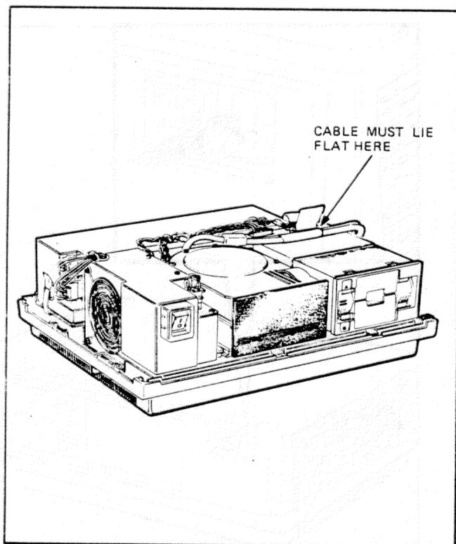
**Step 8.** Place the cover on the system unit. Slide the cover release tabs in and away from you until they spring back, locking the cover. Try lifting the cover to make sure it is secure.
