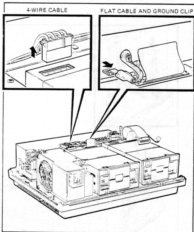
**Step 11.** If you have a hard disk drive, pull the ground clip of the hard disk drive cable off the ground lug on the power supply. Then, press the latch in front of the hard disk drive and slide drive partially forward.
