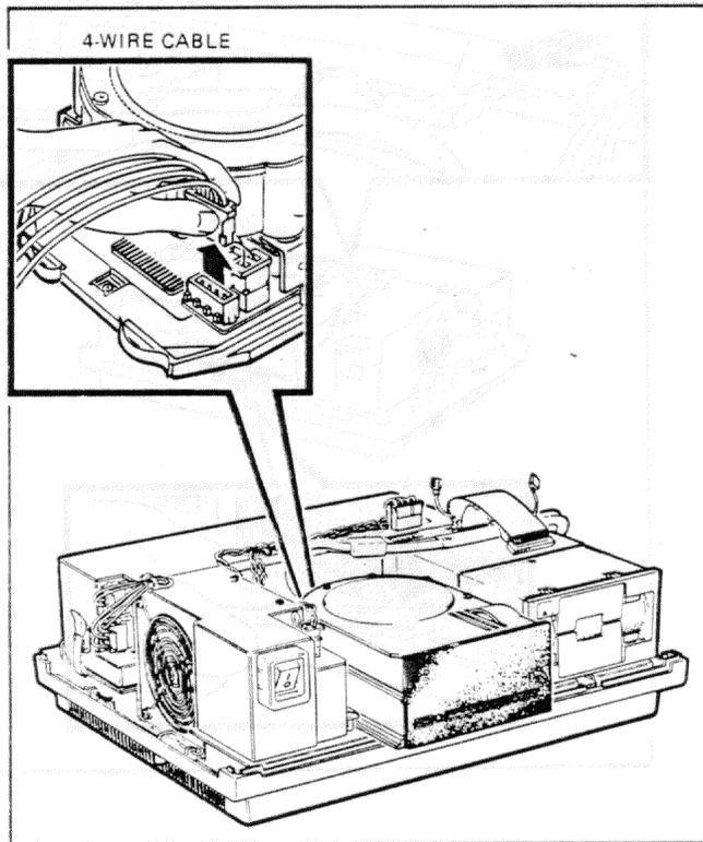
**Step 13.** Squeeze the ends of the two fan assembly plugs and unplug them from the power supply. The plugs are tight so you will need to use some force to squeeze them; however, DO NOT pull on their wires.
