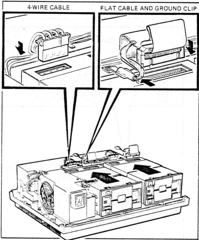
**Step 4.** Make sure the other end of the flat cable for diskette drive C/D is installed in its connector on the system module and that its ground clip is attached.
