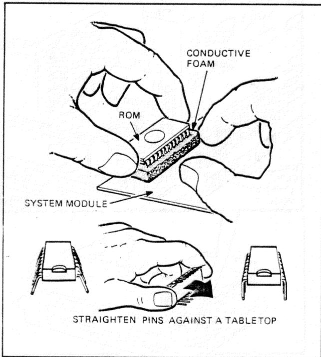
**Step 5.** Alternately, press the top of the ROM at each end until it seats *firmly* in its socket.
