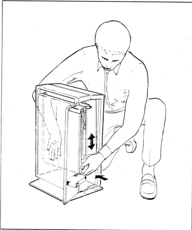
**Step 4.** Connect the cables previously removed. Plug in the power cord. Arrange the cables as shown in the door of the floor stand and run the power cord out the bottom. Close the door.
