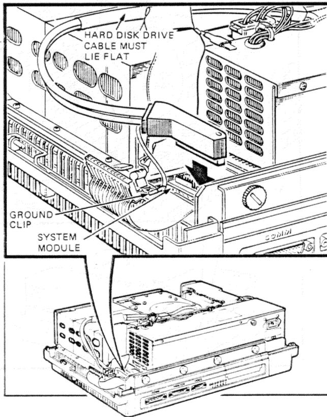
**Step 6.** Plug the power cable *firmly* into power supply.
