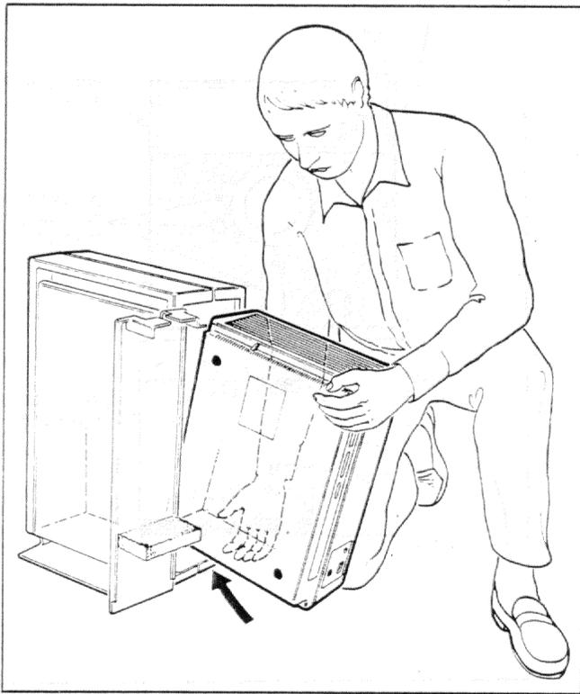
**Step 2.** Slide the system unit into the floor stand.
