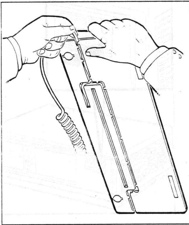
**Step 4.** Install the keyboard feet, if desired.
