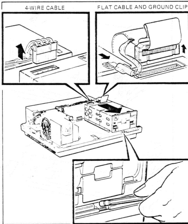
**Step 2.** Hold diskette drive C/D with its sockets facing up and slide it partially into the system unit on its tracks. Place the folded cable between the power supply and both diskette drives.
