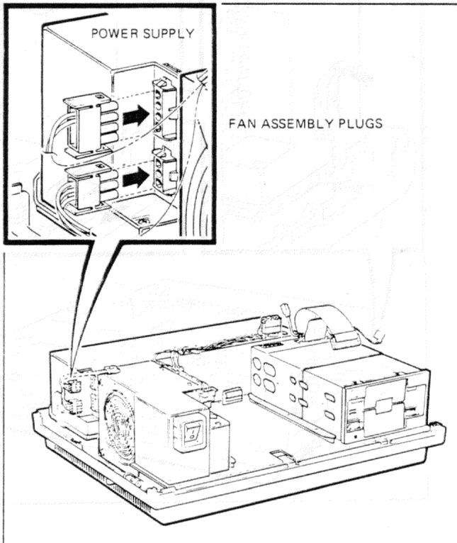
**Step 6.** If the fan assembly has another connector at the front, plug the 2-wire plug from the power supply into that connector. Otherwise, place this plug so it will not interfere with installing the top cover.
