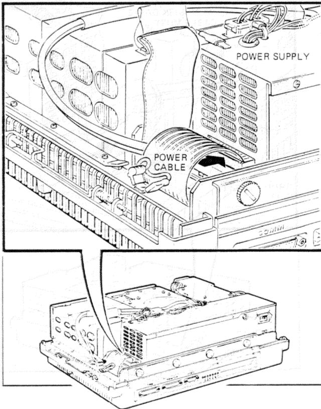
**Step 18.** Place the top cover on the system unit. Slide the cover release tabs in and away from you until they spring back, locking the cover. Try lifting the cover to make sure it is secure.
