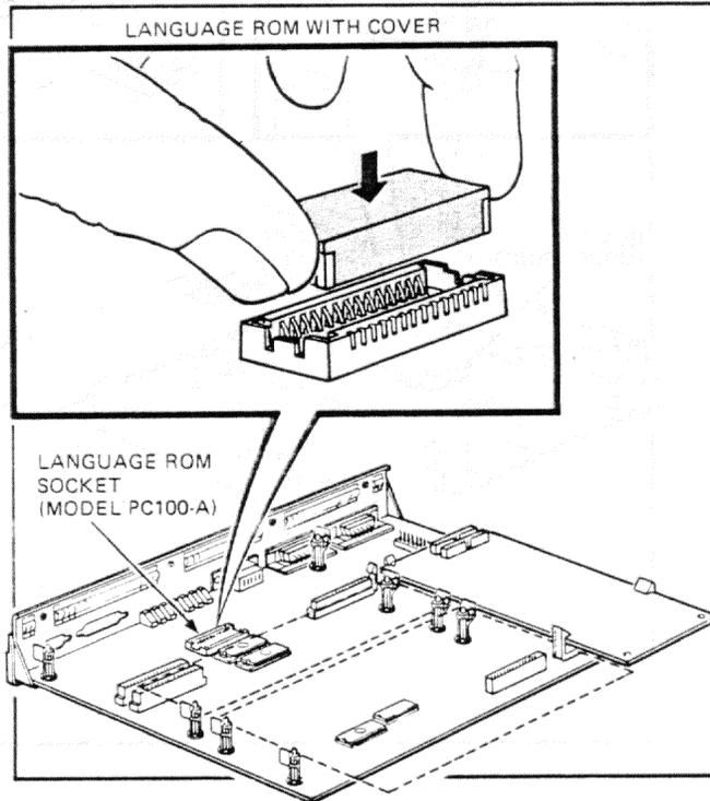
**Step 2.** Seat the ROM *firmly* in the socket by pressing down *only* on the ROM tabs.
