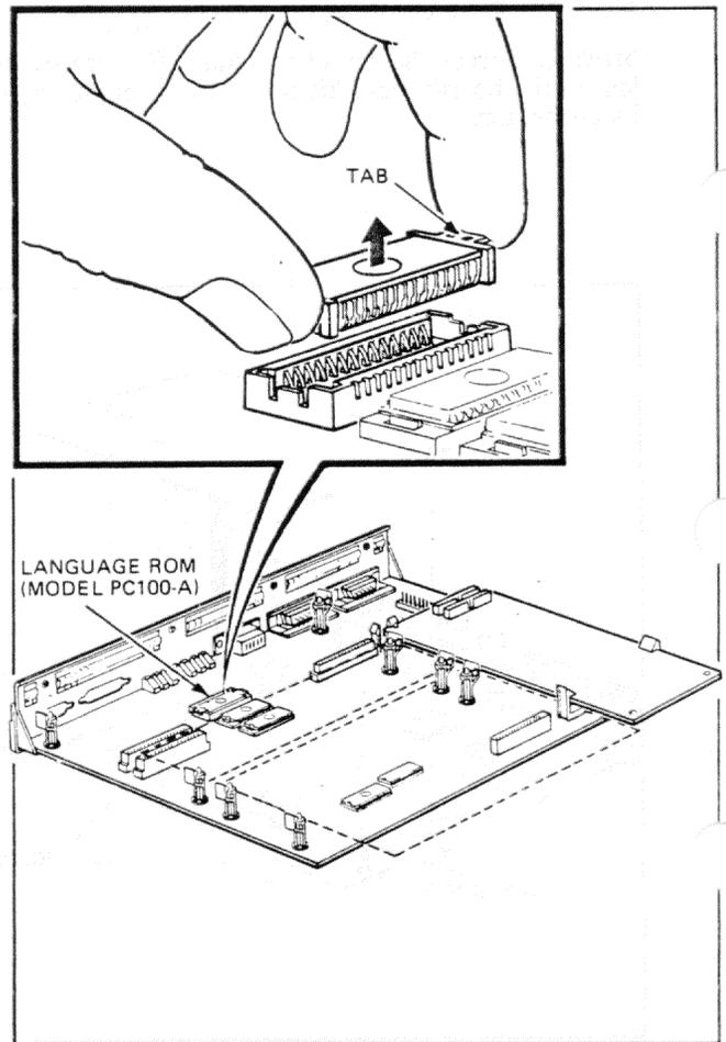
**Step 4.** If you have a model PC100-B system module, use a small flat screwdriver or ROM removal tool (part number 74-30612-01) to gently lift each end of ROM 1 until you can lift it out of its socket.
