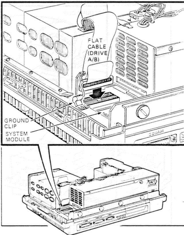
**Step 14.** Plug the diskette drive C/D flat cable into the connector on the system module. Fasten its ground clip to the ground lug.
