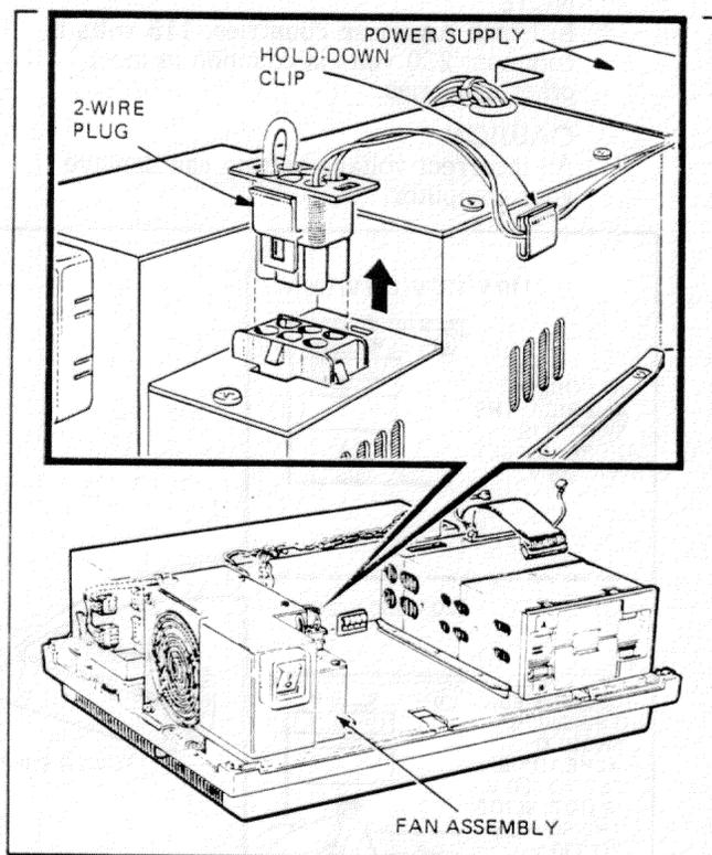
**Step 15.** Pull down the latch on the side of the power supply (or slide the latch on the system unit toward its rear), tilt the power supply up, and remove it from the system unit.
