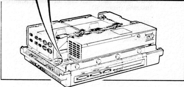
**Step 9.** Use the pull tab and remove the flat cable for diskette drive A/B from the system module. Leave the ground clip attached.
