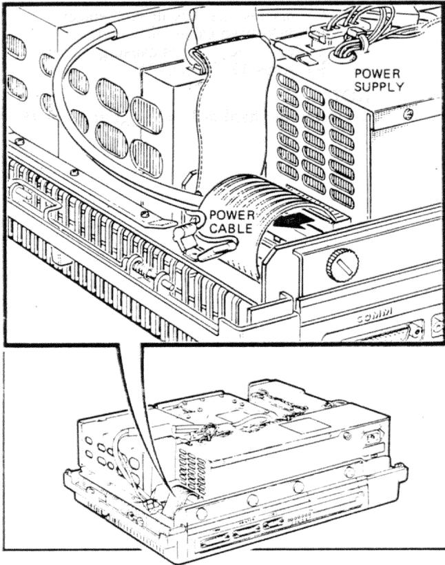
**Step 13.** Unplug the hard disk drive cable from the system module and detach its ground clip from the ground lug.
