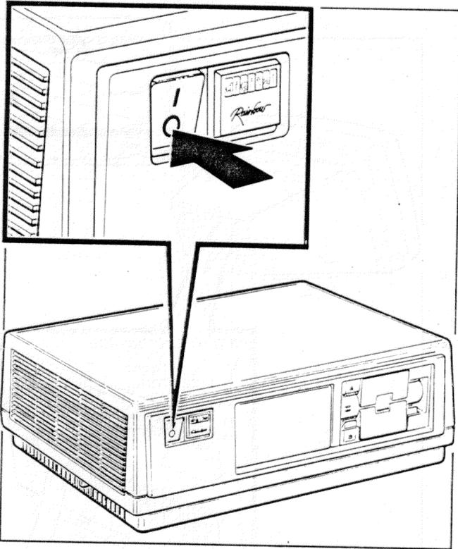
**Step 2.** Connect the cables and the power cord previously removed from the system unit. Plug the power cord into the wall socket.
