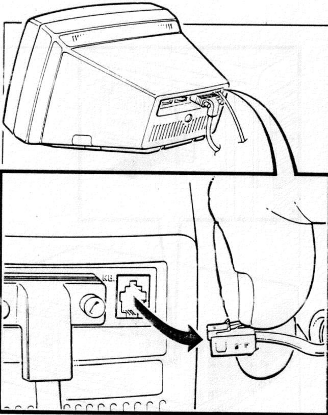
**Step 4.** Loosen the thumbscrews on the monitor cable; then, disconnect the cable from the monitor.
