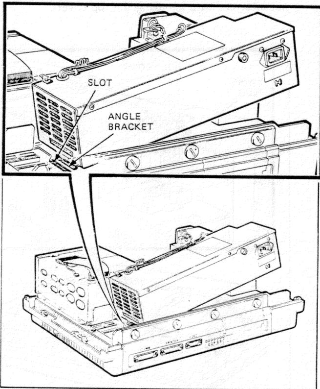
**Step 4.** Press down on the power supply and lock the latch. Try pulling up on the power supply to make sure it is locked in place.
