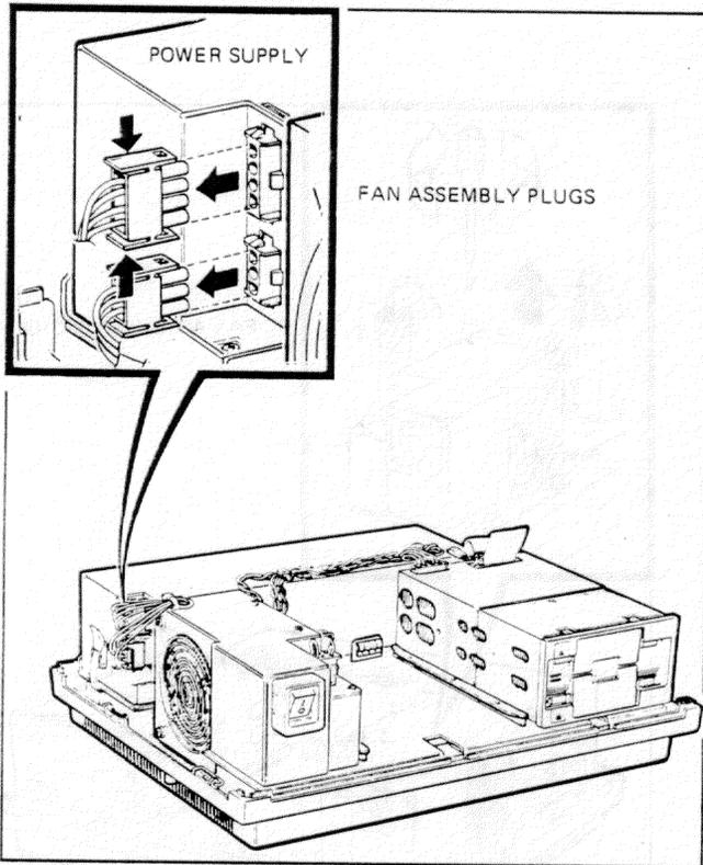
**Step 7.** If your fan assembly has another connector at the front, pull the 2-wire plug from the power supply out of the connector. Remove the wires from any hold-down clip on the side of the fan assembly.
