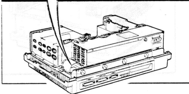
**Step 7.** If a hard disk drive cable is present, remove it from the system module before removing the power cable from the system module. Leave the ground clip attached.
