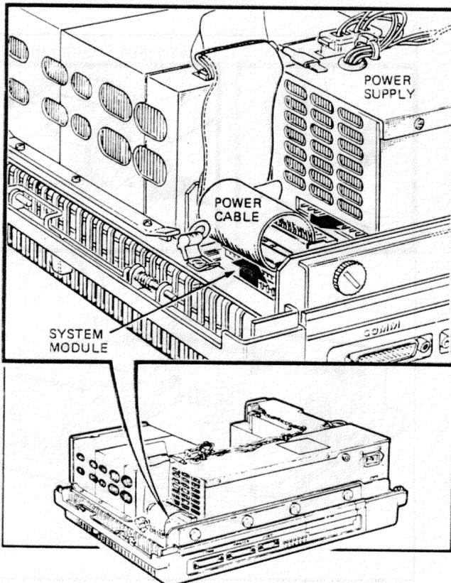
**Step 7.** If diskette drive C/D is present, remove its flat cable from the system module; then, detach its ground clip.
