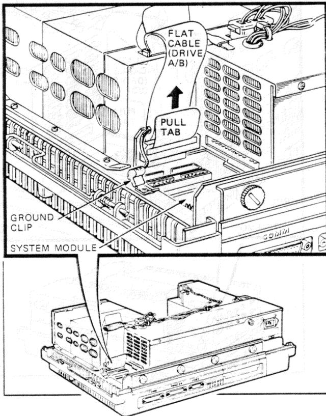
**Step 9.** Unplug the 4-wire cable from the top of diskette drive A/B. Detach the ground clip on the flat cable from the power supply. Leave the flat cable connected to the diskette drive and fold it over the top of the diskette drive.
