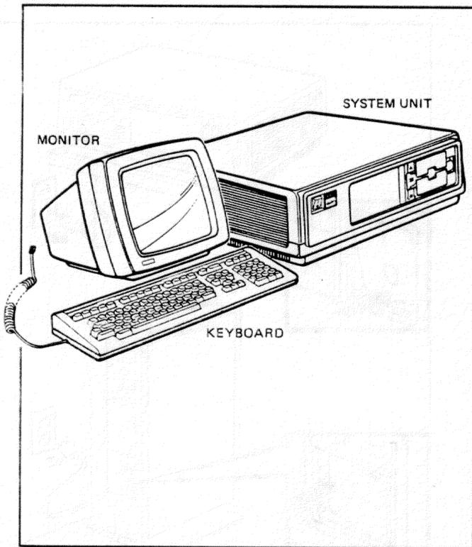
**Step 6.** Plug the keyboard cable into the back of the monitor.
