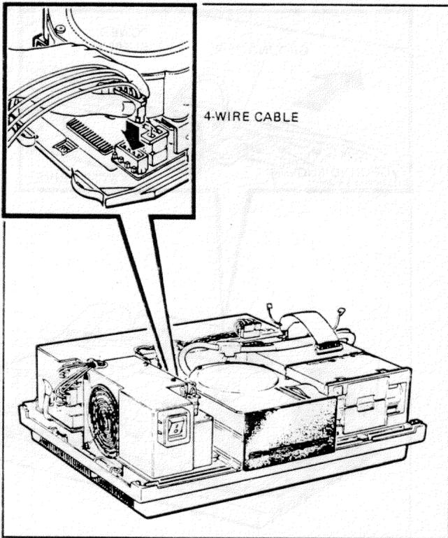
**Step 8.** Push, but do not slam, the hard disk drive completely into the system unit. Pull on the hard disk drive to make sure it is secure. Fasten the ground clip of the hard disk drive cable to the ground lug on the power supply.
