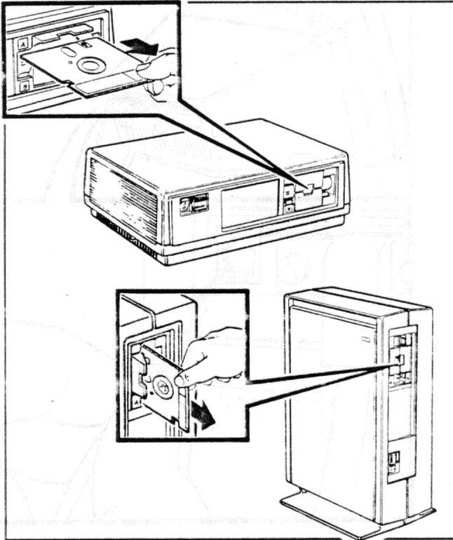
**Step 2.** Set the power switch to 0 (off) and unplug the power cord.
