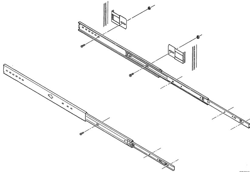
2. Now mount the slide assembly to the vertical uprights in the H9643 cabinet. First, determine the correct H9643 mounting holes. Different holes are used for different RV20 drive positions (second, third or fourth spaces from the top). Figure 4-3 shows the correct holes to use for each drive position.
