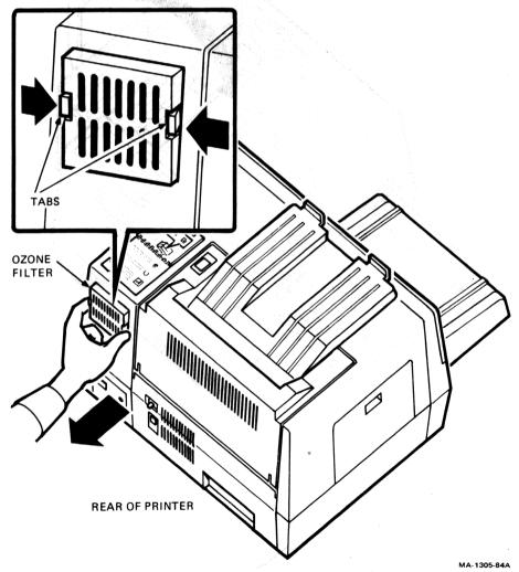
2. Insert the new ozone filter by pushing it in until it snaps into place.
