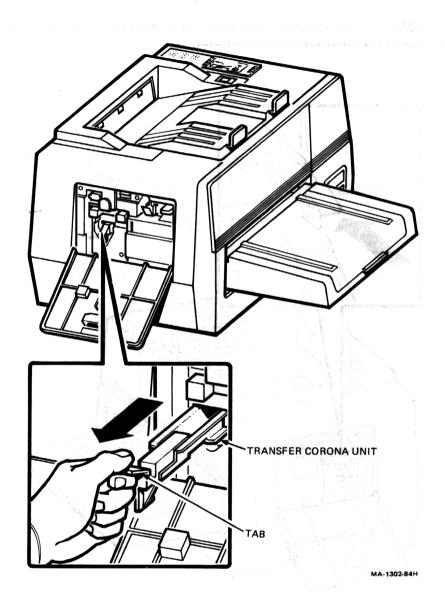
3. Insert the new corona unit (alignment guide down) until it is firmly seated in position.
