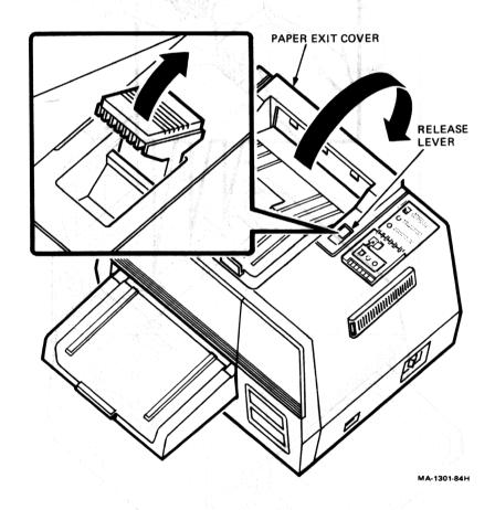
2. Remove each separation pawl by pressing it toward the front of the printer and lifting out.
