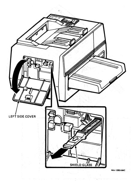
3. Insert new shield glass (arrow side up) until it is firmly seated in position.
