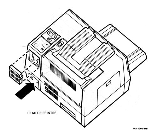
3. If the filter is mounted on the side of the printer, pull out the filter holder and remove the filter.
