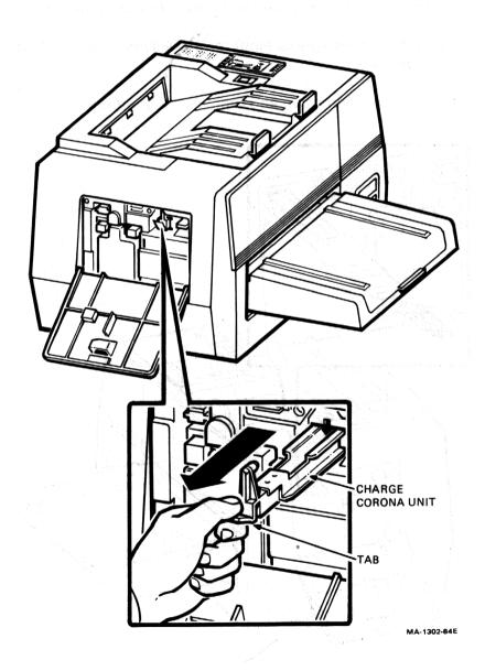
2. Insert new charge corona unit (alignment guide up) until it is firmly seated in position.
