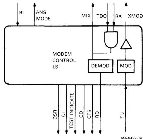
Figure 10-10 Modem Control LSI
