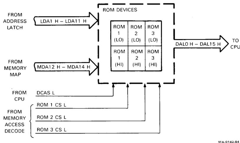
Figure 4-17 Read Only Memory (ROM) Block Diagram
