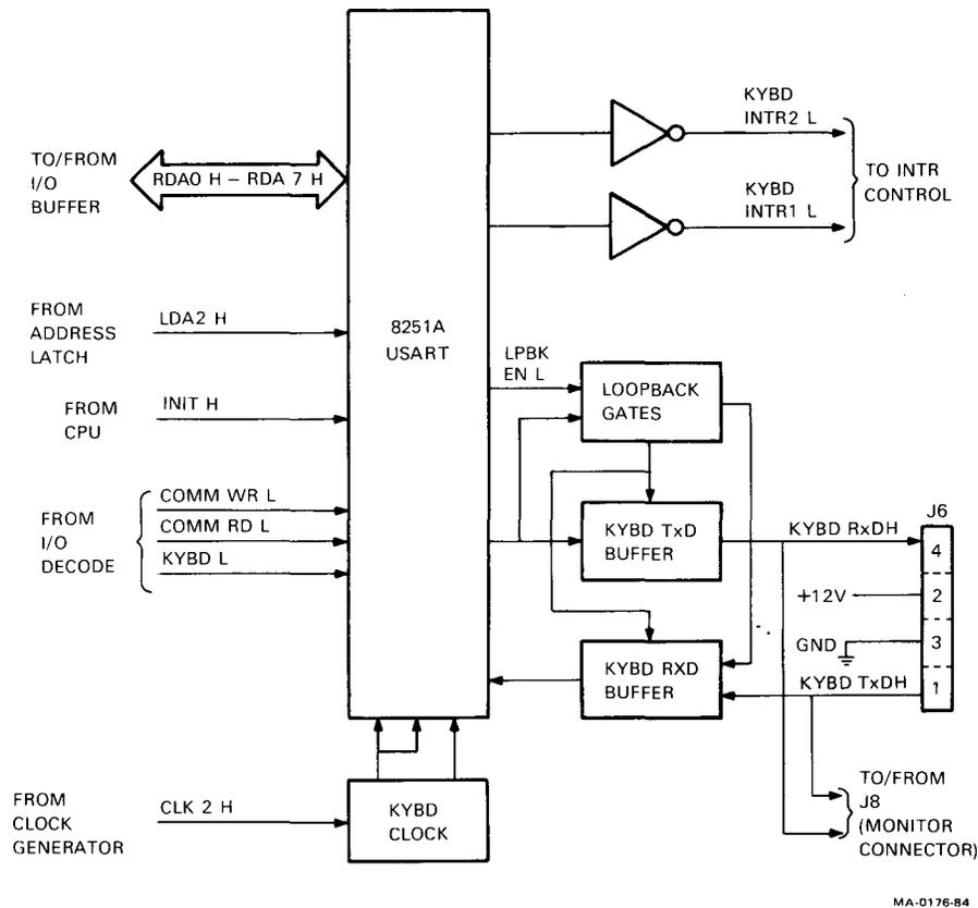
Figure 4-23 Keyboard Interface (I/F) Block Diagram
