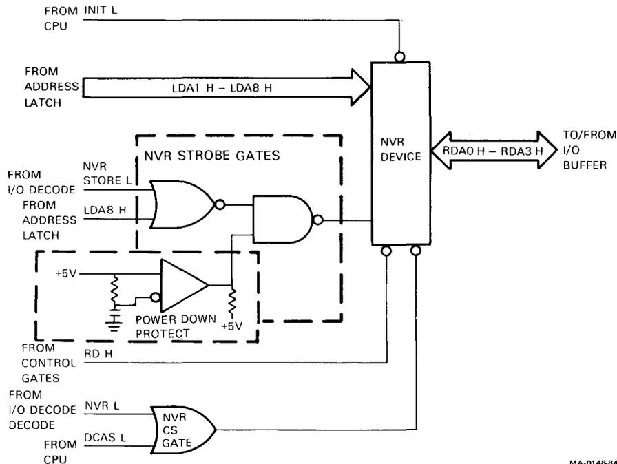
Figure 4-27 Nonvolatile RAM (NVR) Block Diagram
