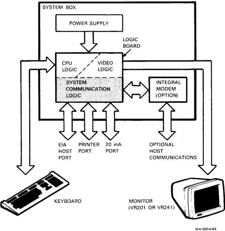
Figure 5-1 VT240-Series Terminal System Block Diagram
