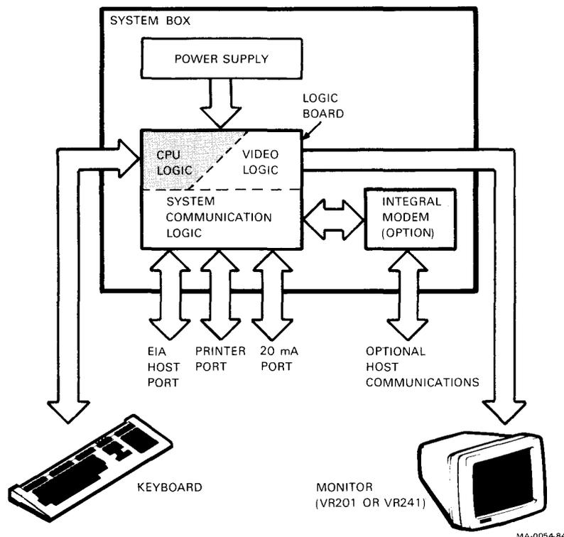
Figure 4-1 VT240-Series Terminal System Block Diagram
