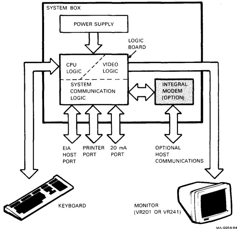
Figure 10-1 VT240-Series Terminal Block Diagram
