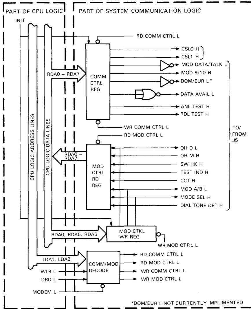
Figure 5-7 Communication/Modem (Comm/Modem) Control Block Diagram
