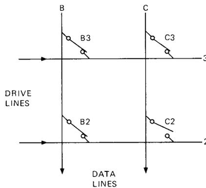
1. CONDITIONS ARE: SWITCHES B2, B3, AND C3 CLOSED, SWITCH C2 OPEN; LINE 2 IS BEING DRIVEN AND LINE C IS BEING READ.
