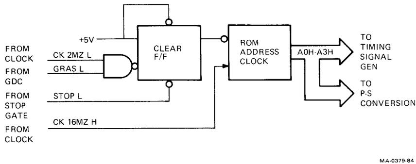
Figure 6-19 ROM Address Counter Block Diagram
