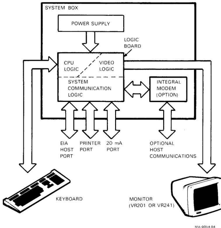
Figure 3-1 VT240 Series Terminal System Block Diagram
