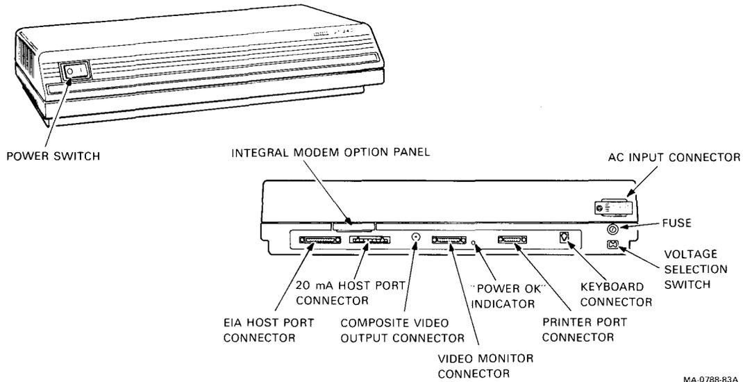
Figure 2-1 System Box Controls, Indicators, and Connectors
