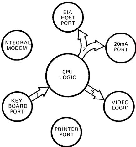
1. DATA IS TRANSFERRED FROM THE KEYBOARD TO THE CPU LOGIC.
