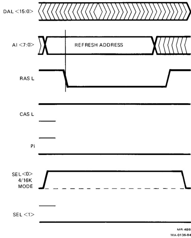
Figure 4-9 T11 Refresh Transaction Diagram
