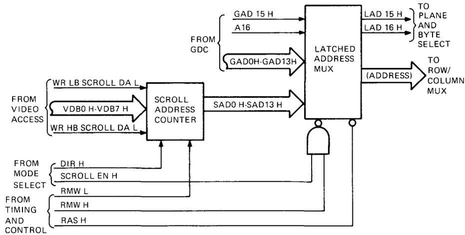
Figure 6-26 Address Select Block Diagram
