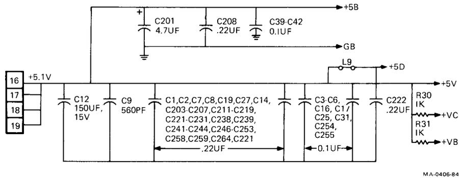
Figure 9-11 +5 V Input Circuit
