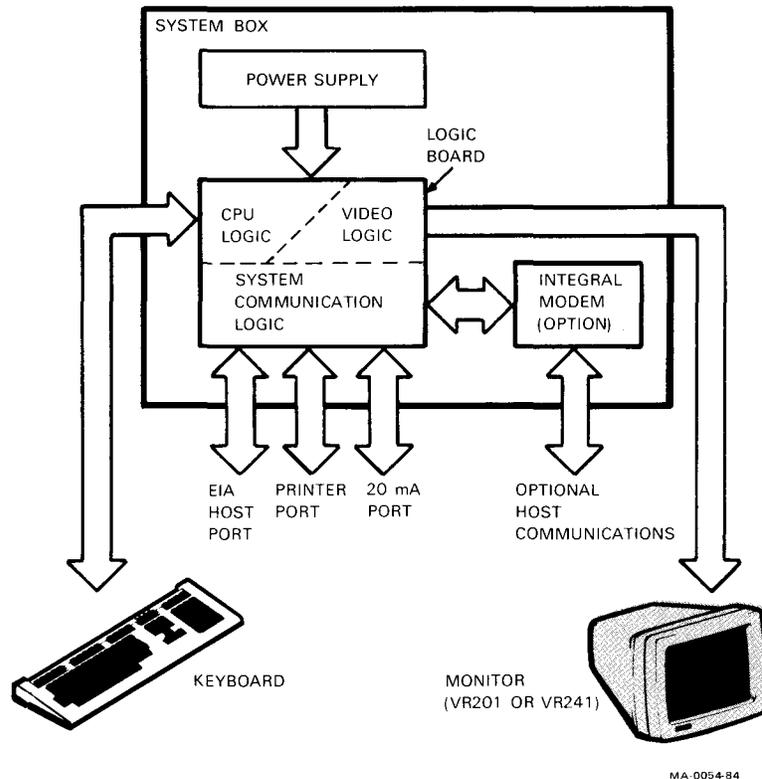
Figure 8-1 VT240-Series Terminal System Block Diagram
