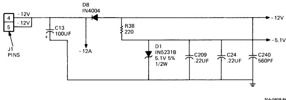
Figure 9-13 -12 V Input Circuit
