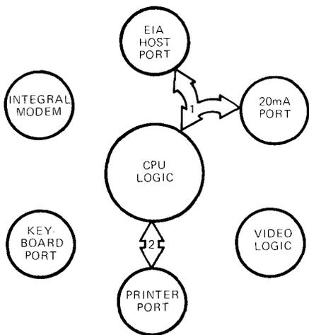
1. DATA IS TRANSFERRED BETWEEN THE CPU LOGIC AND THE HOST, VIA EITHER EIA HOST PORT, OR 20 mA PORT PORTIONS OF THE SYSTEM COMMUNICATION LOGIC.
