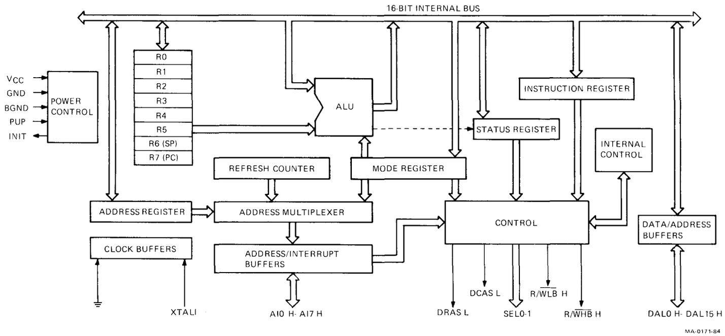
Figure 4-4 T11 Internal Block Diagram
