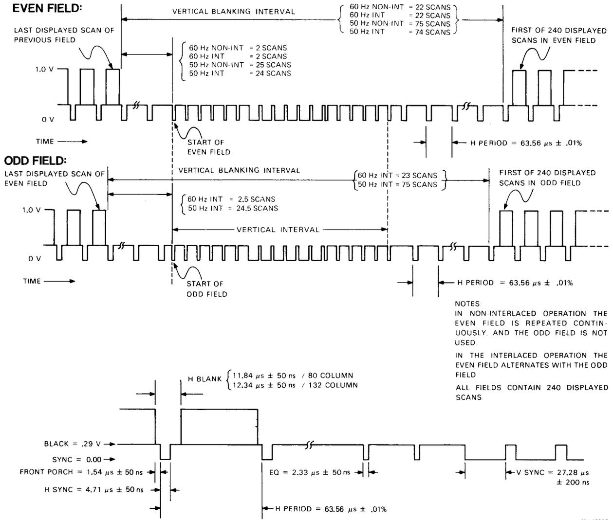
Figure 8-6 Composite Video Sync Timing Diagram
