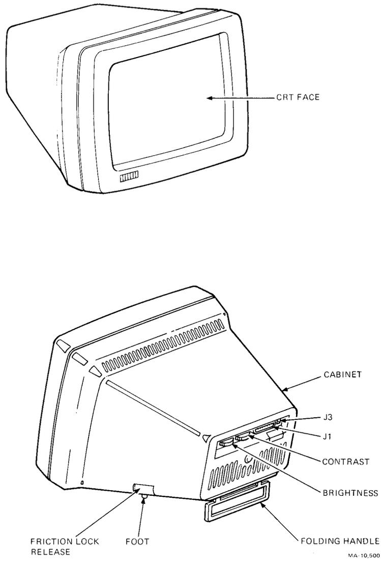
Figure 8-2 Monochrome Monitor Exterior View
