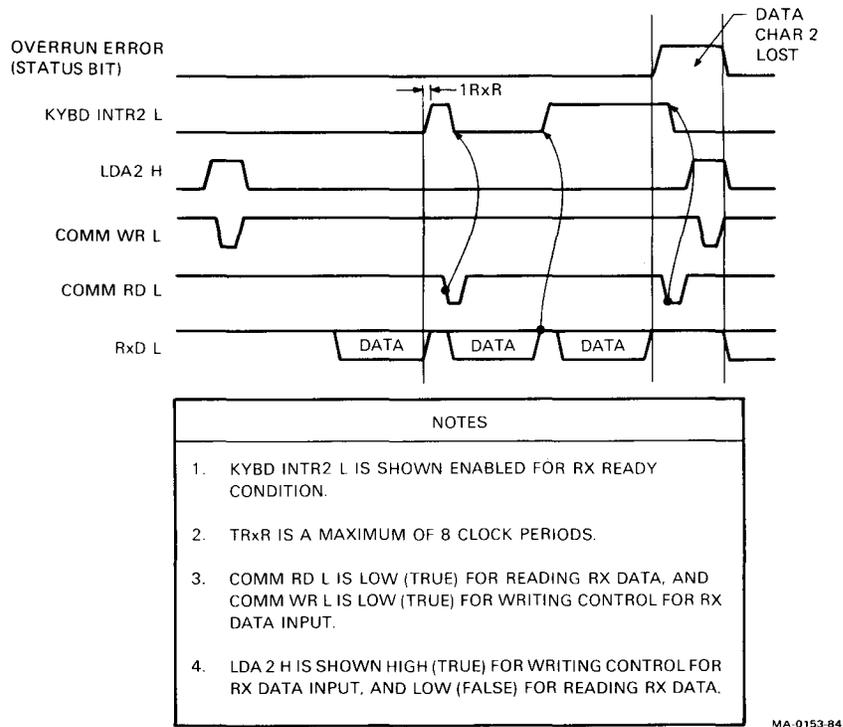
Figure 4-26 8251A USART Receive Data (RxD) Timing Diagram
