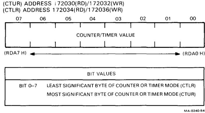
**Figure D-12 2681 DUART: Counter Timer/Upper (CTUR) and Lower (CTLR) Registers**
