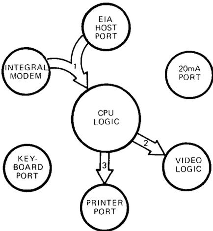
1. DATA IS TRANSFERRED TO THE CPU LOGIC FROM THE HOST, VIA EITHER INTEGRAL MODEM, OR EIA HOST PORT PORTIONS OF THE SYSTEM COMMUNICATION LOGIC.
