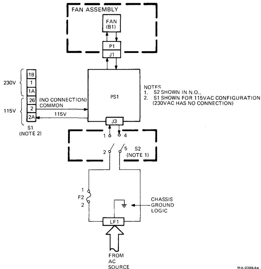
Figure 9-3 AC Input and Fan Components Block Diagram
