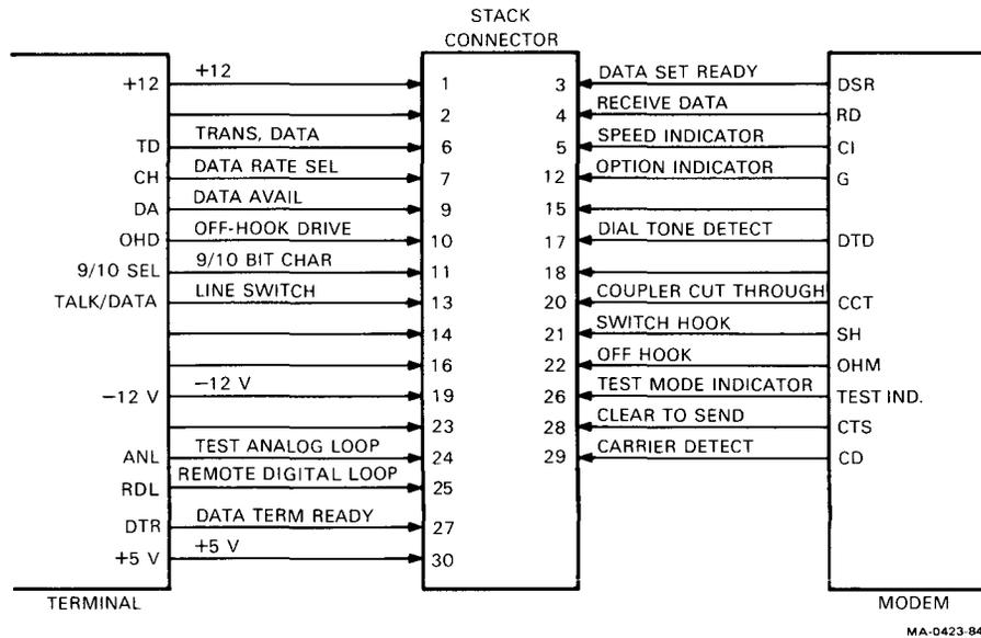
Figure 10-11 Stack Connector
