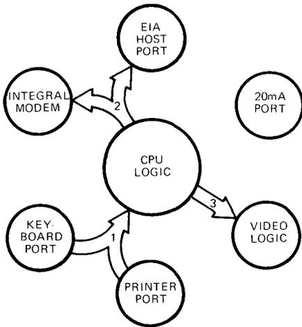
1. DATA IS TRANSFERRED TO THE CPU LOGIC FROM AN ENABLED INPUT, EITHER THE KEYBOARD, OR THE AUXILIARY DEVICE (VIA PRINTER PORT PORTION OF THE SYSTEM COMMUNICATION LOGIC); IF DATA IS PRESENT FROM BOTH SOURCES, AND BOTH ARE ENABLED, CPU LOGIC WILL DETERMINE WHICH DATA TO PROCESS FIRST.
