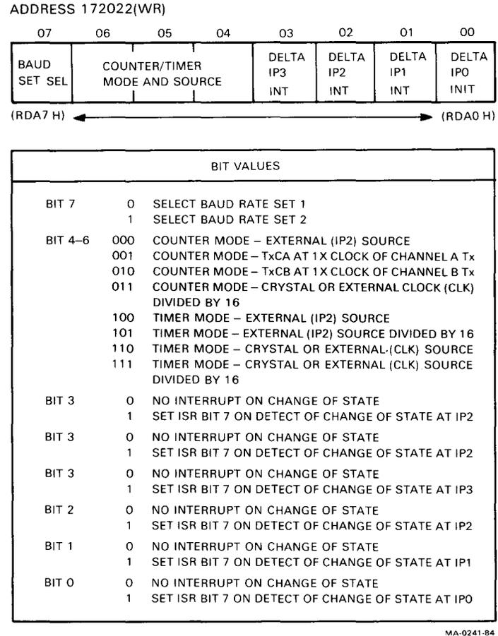
**Figure D-13 2681 DUART: Auxiliary Control Register (ACR)**
