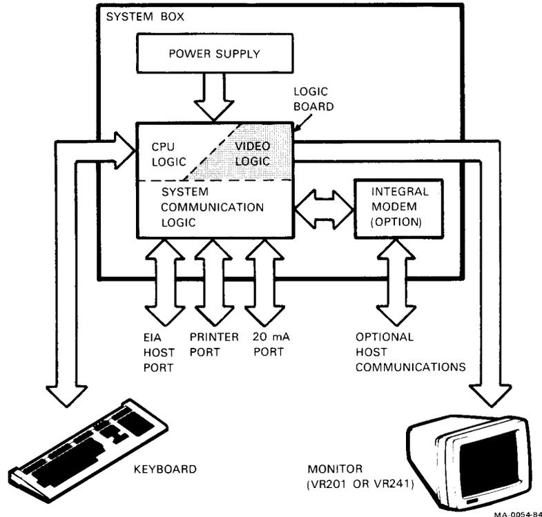
Figure 6-1 VT240-Series Terminal System Block Diagram
