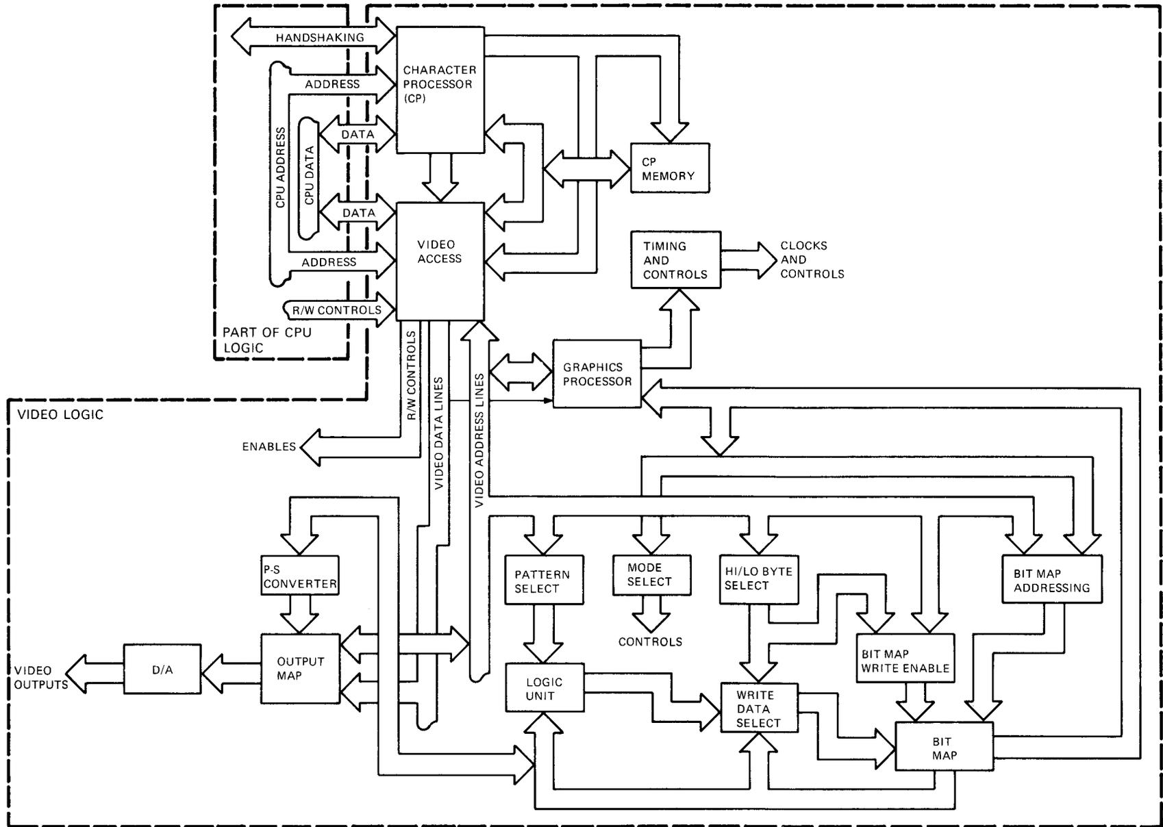
Figure 6-2 Video Logic Block Diagram
