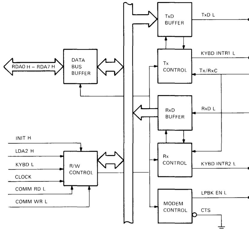
Figure 4-24 8251A USART Internal Circuits Block Diagram
