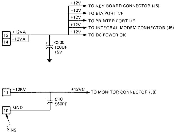
Figure 9-12 +12 V Input Circuit
