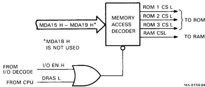
Figure 4-16 Memory Access Decode Block Diagram
