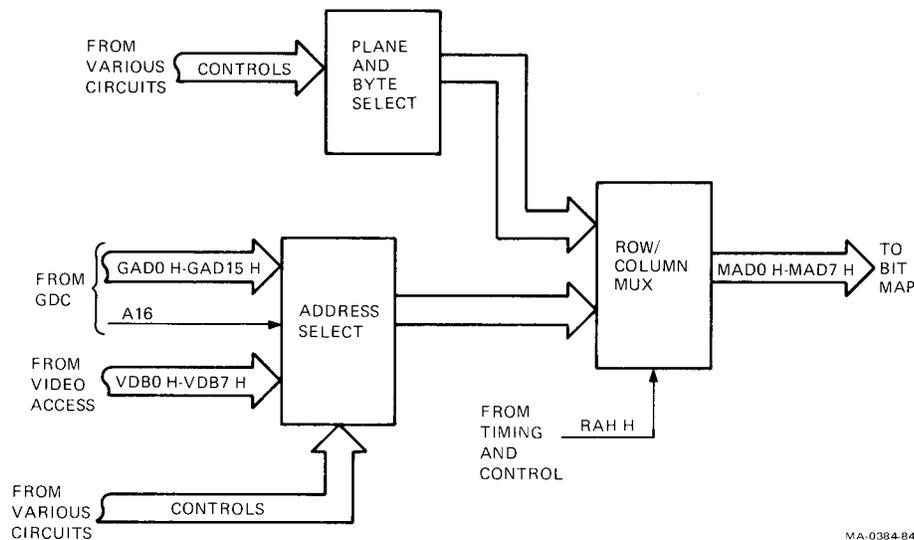
Figure 6-24 Bit Map Addressing Circuit Block Diagram
