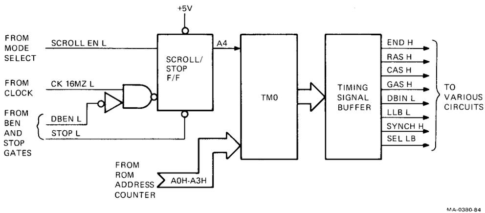
Figure 6-20 Timing Signal Generator Block Diagram
