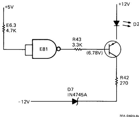
Figure 9-14 DC Power OK Circuit
