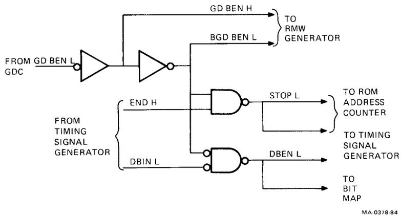
Figure 6-18 BEN and STOP Gates Block Diagram
