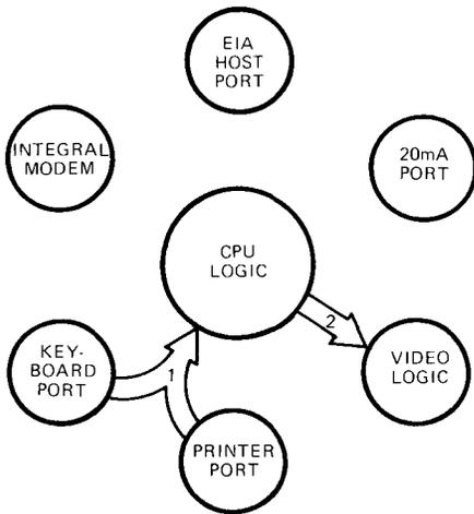
1. DATA IS TRANSFERRED TO THE CPU LOGIC FROM AN ENABLED INPUT, EITHER THE KEYBOARD, OR THE AUXILIARY DEVICE (VIA PRINTER PORT PORTION OF THE SYSTEM INTERFACE LOGIC); IF DATA IS PRESENT FROM BOTH SOURCES, AND BOTH ARE ENABLED, CPU LOGIC WILL DETERMINE WHICH DATA TO PROCESS FIRST.
