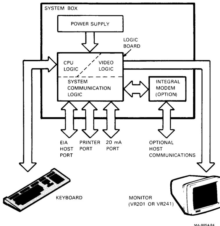
Figure 7-1 VT240-Series Terminal System Block Diagram
