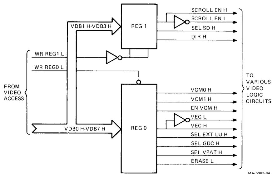
Figure 6-23 Mode Select Block Diagram
