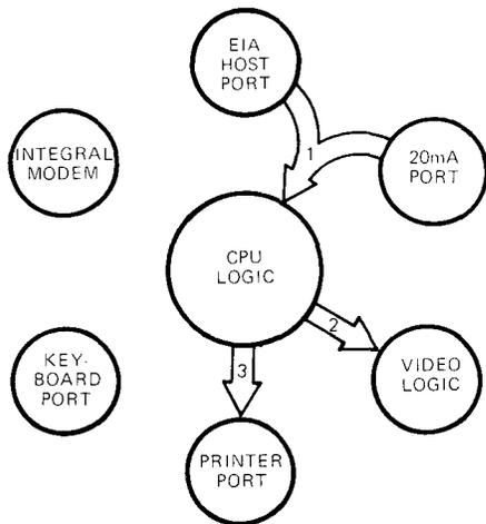
1. DATA IS TRANSFERRED TO THE CPU LOGIC FROM THE HOST, VIA EITHER EIA HOST PORT, OR 20 mA PORT PORTIONS OF THE SYSTEM COMMUNICATION LOGIC.
