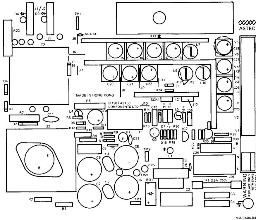
Figure 9-9 PS1 Component Layout
