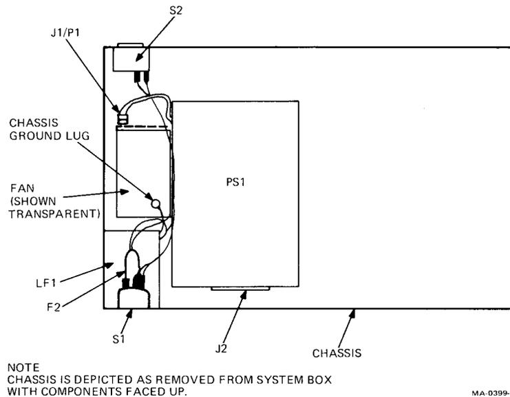
Figure 9-4 Physical Location of Power Supply Components
