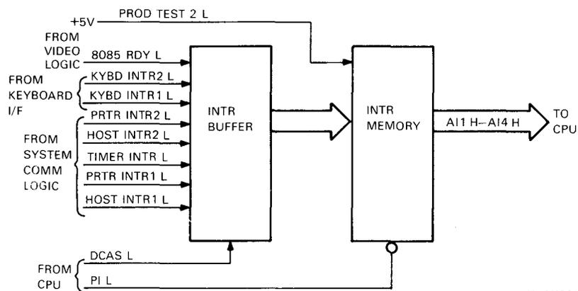
Figure 4-28 Interrupt Control Block Diagram
