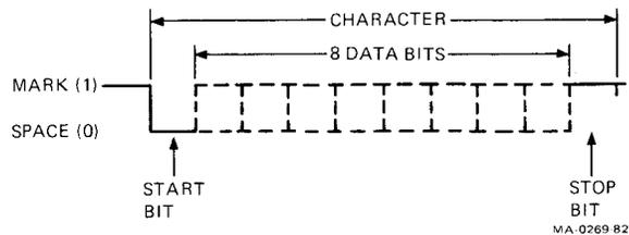
Figure 7-10 Keyboard Transmit and Receive Character Format
