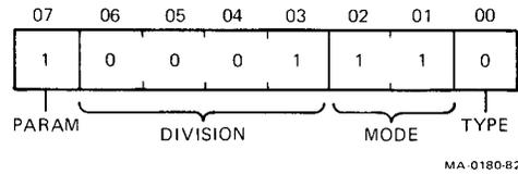
Figure 7-15 Set Main Array to Down/Up Example
