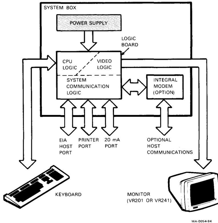
Figure 9-1 VT240-Series Terminal System Block Diagram
