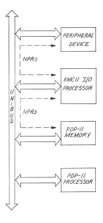
Figure 1-1 KMC11-A I/0 Microprocessor
