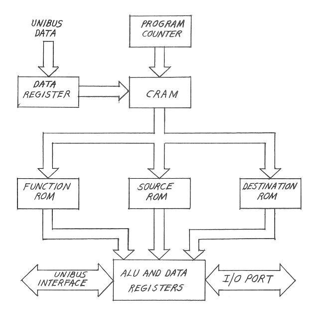
Figure 1-4 Microprocessor Simplified Block Diagram
