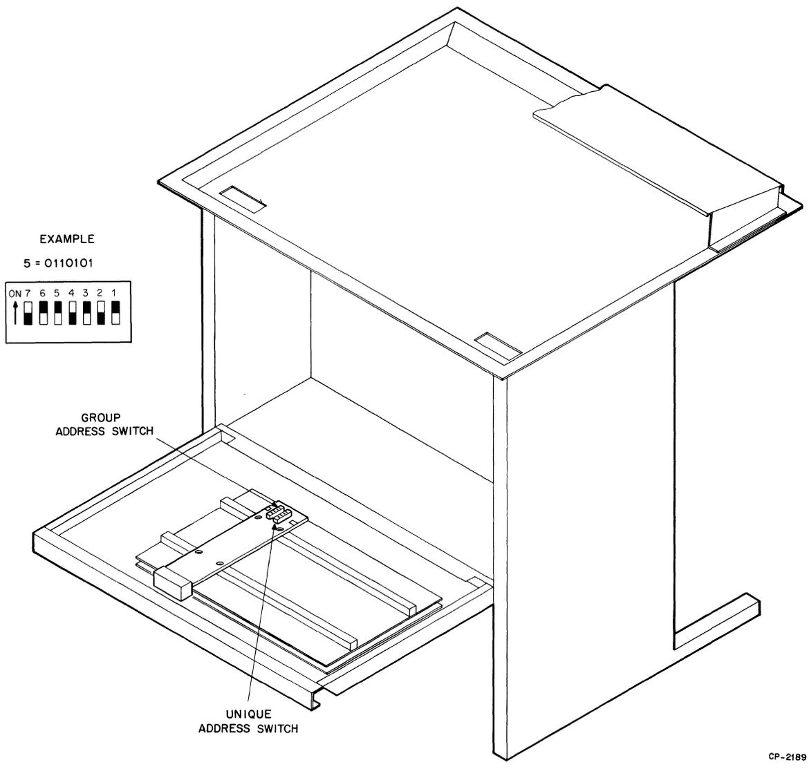
Figure 31 Location of Address Setting Switches
