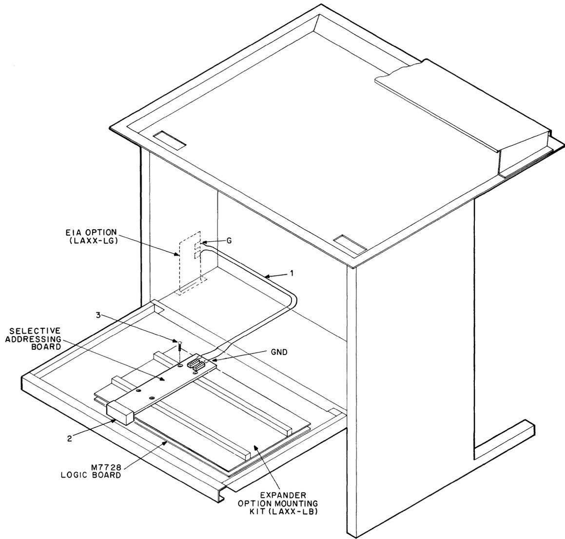
Figure 15 Installation of Selective Addressing Option Kit (LAXX-KW)
