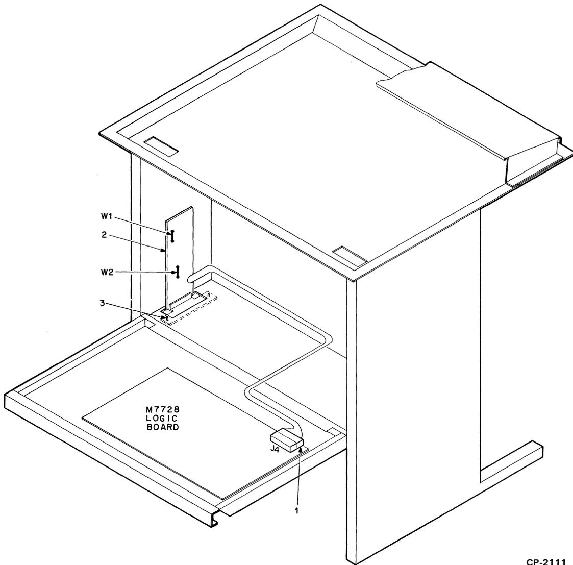
Figure 41 Installation of EIA Interface Option Kit (LAXX-LG)
