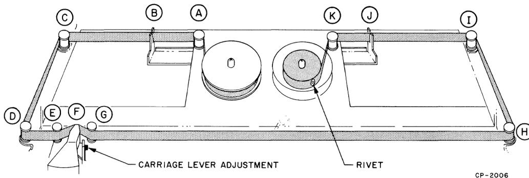
1. Place the full spool on the left spindle and turn clockwise until it drops into position.
