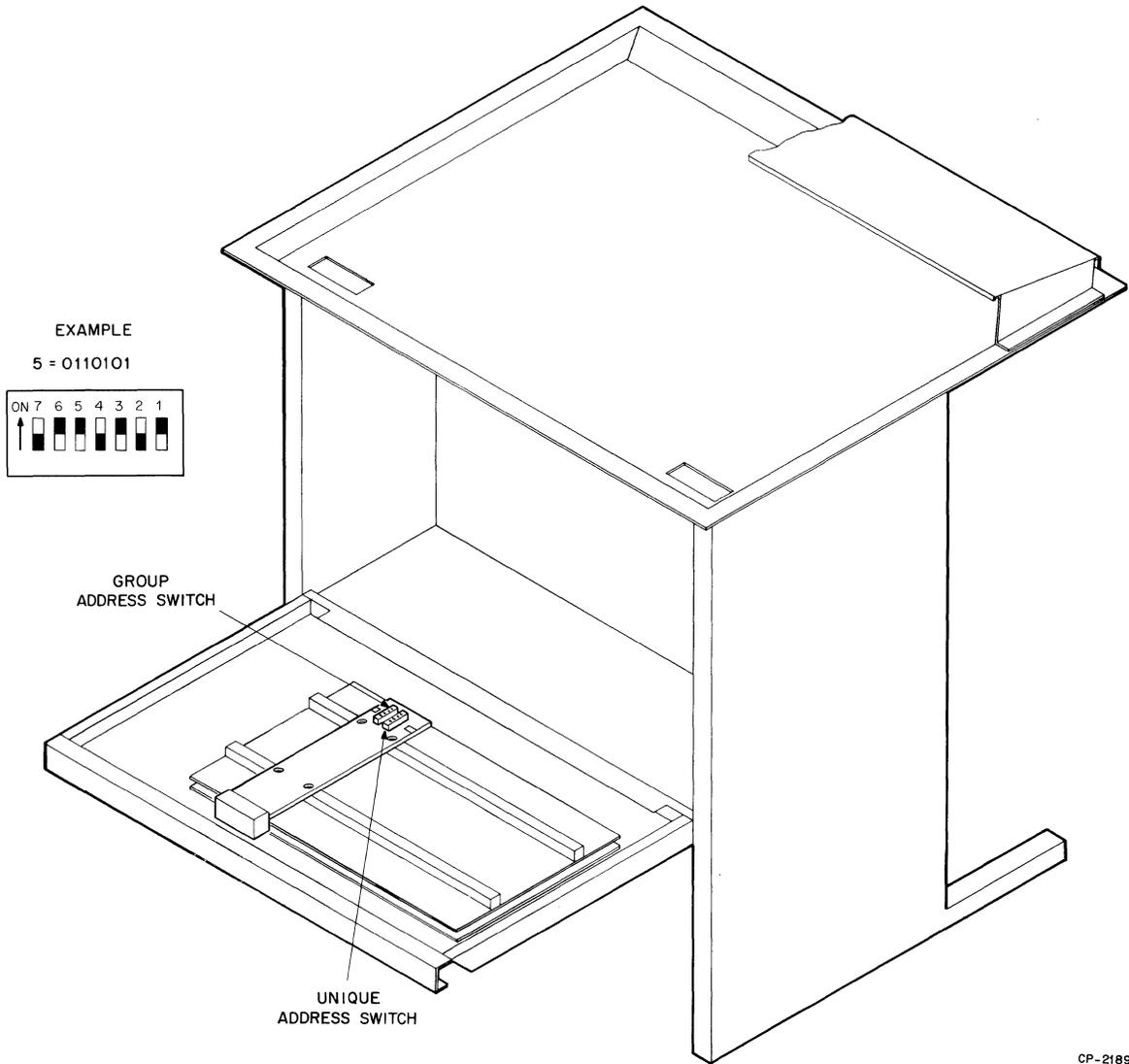
Figure 6 Location of Address Setting Switches
