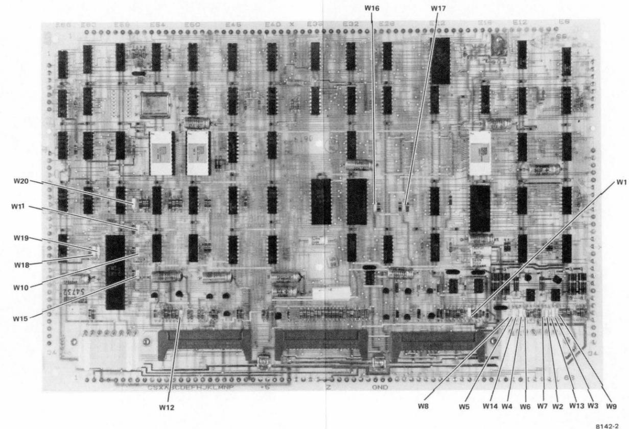
Figure 9-3 Location of Jumpers on M7728 Logic Board
