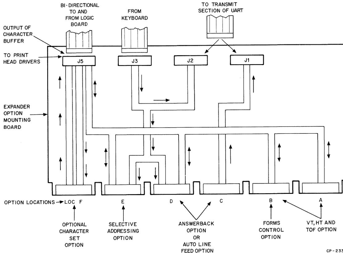
Figure 16-1 ASCII Data Distribution on Expander Board
