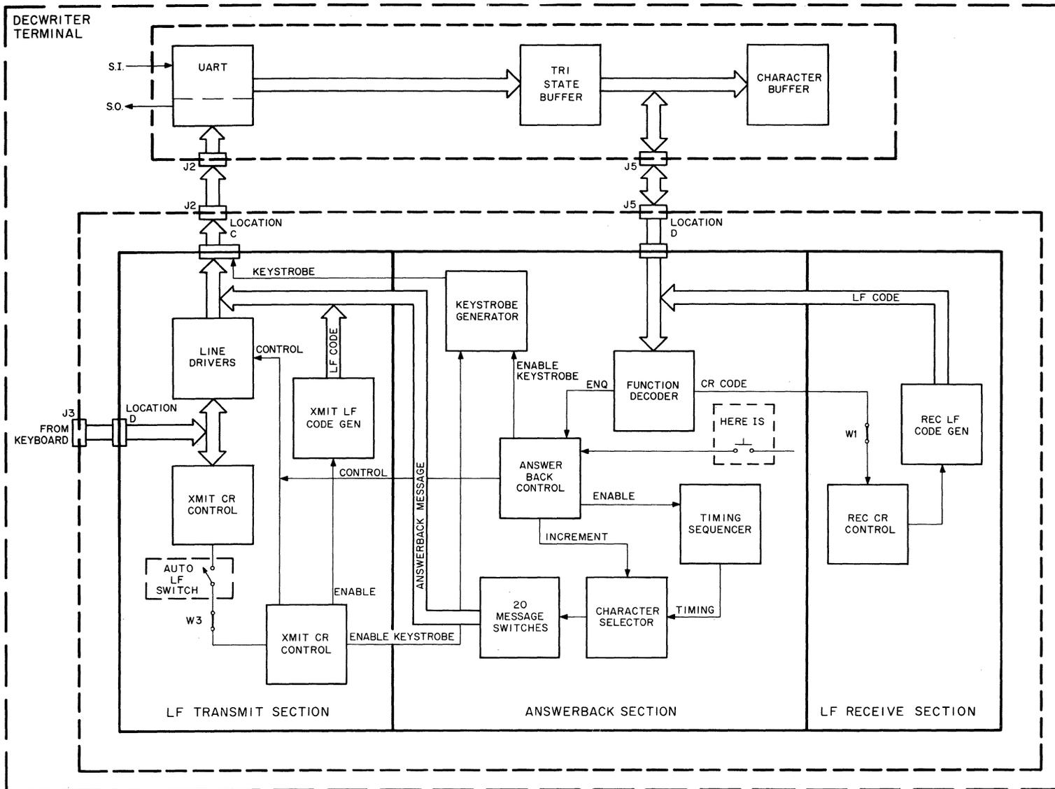
Figure 13-1 Automatic Answerback Option Functional Block Diagram
