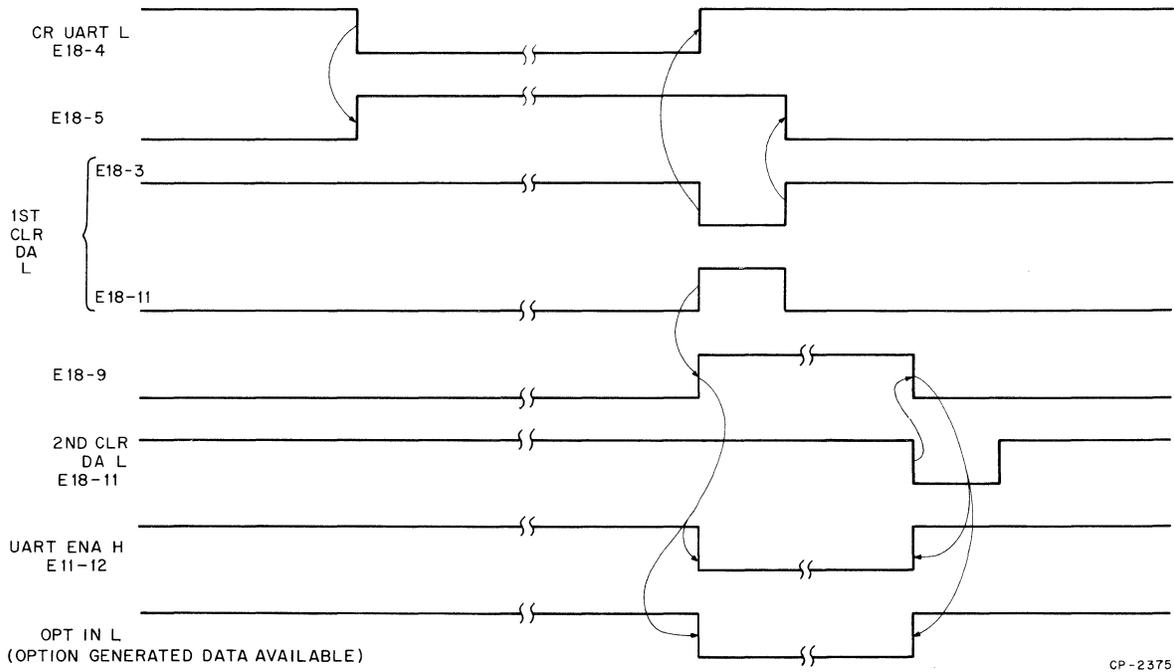
Figure 13-7 LF Receive Section Timing Sequence
