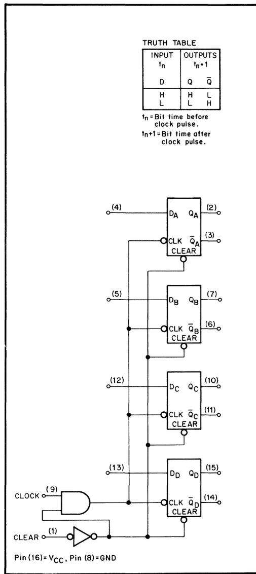
Figure A-24 74175 Quad D-Type Flip-Flop with Clear
