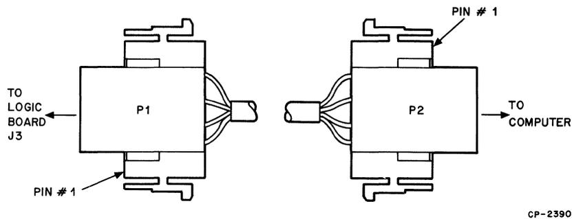
Figure 18-2 20 mA Interface Cable Option (LAXX-LH) Pin Assignments
