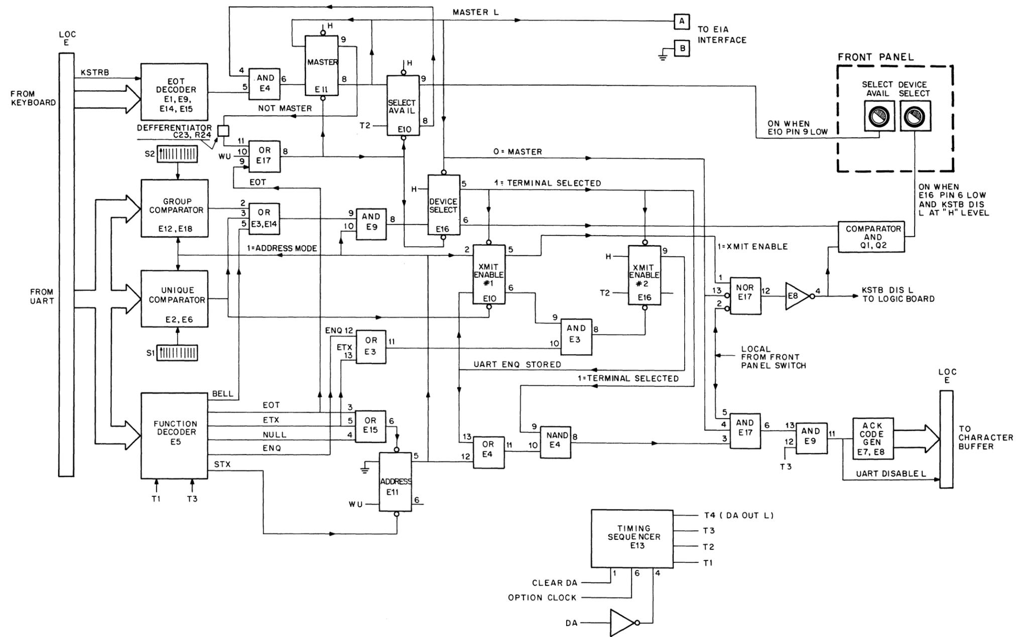
Figure 12-2 Selective Addressing Basic Block Diagram
