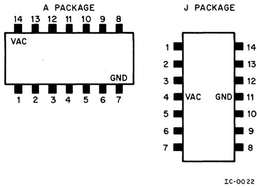
Figure A-5 7400 Quad 2-Input Positive NAND Gate
