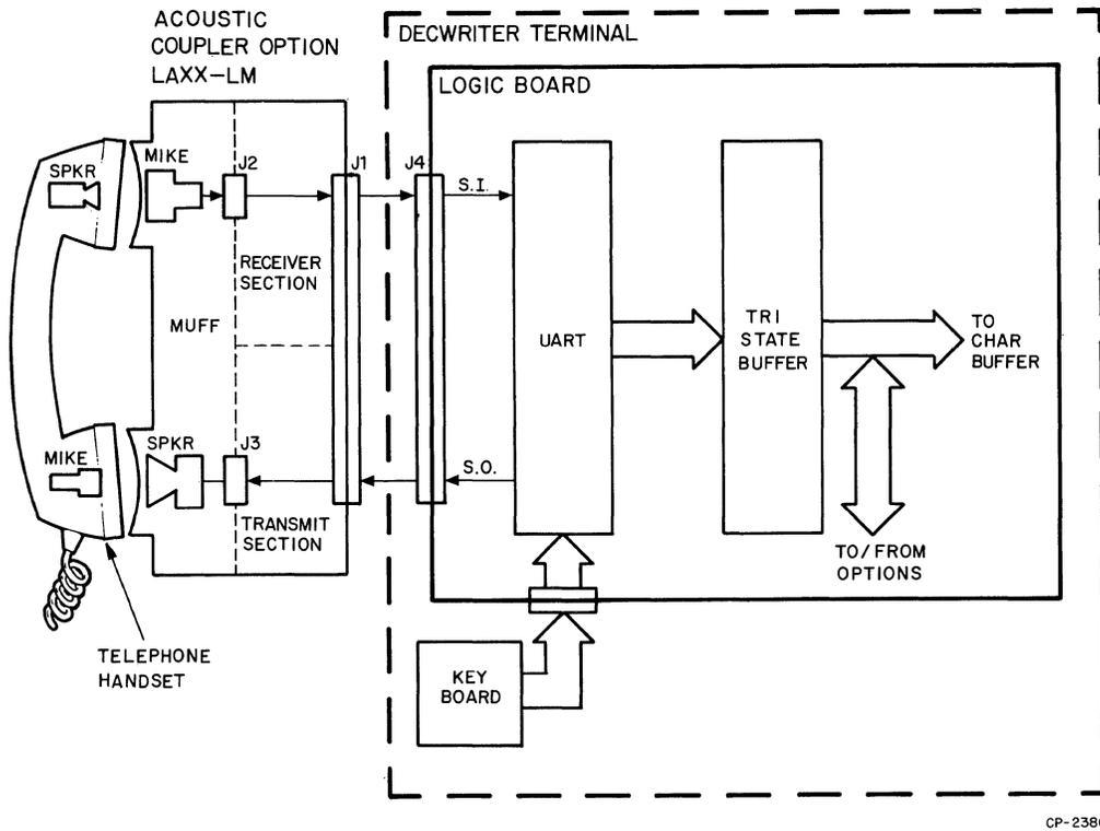
Figure 19-2 Acoustic Coupler Functional Block Diagram
