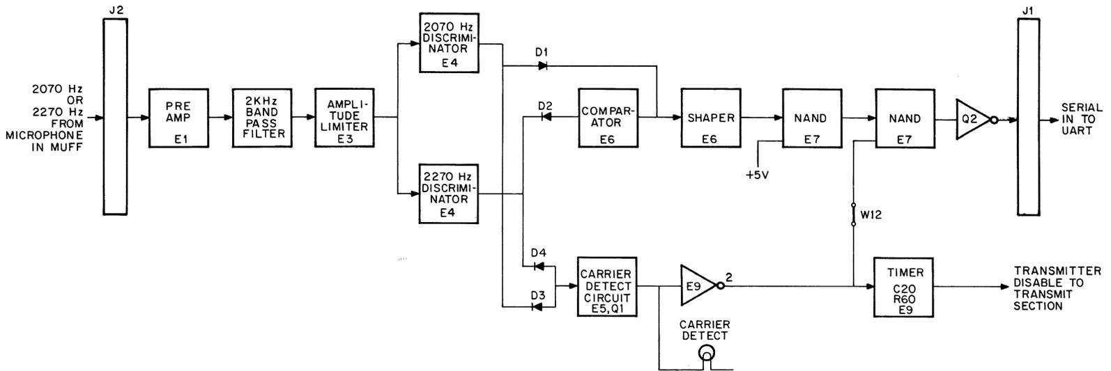
Figure 19-4 Acoustic Coupler Receive Section Basic Block Diagram
