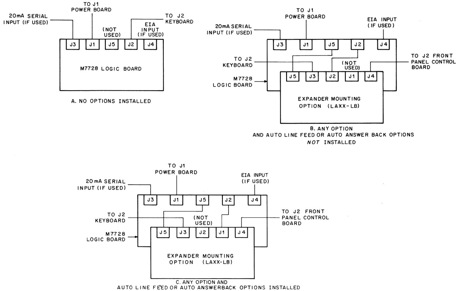
Figure 9-4 Cabling Configurations for the M7728 Logic Board
