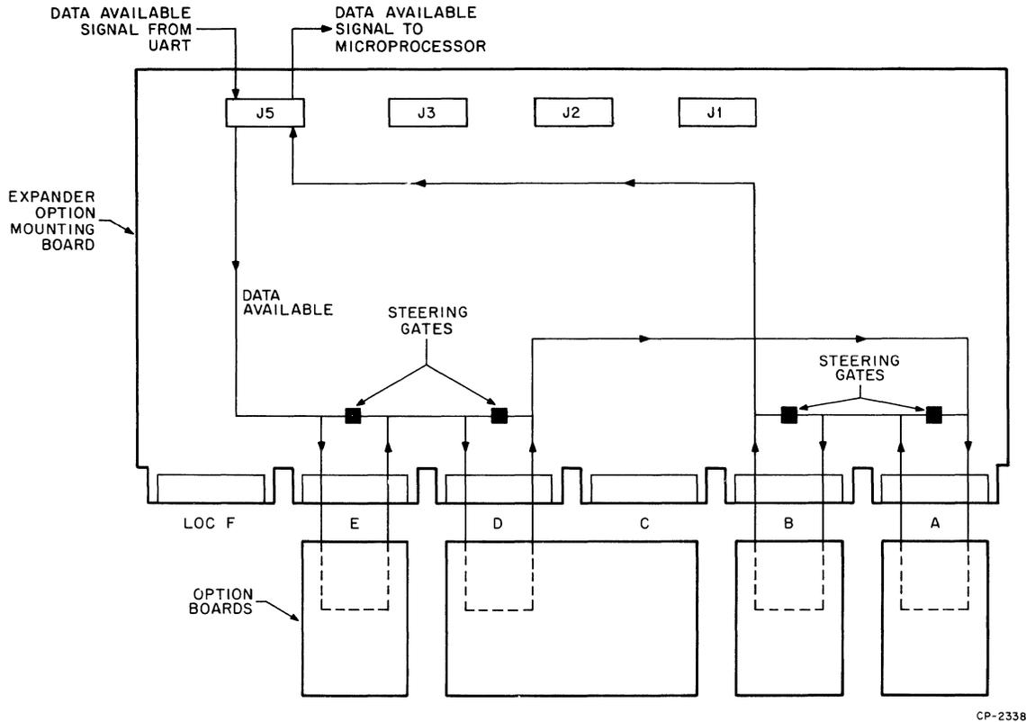
Figure 16-2 Data Available Signal Distribution on Expander Board
