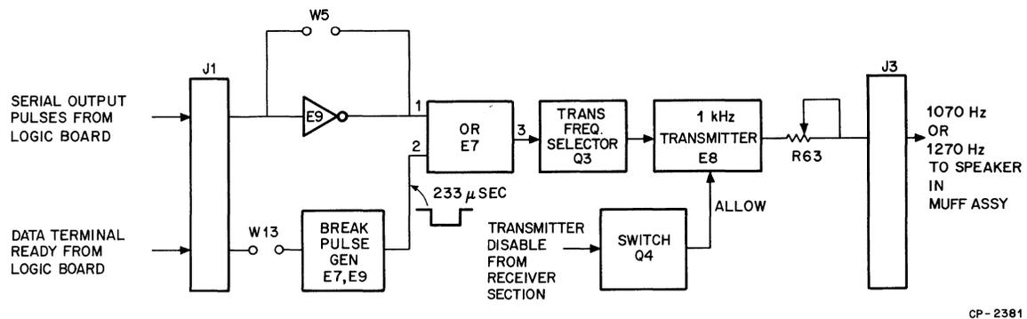
Figure 19-3 Acoustic Coupler Transmit Section Basic Block Diagram
