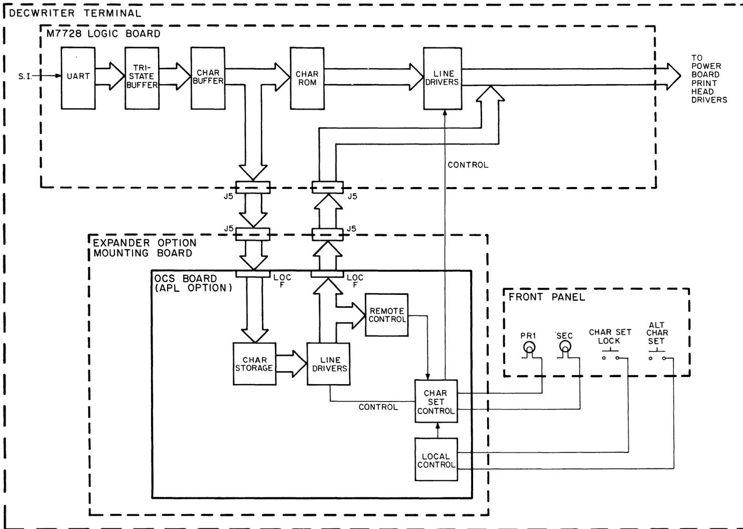
Figure 20-1 APL Character Set Functional Block Diagram
