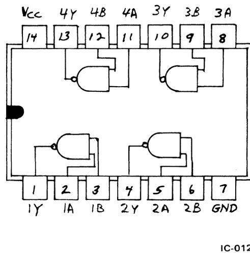
Figure A-6 7401 NAND Gate-Quad 2-Pin Open Collector
