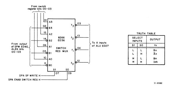
Figure 4-13 Typical Switch Register Multiplexer
