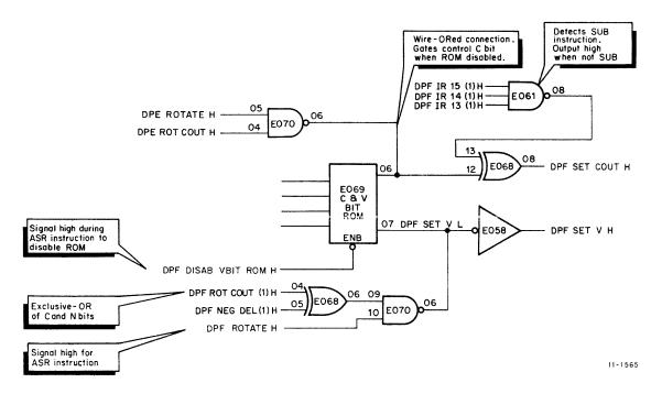
Figure 4-12 Logic For Determining C and V Bits (Example Shown for ASR Instruction)
