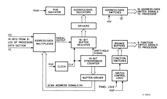
Figure 3-1 Console Functional Block Diagram
