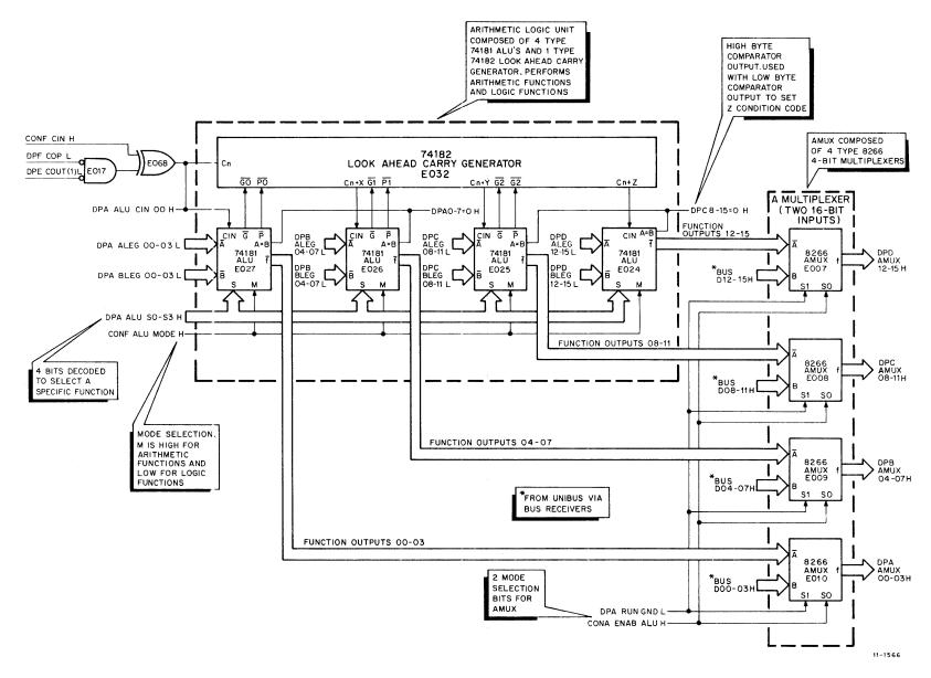
Figure 4-7 Arithmetic Logic Unit Block Diagram
