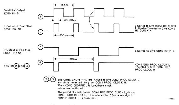
Figure 4-15 Processor Clock Timing Diagram
