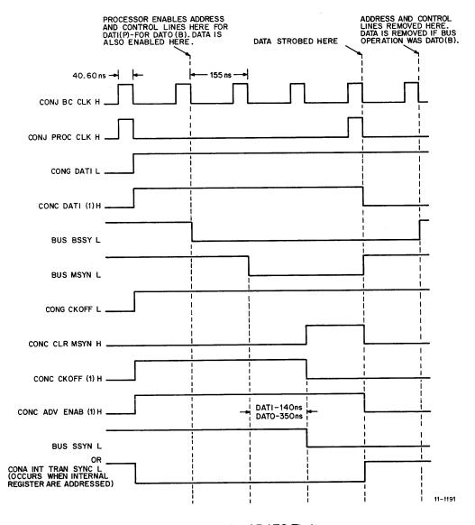
Figure 4-16 DATI and DATO Timing
