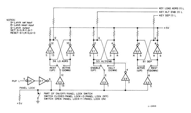
Figure 3-6 Control Switches and Bounce Buffers, Logic Diagram
