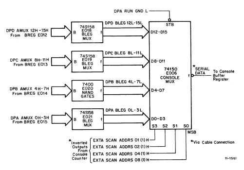
Figure 4-14 Console Multiplexer Block Diagram
