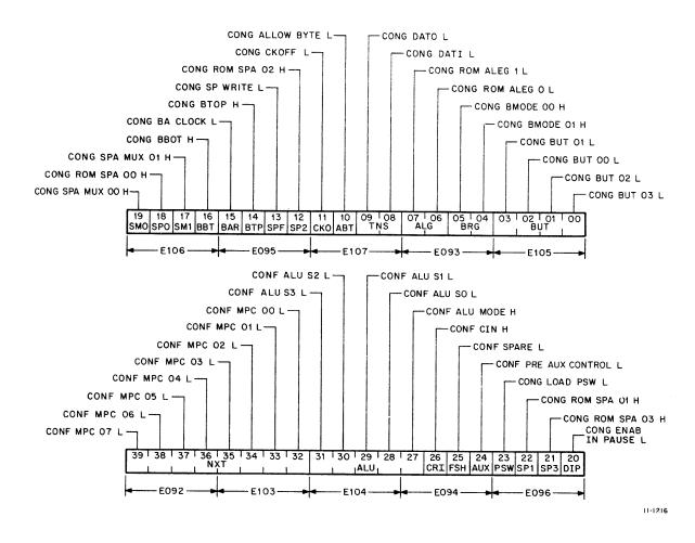
Figure 2-1 Control Store Word Bit and Field Format
