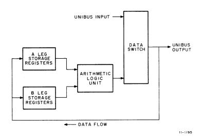
Figure 4-3 KD11-B Simplified Data Path Block Diagram
