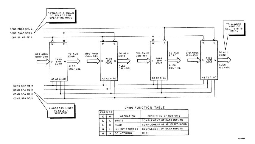
Figure 4-11 Block Diagram and Function Table for Scratch Pad Memory
