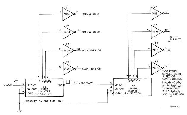
Figure 3-3 Counter, Simplified Logic Diagram
