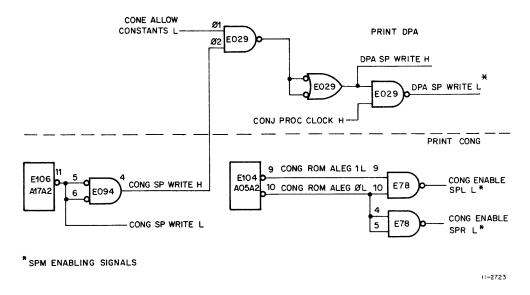
Figure 2-7 Generation of SPM Enabling Signals
