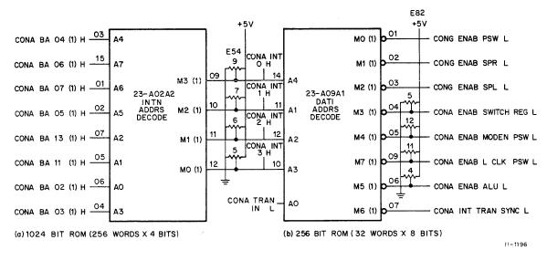
Figure 4-1 1024-Bit and 256-Bit ROMs
