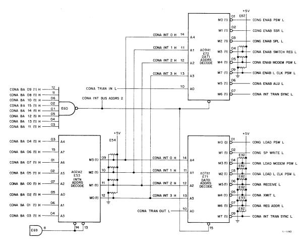
Figure 4-17 Unibus Address Decoding
