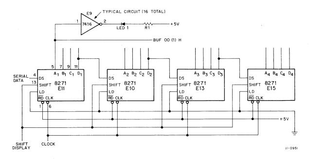
Figure 3-4 Display Buffer and Driver, Simplified Logic Diagram
