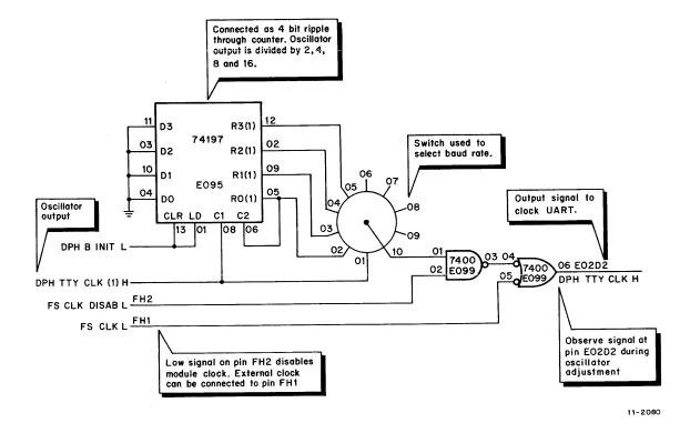
Figure 4-21 Baud Selection Logic
