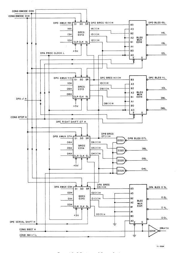
Figure 4-8 B Register and Output Logic
