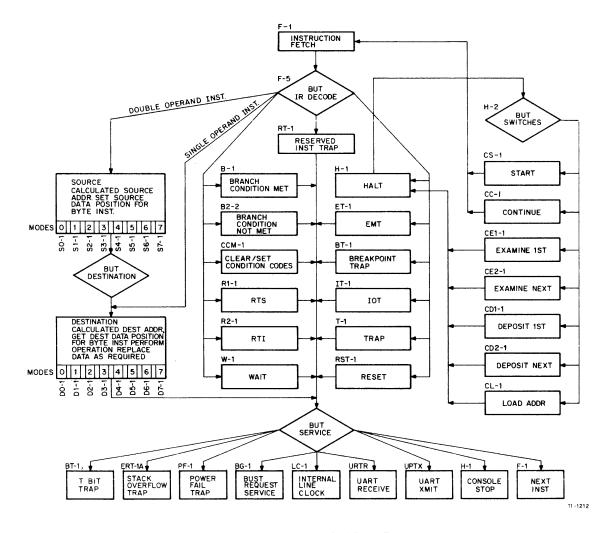
Figure 2-2 KD11-B Simplified Flow Diagram
