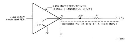
Figure 3-5 LED Driver Circuit
