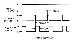
Figure 4-20 SCL Oscillator Schematic and Timing Diagram
