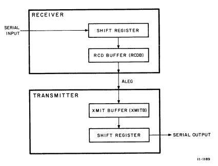
Figure 4-19 Double-Buffering Data Flow
