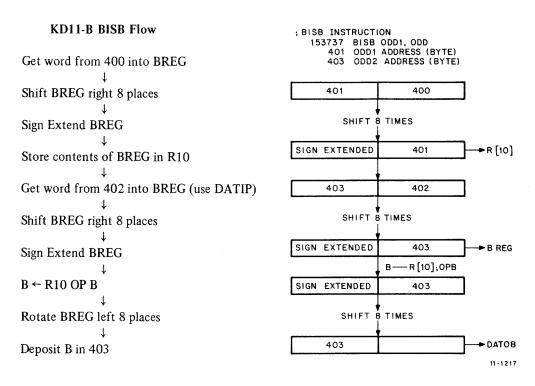
Figure 4-10 Byte Format for Shifting Instructions
