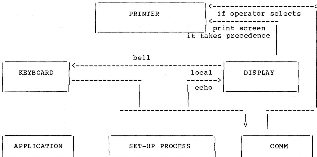
Figure 13. 'Terminal' Mode 'On Line' In 'Printer Controller'
