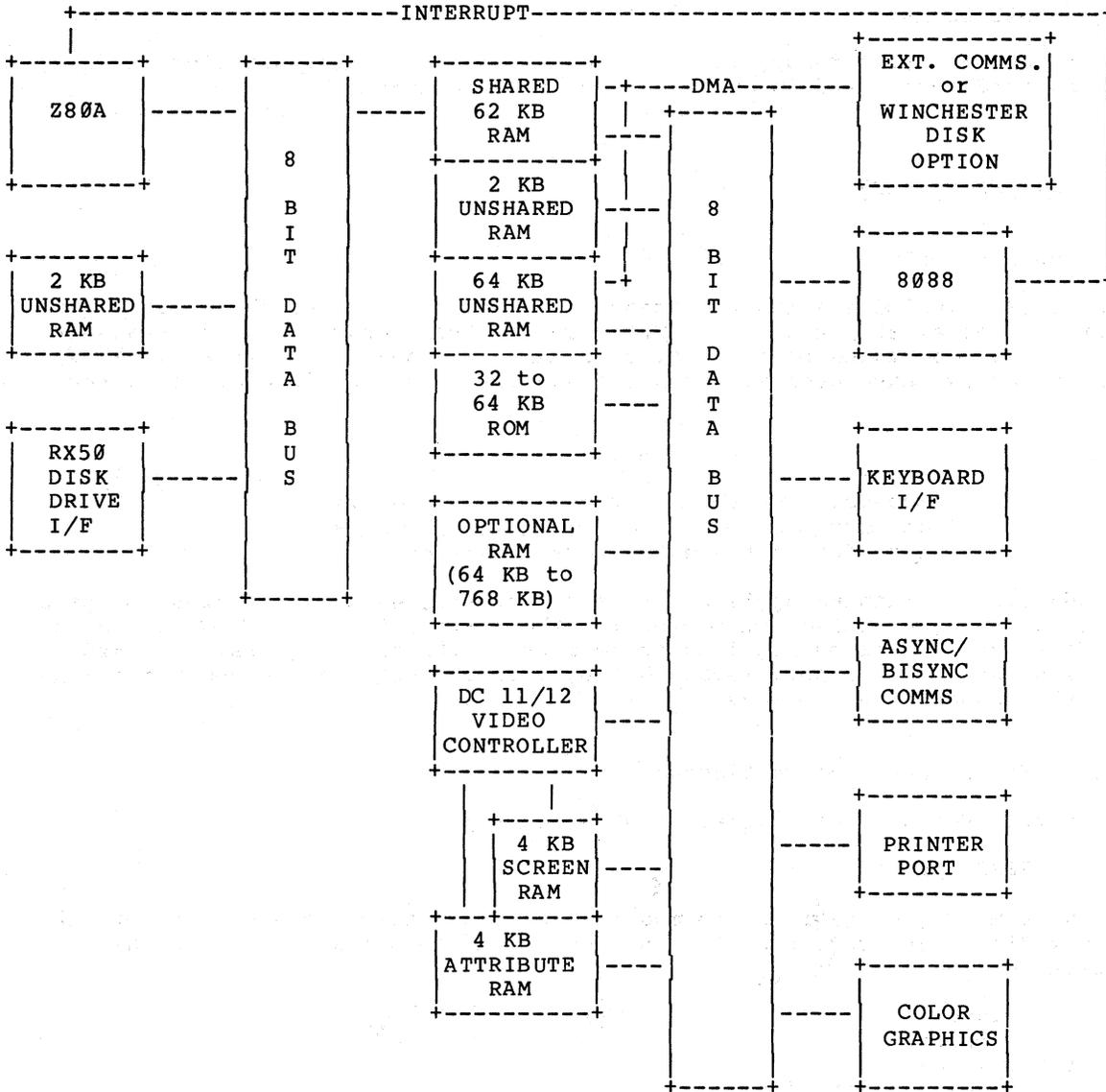
Figure 1. Mother Board Block Diagram
